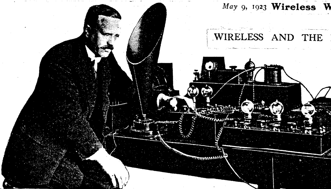
Extensive experiments have recently been carried out at Scotland Yard with a view to ascertaining whether wireless telephony would afford a quicker means of inter-communication between stations. The photograph shows the apparatus installed at Scotland Yard.
