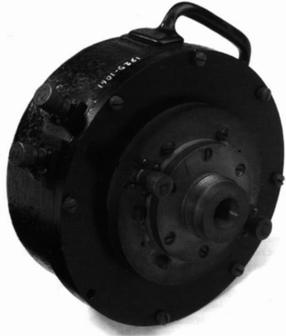
Fig 8: The Western Electric 555 W drive unit used with the loudspeaker horn.
