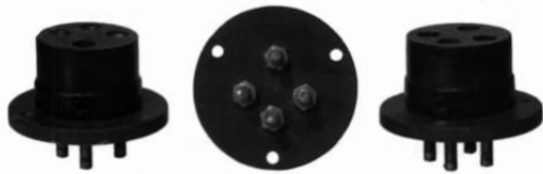
From left to right: valve holder, Valve holder also used for reactance unit, valve holder
