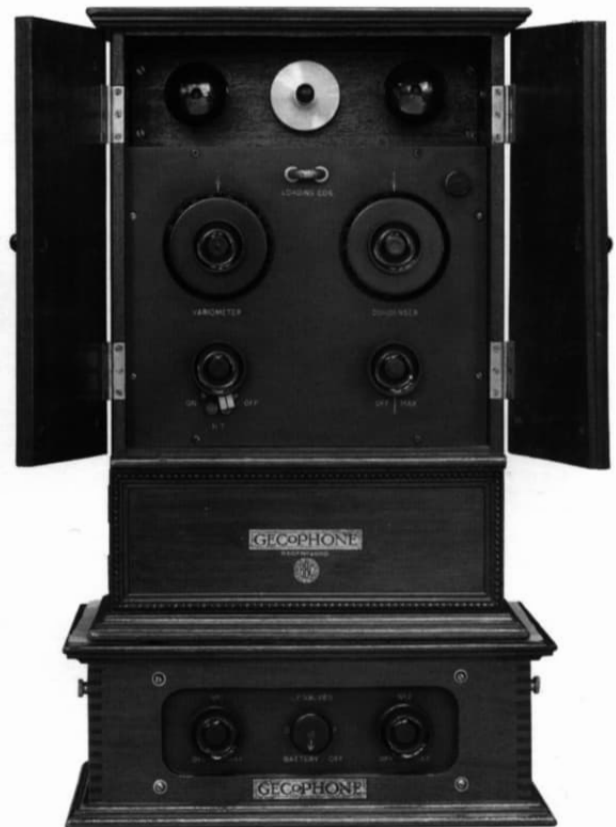
Ken Tythacott's set (has had a retro-fitted switch to isolate the LT supply in the top right hand corner of the control panel).
