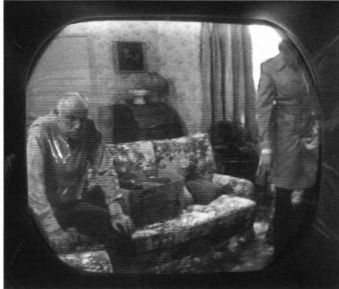
Close up of new re-gunned tube face showing bright crisp picture.
