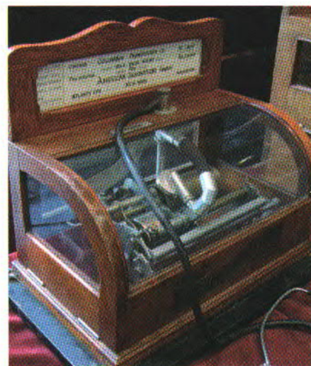
"Graphophone" a phonograph that uses a stethoscope
