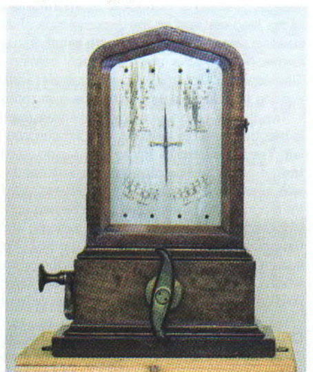
Single Needle Telegraph (UK c. 1845)
