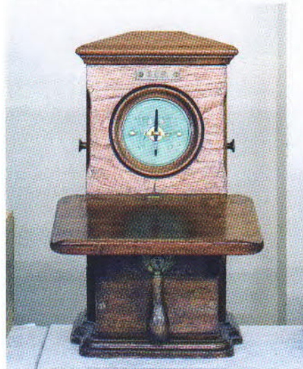
Single Needle Telegraph (UK c.1865)
