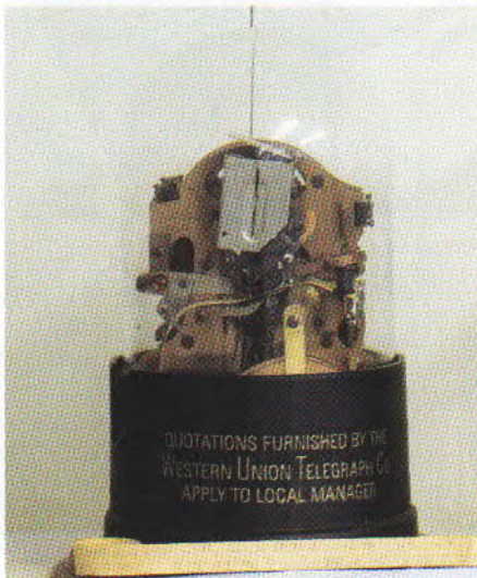
Self Winding Stock Ticker by Western Union (USA 1902)
