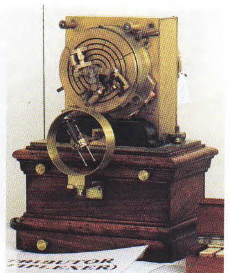
Multiplexer (Distributor) by Baudot (France c. 1880)
