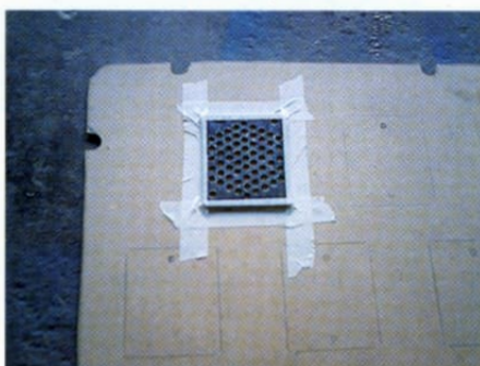
Blank roughed out and drilling guide attached using tape
