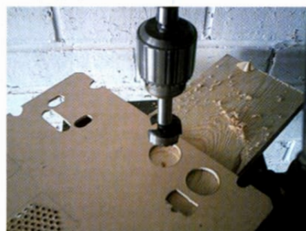
Big holes require big bits. 1" Forstner bit
