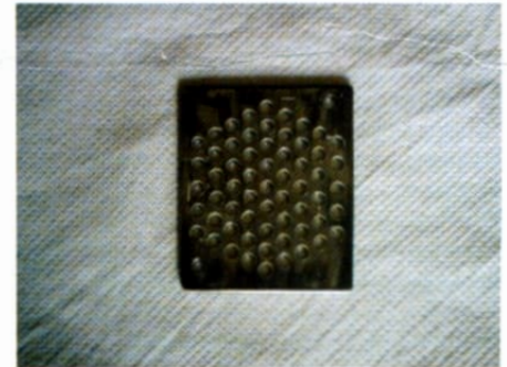
The drilling Guide, two additional corner holes were used for mounting on the Philco backs. Ten at a time!
