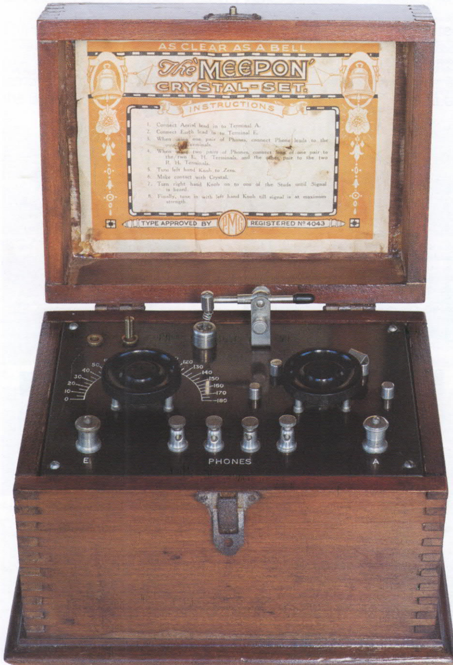
Above and opposite page: Later versions of the Meepon receiver were available with either an open or enclosed detector. These versions have a more ornate instruction label, and although there is no conventional BBC stamp, they feature an unusual "PMG" symbol on the instruction label. Although originally for broadcast band reception, many extant examples have been modified to allow for provision of a long-wave loading coil.
