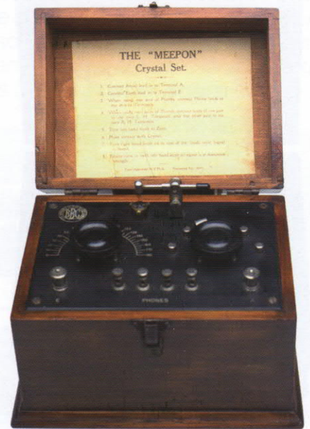
Early examples of the Meepon receiver, with plain instruction labels and the BBC stamp etched into the panel.
