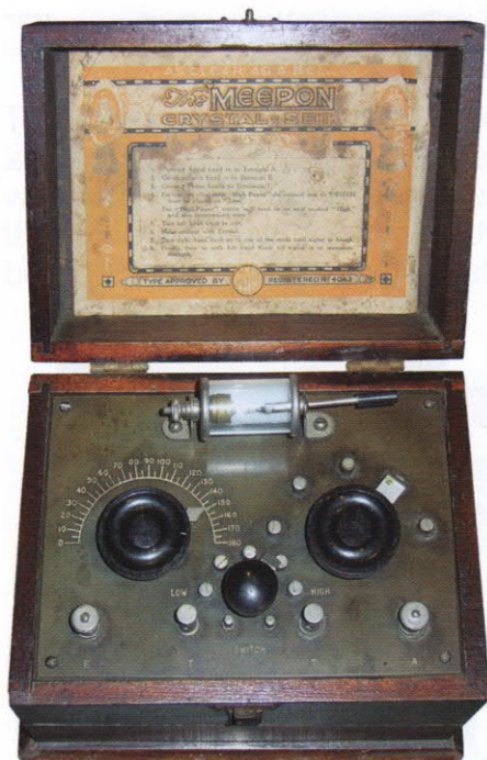
Above: The Meepon No.3 Super - a long-wave model with switch for reception of the high-power Chelmsford, 5XX station. Broadcast band could be tuned with switch in "low" position. Photograph courtesy Howard Stone.
