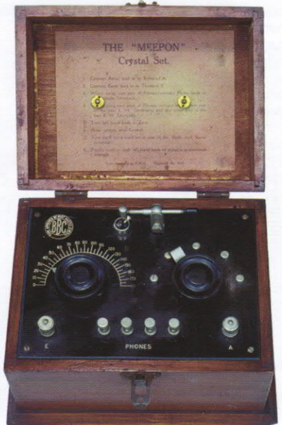
Above and opposite page: Later versions of the Meepon receiver were available with either an open or enclosed detector. These versions have a more ornate instruction label, and although there is no conventional BBC stamp, they feature an unusual "PMG" symbol on the instruction label. Although originally for broadcast band reception, many extant examples have been modified to allow for provision of a long-wave loading coil.
