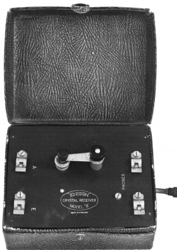
Ensign Model B with Perikon detector.
