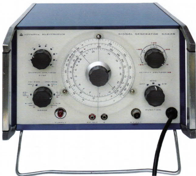
1: Advance SG62B signal generator
