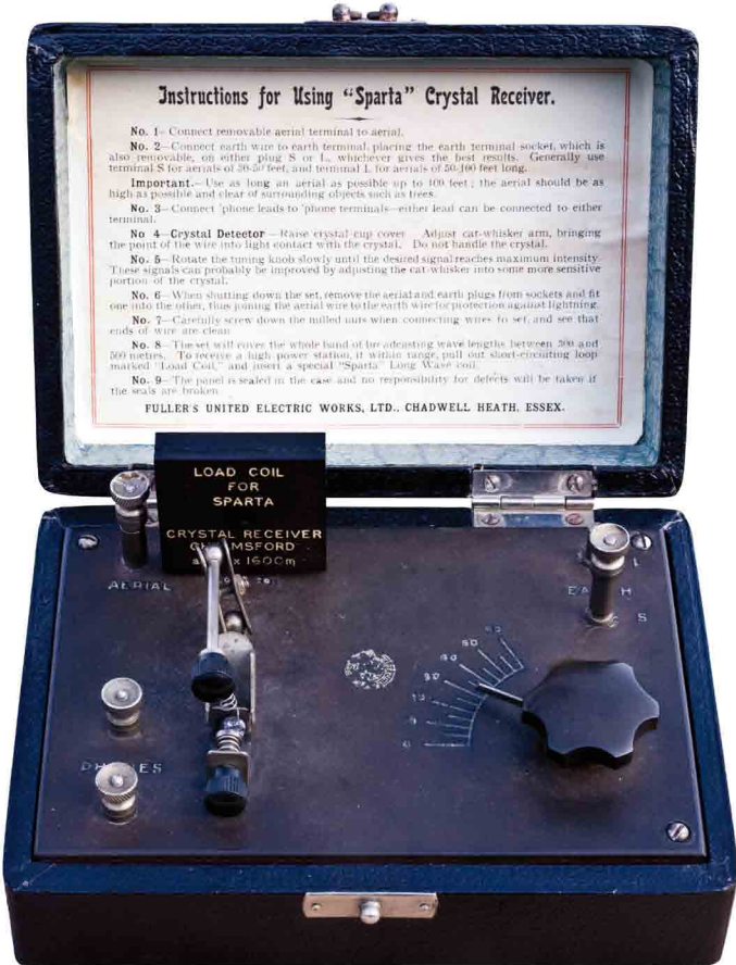
Above: Sparta crystal set of 1924 by Fullers United Electric Works Ltd., fitted with an early-style loading coil for reception of Chelmsford, 5XX.
