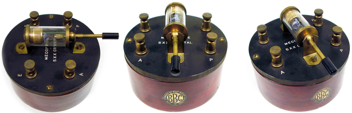
Measuring just 3½ inches in diameter, the 1924 circular Mecophone 5XX Crystal by Mann, Egerton & Co., Ltd. of Norwich was pre-tuned for reception of the BBC's long-wave station. The Post Office approval stamp indicates a manufacture date sometime before the end of the registration scheme in September 1924; in other words, shortly after the opening of Chelmsford, but almost a year before Daventry went on the air.
