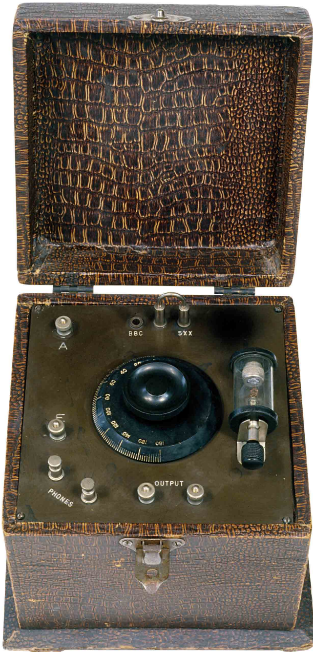
This unnamed set employed a shorting link to switch from "BBC" (the broadcast band) to 5XX.
