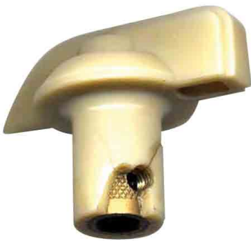
Broken wave-change knob
