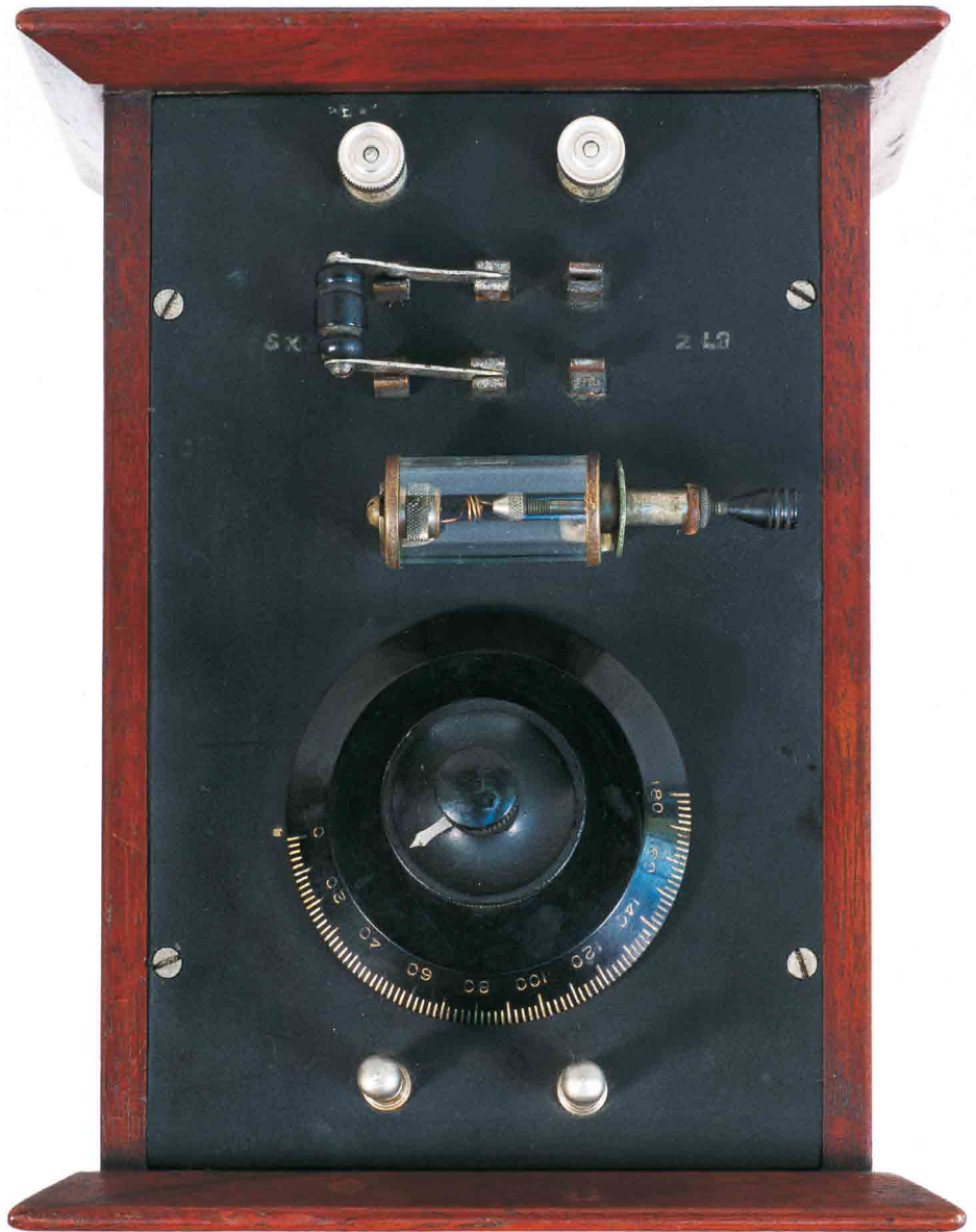
Above: Well-built amateur set with a double-pole panel switch for 2LO/5XX.
