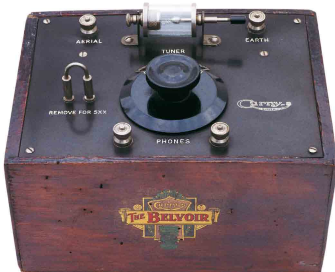
Currys produced their Belvoir model with a shorting link that could be removed for reception of 5XX.
