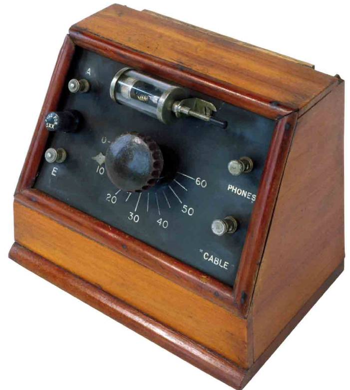
The Cable receiver by Cables and Electrical Supplies of London and the Rooco by J.R. Wireless, also of London, featured a pull-switch for reception of 5XX.
