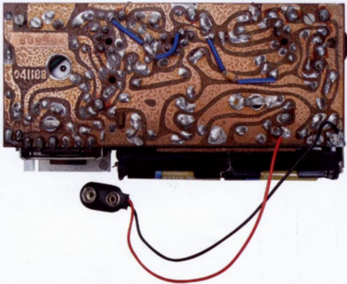
Fig 4: Alternative methods of using AAA cell holder on 6 volt radio, card circuit cover not shown
