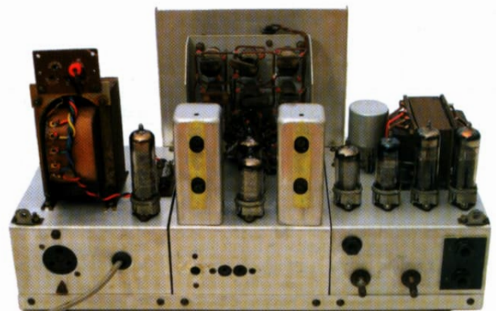
Centre right and right: The chassis of the SB4 showing the neat and modular layout of the set, a feature that would be retained on many of the later designs. The valve line up is typical of a period superhet with the B8A range of valves being employed these being EZ40, ECH42, EF41, EBC41, ECC40 and two EL41s. A 4 Watt output is claimed from the set. A gram socket is located on the rear along with the bass and treble controls.
