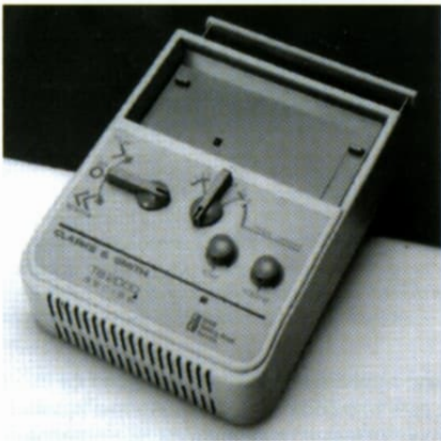
The later talking book cassette cartridge known as the "Tapete" was first introduced in 1965 with a 13 hour playing time using standard ¼ inch tape, and would remain the Clarke and Smith proprietary format for the talking book service until the demise of the firm in the late 1990s. Various versions were produced including a recordable unit for dictation purposes and language laboratory use.
