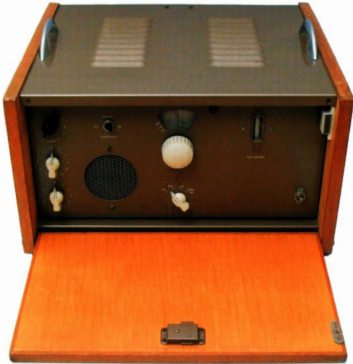
The later 88-20 AM/FM receiver amplifier. This example dates from the mid 1960s and followed the well established cabinet tradition with the drop down lockable flap. This example features EL84s in a parallel push pull arrangement and a semiconductor based FM tuner. Various versions of the 88 series were produced over the years, the second generation AM only equipment for example, and originally featured B8A valves throughout with parallel push pull EL41s and a neon tuning indicator. EM34s or EM84s will also be found as the tuning indicator in some models. The earliest of the 88 series FM models featured a valve based "bought in" tuner utilising an ECC85 which was prone to periodic drifting.
