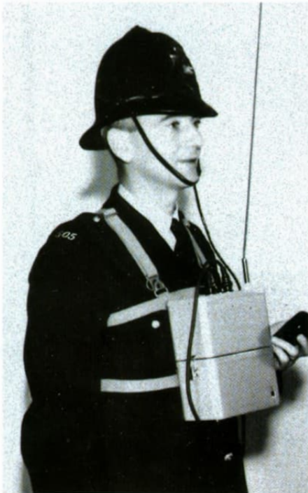
A marvel of post war miniaturisation, the Clarke and Smith design of portable two way radio supplied to the Metropolitan Police in the late 1940s. The battery supplies are located in the lower compartment.
