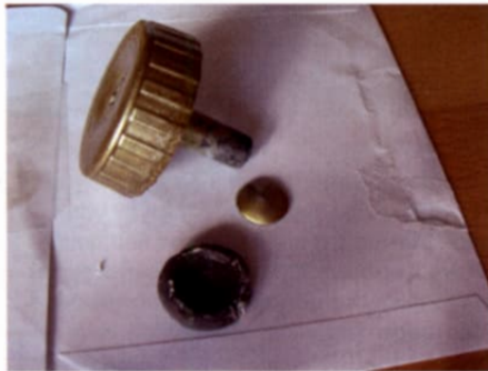
Sprayed knob, mould and finished brass cap
