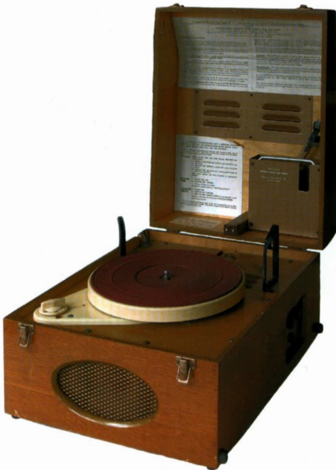
Above: The model 12 talking book gramophone first designed and produced by Clarke and Smith in 1950. The unit featured the novel method of housing the pickup in the lid, simplifying the replay process for the visually impaired. Initially the player was introduced with the original talking book standard of 24rpm. Later versions of the machine also accommodated the 16 rpm speed.
