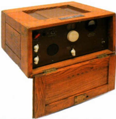
The 88-10 AM receiver amplifier dating from the very early 1950s and featuring the standard Mullard range of octal valves available at the time. This set has an abundance of EBC33s, three of which are strapped as triodes. As there appears to be no technical advantage it has to be assumed that these valves were obtained at such a low price that it worked out cheaper to produce like this. Provision is made for gram and for feeding into further amplifiers. The output pair are EL33s. Note the use of a moving coil meter to indicate signal strength. The set still has its previous owner's badge declaring it Equipment Number 4, Surrey County Council. The cabinet is made of solid oak. The similarly designed later series were manufactured from oak-faced ply.
