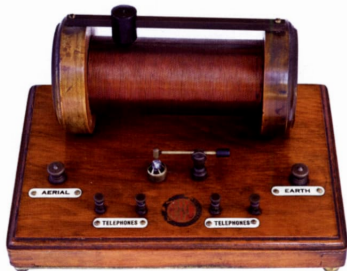
The slider-tuned Westraphone by Western Radio Company of Queen Street, Cardiff was a simple receiver built on an open mahogany plinth. The set at top (shown here with a replacement permanent detector) carries the Post-Office registration number 863 and features the manufacturer's transfer on the coil. The version at bottom, with an original cat's-whisker/galena detector and terminals for two pairs of headphones, has the registration number 4182 inscribed under the base. Top photograph courtesy of David Jones.
