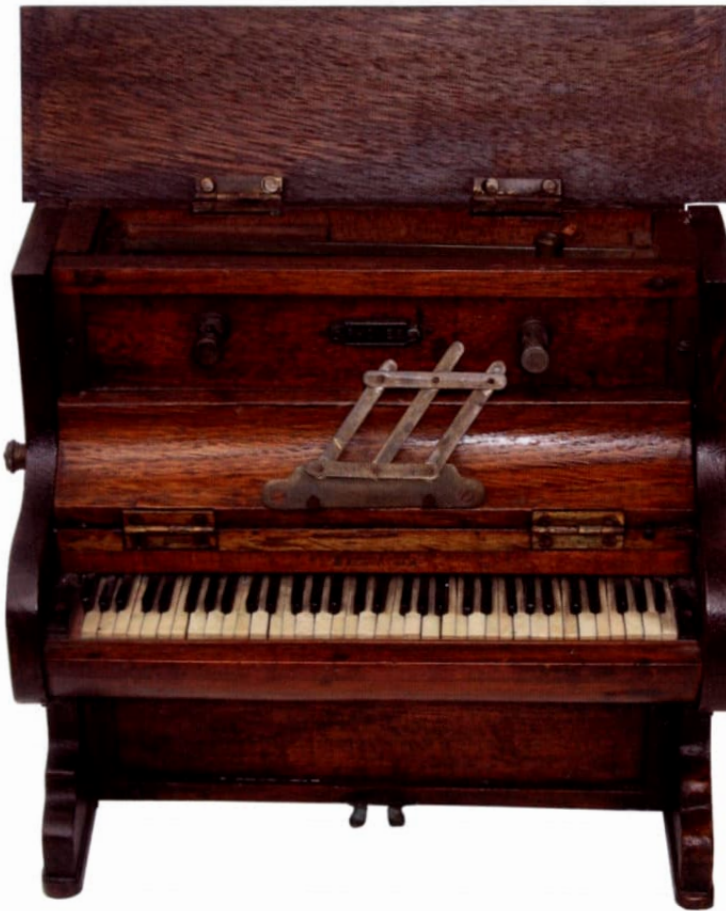
This circa 1924 "piano-style" crystal set was built by a Mr. Edwards (see close-up at top left) living near Ruthin, North Wales. Ruthin is about 45 miles from Manchester (2ZY) and about 25 miles from Liverpool (6LV), so it might just have been possible to listen-in on a crystal set if conditions were favourable. Photographs courtesy of David Jones.
