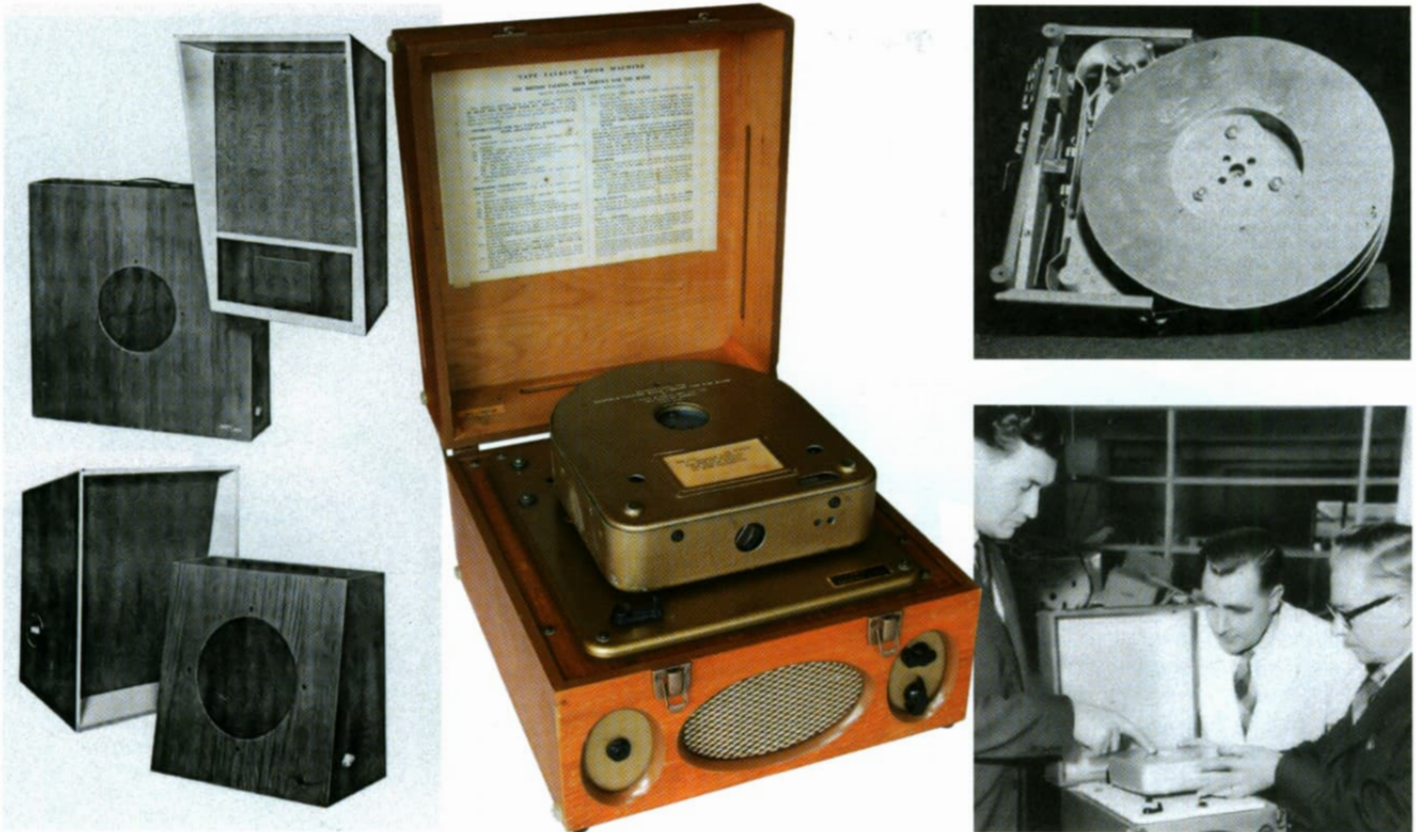
Far left: A small selection from the range of loudspeaker enclosures available to schools and various institutions during the 1950s and 1960s. Centre: MK1 Talking Book: The first magnetic tape based talking book produced for the RNIB from around 1960. The development period appears to have spanned nearly ten years. Top right: The fairly complex internal mechanism of the talking book magazine, using a stacked spool arrangement and 1/2 inch magnetic tape. Far right: Major Clarke, Freddie Bellis and Alec Smith seen here examining the MK1 talking book player by this time in production form.
