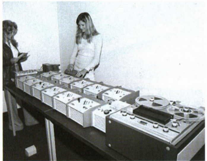
Above: How the duplication process was handled in Australia during the 1970s. A Ferrograph Series seven recorder provides the master source with an intermediate controller and recordable Tapete machines. This operation required a fair amount of manual dexterity on the part of the operators overseeing the process. Each machine had to be loaded manually although some of the remaining process does appear to be semi automatic. It is thought that the tape was duplicated across in real time.
