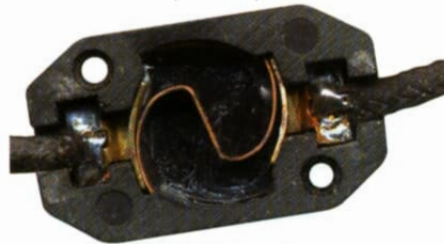
Inside the mains switch
