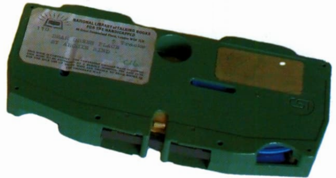
The later talking book cassette cartridge known as the "Tapete" was first introduced in 1965 with a 13 hour playing time using standard ¼ inch tape, and would remain the Clarke and Smith proprietary format for the talking book service until the demise of the firm in the late 1990s. Various versions were produced including a recordable unit for dictation purposes and language laboratory use.
