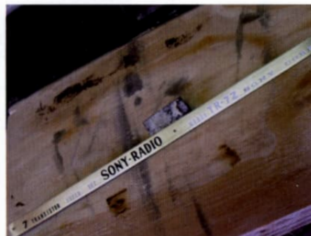
Wet & Dry removes the lacquer, leaves the lettering
