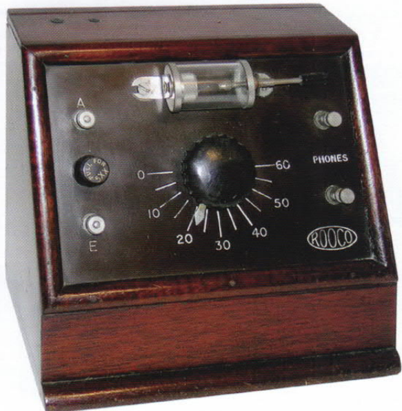
Above and below: Another example of a J.R. Wireless Company (ROOCO) and a Cables & Electrical Supplies Company (CABLE) receiver sharing a common design. So the connection between the two firm's products extended to receivers beyond the 5304 sets.
