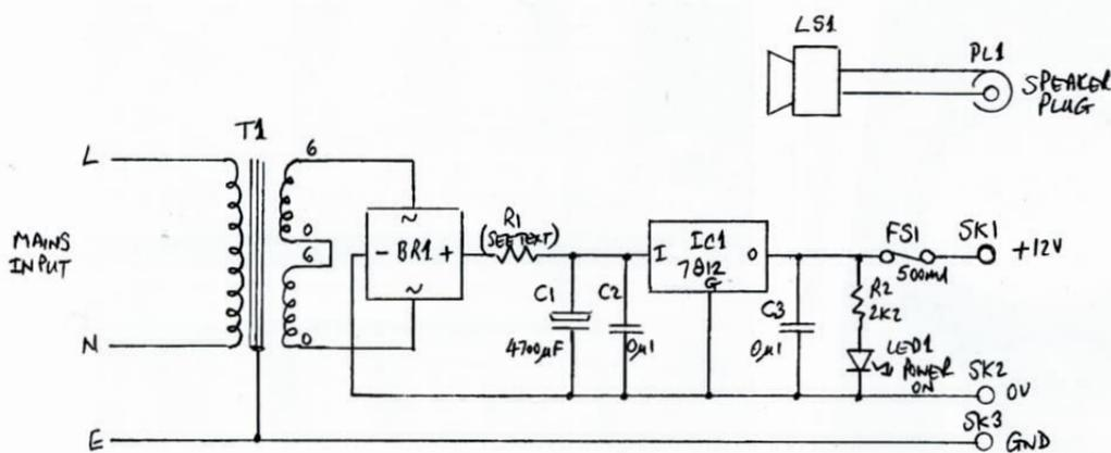
Figure 1. SCHEMATIC OF THE SAILOR 66T POWER SUPPLY & SPEAKER UNIT
