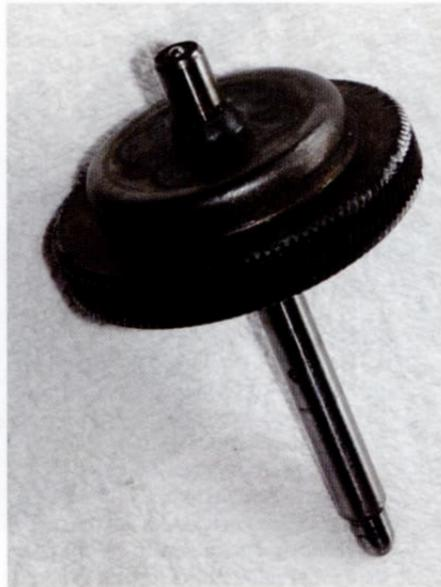
2: Fibre gear wheel
