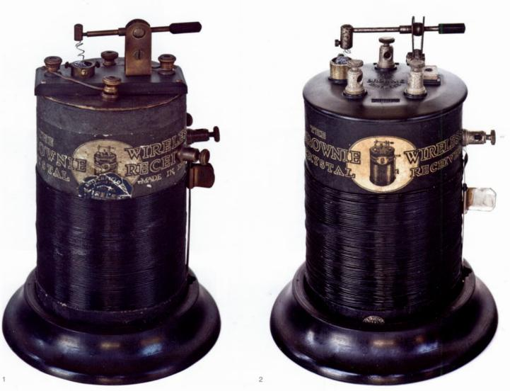
The original Brownie crystal set of 1923 (1) was sold as a kit with a discrete detector assembly mounted on a cardboard panel. Later sets featured an ebonite panel with
