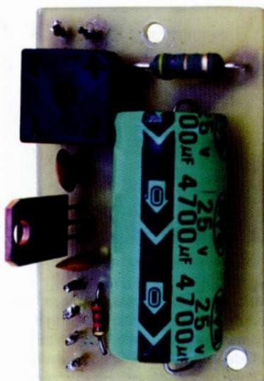
The assembled power supply board
