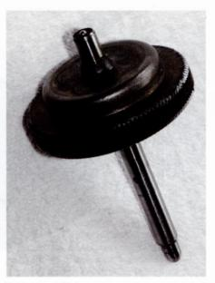
2: Fibre gear wheel
