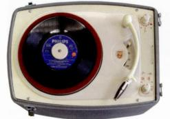
Fig 15. AG9104 Gramophone 1955. First battery turntable with a transistor amplifier.
