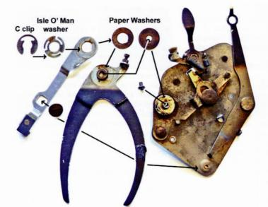
12: Brake mechanism stripped
