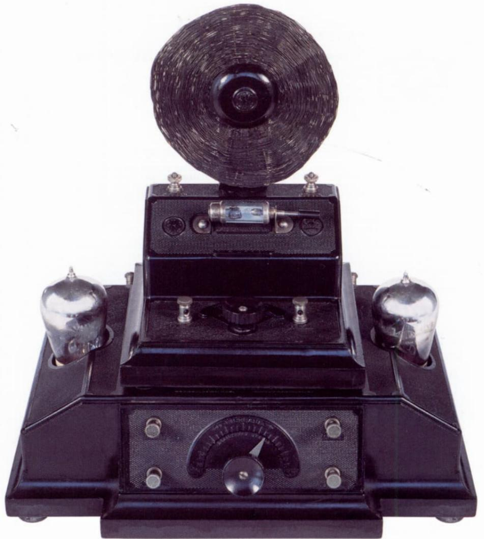
Two-valve note magnifier unit designed to accommodate the Brownie No.1 crystal receiver.
