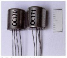
Fig 10. Germanium "pushed out base transistor. Types OC170, OC171. Suitable for high frequencies. c. 1958
