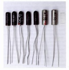
Fig 16. The amplifier in the AG9104 gramophone with 1xOC71, 2xOC72 transistors
