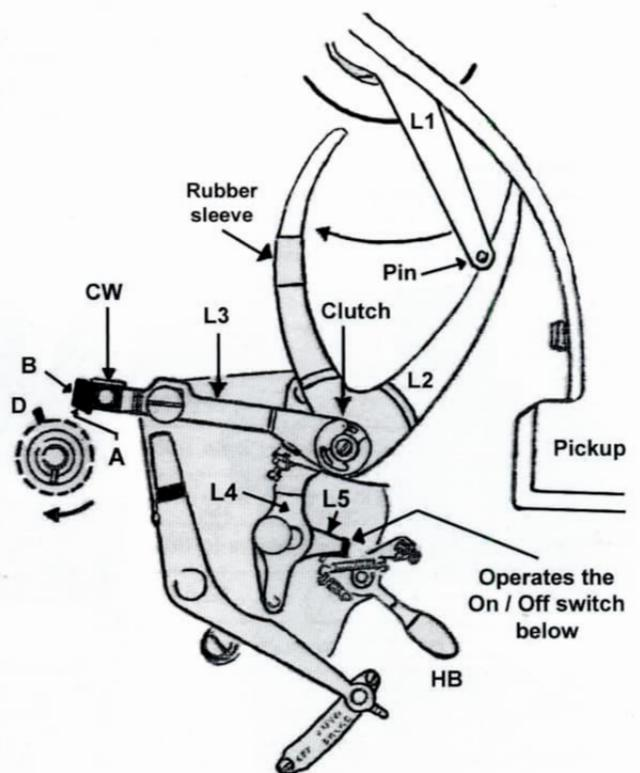
Fig 2: Brake mechanism from HMV service data
