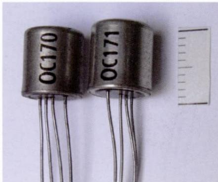
Fig 10. Germanium "pushed out base" transistor. Types OC170, OC171. Suitable for high frequencies. c. 1958
