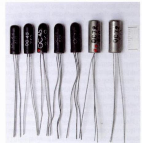
Fig 18. Transistor line up for the L3X71T radio: 1xOC44 2xOC45 2xOC71 2xOC72
