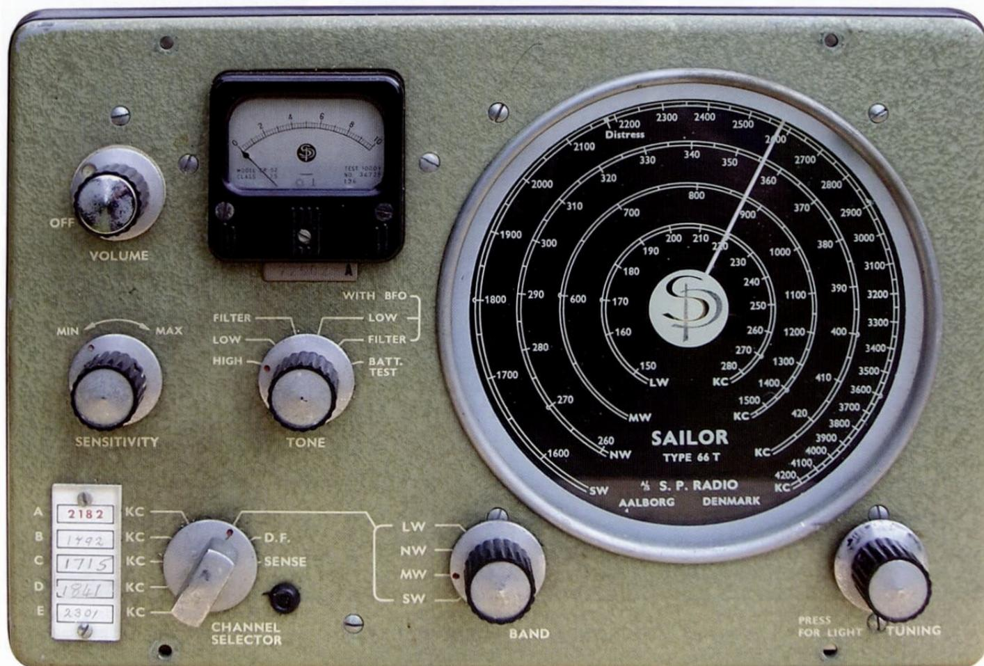
The receiver allows for five crystal-controlled frequencies, selectable from the front panel. My receiver was equipped with 2652kHz, 2262kHz, 2185kHz, 2311kHz and 2771kHz crystals, giving reception frequencies of 2182kHz, 1792kHz, 1715kHz, 1841kHz and 2301kHz respectively. With an associated transmitter, no doubt the boats these receivers were fitted to contributed to the "fish phone" annoyances in the 160m band.
