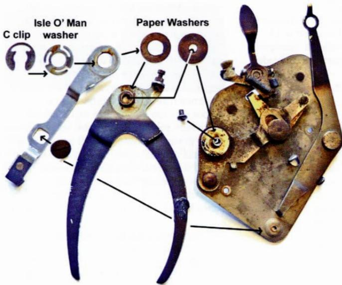
12: Brake mechanism stripped
