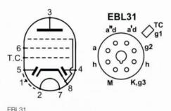
Double Diode output valve and base connections
