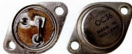
Fig 13. Germanium high power transistor type OC36. In the standard TO-3 case. c. 1959
