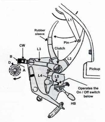
Fig 2: Brake mechanism from HMV service data
