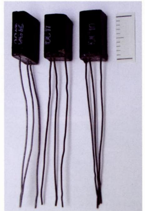
Fig 6 The first commercial Philips Ge junction transistors OC10/11/12. The housing is plastic. c. 1953-54
