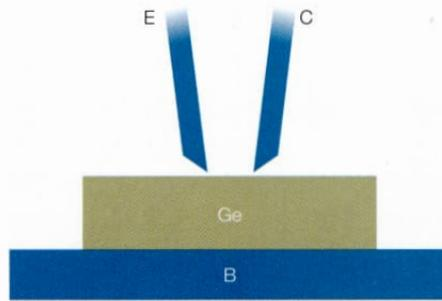
Fig 5 Point Contact Transistor. Ge Germanium Crystal. E emitter. C collector. B base. Thin wires of phosphor bronze or tungsten form contacts with the germanium. A current pulse melted and re-crystallized the germanium, forming the p-n junction.
