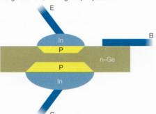
Fig 7 Germanium junction transistor made by alloying. Each p-n junction was made from melting a dot of indium on the germanium which gave p-type on cooling and recrystallising. The problem with this pnp junction transistor was poor control of the distance between the two p-regions (base thickness).
