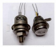
Fig 12. Germanium high power transistor type OC16. The first commercial power transistor in Europe. c. 1956
