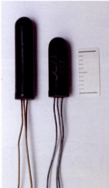
Fig 8 Germanium Junction Transistor. Types of OC70, OC72 in glass encapsulation. Later, c. 1954, the OC72 had metal encapsulation.
