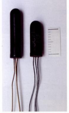
Fig 8 Germanium Junction Transistor. Types of OC70, OC72 in glass encapsulation. Later, c. 1954, the OC72 had metal encapsulation.
