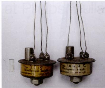
Fig 11. Germanium high power transistor. Prototypes OC15, 100 OC c. 1955
