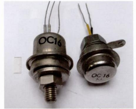
Fig 12. Germanium high power transistor type OC16. The first commercial power transistor in Europe. c. 1956
