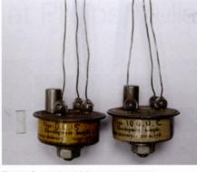
Fig 11. Germanium high power transistor. Prototypes OC15, 100 OC c. 1955
