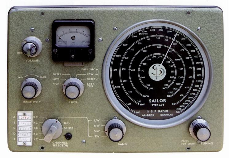
The receiver allows for five crystal-controlled frequencies, selectable from the front panel. My receiver was equipped with 2652kHz, 2262kHz, 2185kHz, 2311kHz and 2771kHz crystals, giving reception frequencies of 2182kHz, 1792kHz, 1715kHz, 1841kHz and 2301kHz respectively. With an associated transmitter, no doubt the boats these receivers were fitted to contributed to the "fish phone" annoyances in the 160m band.
