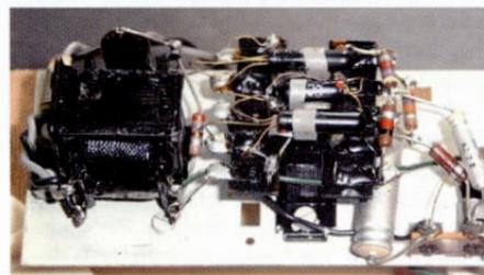
Fig 16. The amplifier in the AG9104 gramophone with 1xOC71, 2xOC72 transistors
