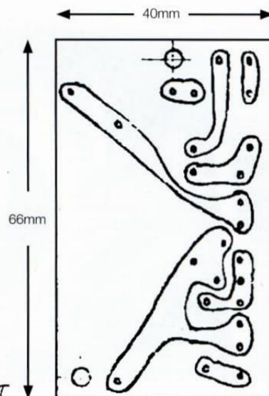
Figure 2a: PCB tracking
