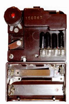
Fig 14. Philips first transistor hearing aid. Type KL5400, c. 1954
