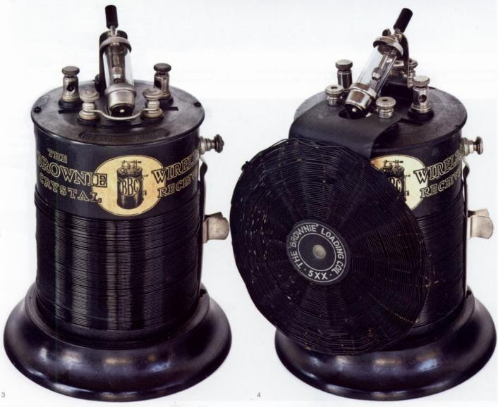
either an open (2) or glass-enclosed detector (3). A loading coil was available for side mounting for reception of Chelmsford, 5XX on long-wave. (4).
