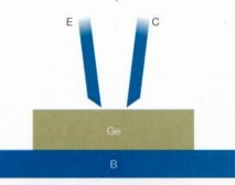
Fig 5 Point Contact Transistor. Ge Germanium Crystal. E emitter. C collector. B base. Thin wires of phosphor bronze or tungsten form contacts with the germanium. A current pulse melted and re-crystallized the germanium, forming the p-n junction.
