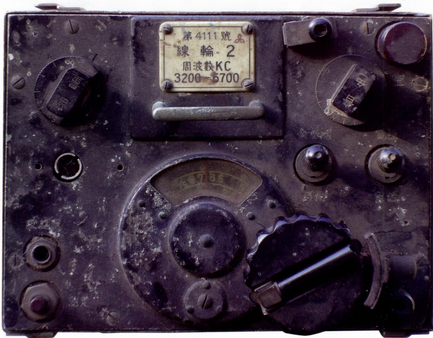
An early reference<sup>1</sup> gives the valves as being 'identical' with the American 6P7. It also records a frequency coverage, using two plug-in coils, of 1.5 to 6.7 mHz, the IF being 450 kHz. A later Article<sup>2</sup> gives more illustrations. Both articles give good general details. Howard's radio has a No.2 coil pack, 3.2 to 6.7 mHz. He thought he had the other in his garage but I have never found it.
