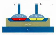
1958. This made it finally possible to produce high-frequency transistors (above 100 MHz).
