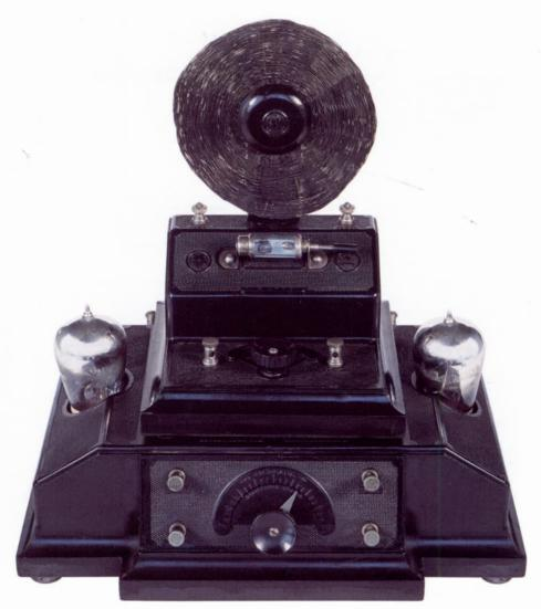
Two-valve note magnifier unit designed to accomodate the Brownie No.1 crystal receiver.
