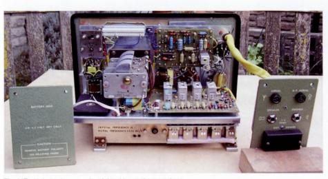
The 66T with its back removed and the side panels opened out
