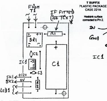
The assembled power supply board
