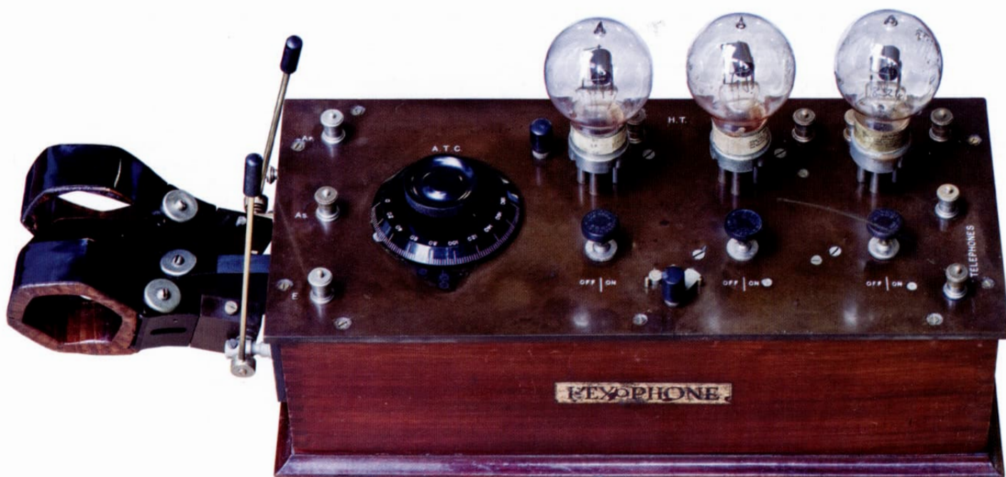
Rexophone three-valve receiver. (Frame aerial holder is not present on this example.)
