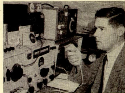
An Amateur station assembled with aerial tuner, wavemeter, receiver, transmitter, and other equipment for receiving and transmitting on the amateur bands.
