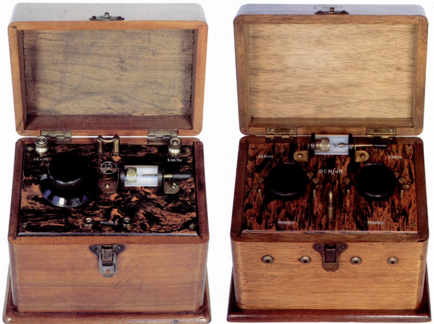
Above: Sloping panel, variometer-tuned design. No model name, other than the company's trademark, but – other than the closed cabinet design – consistent with the V-Type listed in the 1926 Wireless World Buyer's Guide . Headphone connection was by means of patented Rigaut sockets. Socket for long-wave loading coil with "folded" shorting link to permit lid closure. Year of manufacture was probably 1924.
