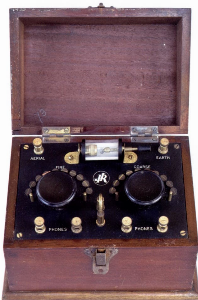
Above: Jean Rigaut model S Type. Tuning was by a linear slide coil contact operated by an arm projecting through the plinth. Socket for long-wave loading coil.
