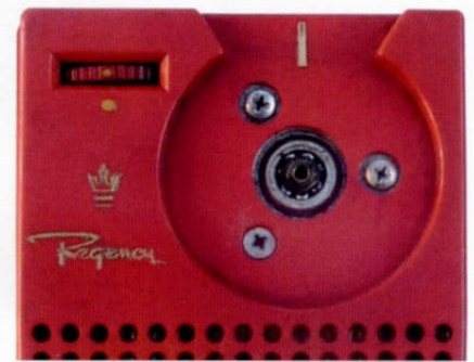
Tuning knob removed revealing screws
