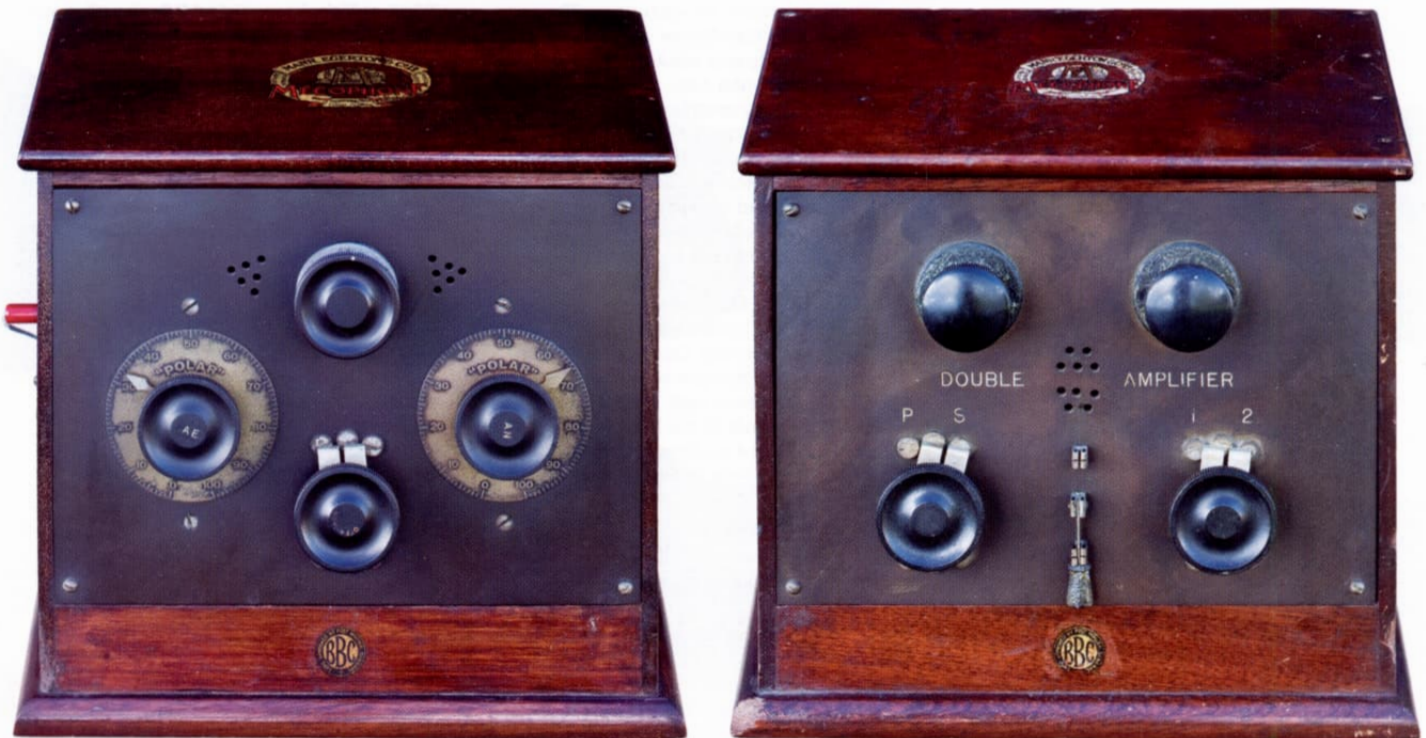
The Mecophone one-valve receiver used Mann, Egerton's patented circuit intended for improved volume and stability. The station list in the receiver's lid provides the wavelengths of the original eight BBC Main Stations. Bournemouth, 6BM was the last of these to open, on October 17th, 1923, so the model was likely introduced close to this date. The company produced a matching two-valve note magnifier.
