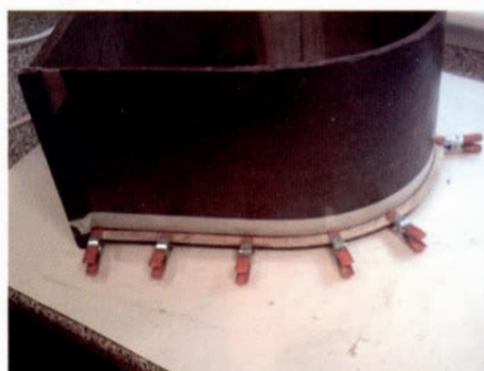
Replacement strips glued in place
