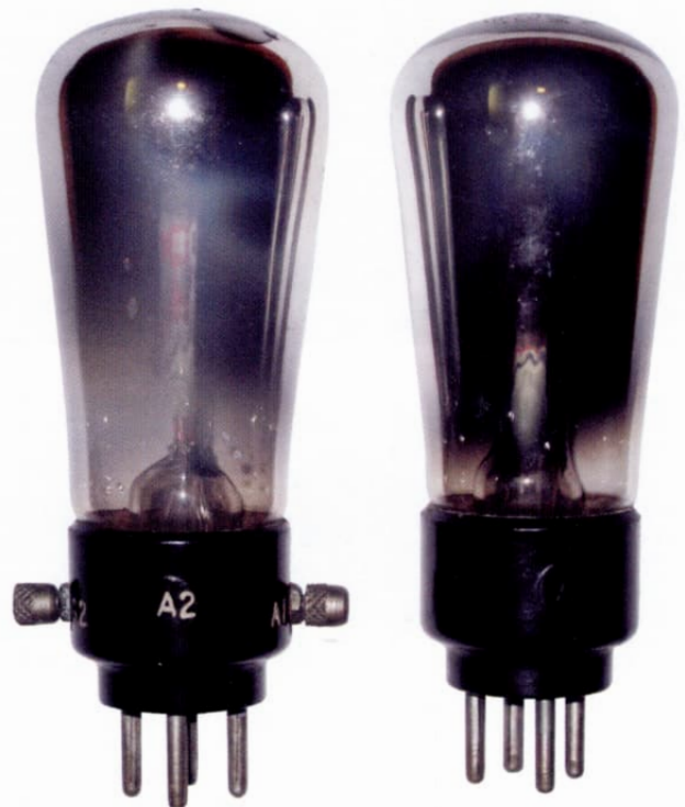
Above: The original TS215 and P227 (both O/C) as found in the radio.
