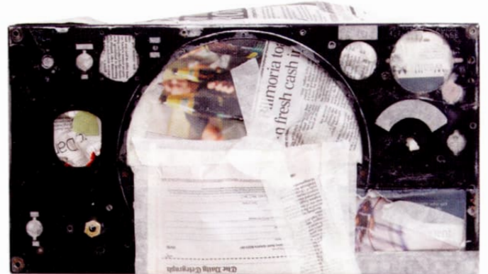
The front panel ready for re-spray
