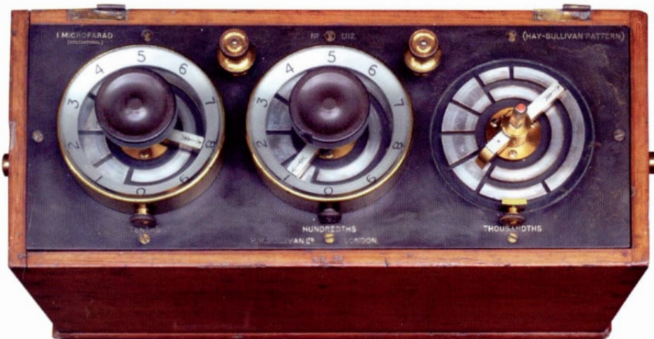
25: Decade Mica Condenser, 0.001-1uF (post-1922)
