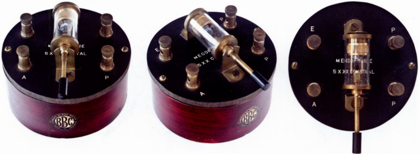
Above: The Mecophone 5XX receiver was tuned for reception of 1,600 metres, long-wave only.
