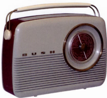
The MB60 (Early) model using the A99 chassis
