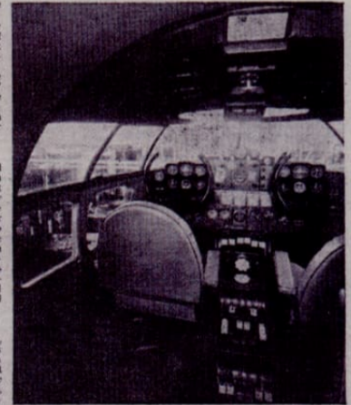
View of the interior of the pilot's compartment of a Curtiss-Wright aircraft (Model 20), showing arrangement of instruments, a type control wheel and the tail-rod instrument panel.
