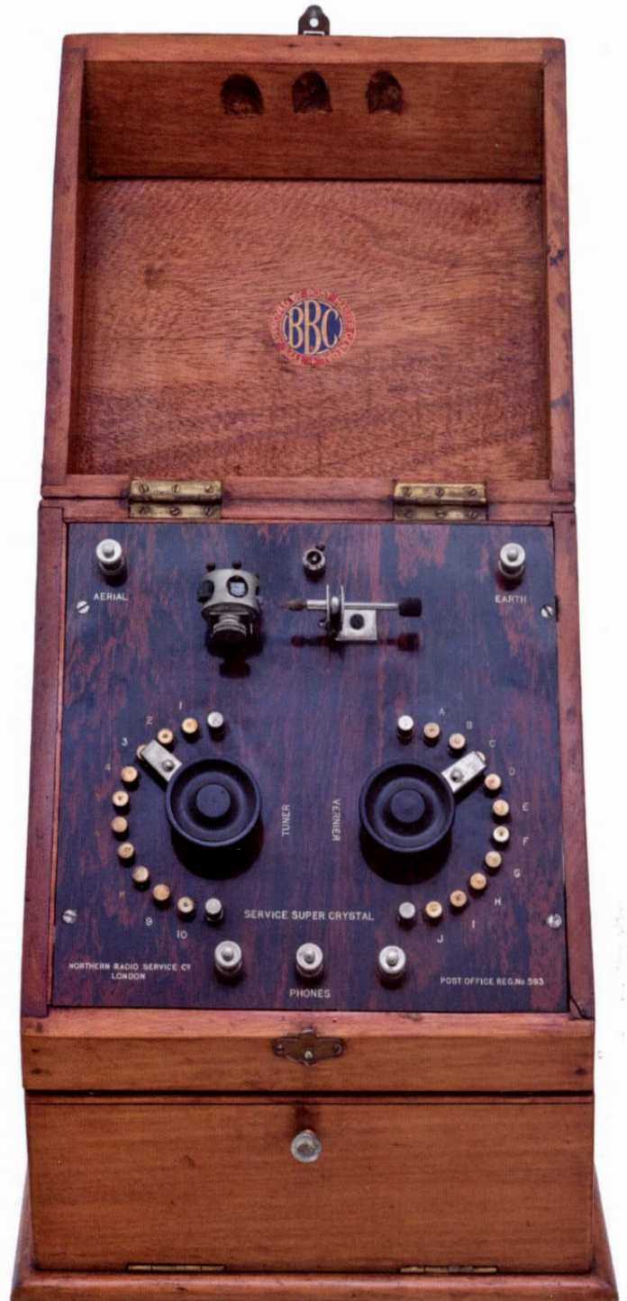
Above: 'SERVICE SUPER CRYSTAL' receiver by Service Radio Company Limited featuring the Service Multi-Crystal Detector and Multiphone headphone adaptor Above, Right: 'SERVICE SUPER CRYSTAL' receiver by Northern Radio Service Company Limited also featuring the Service Multi-Crystal Detector
