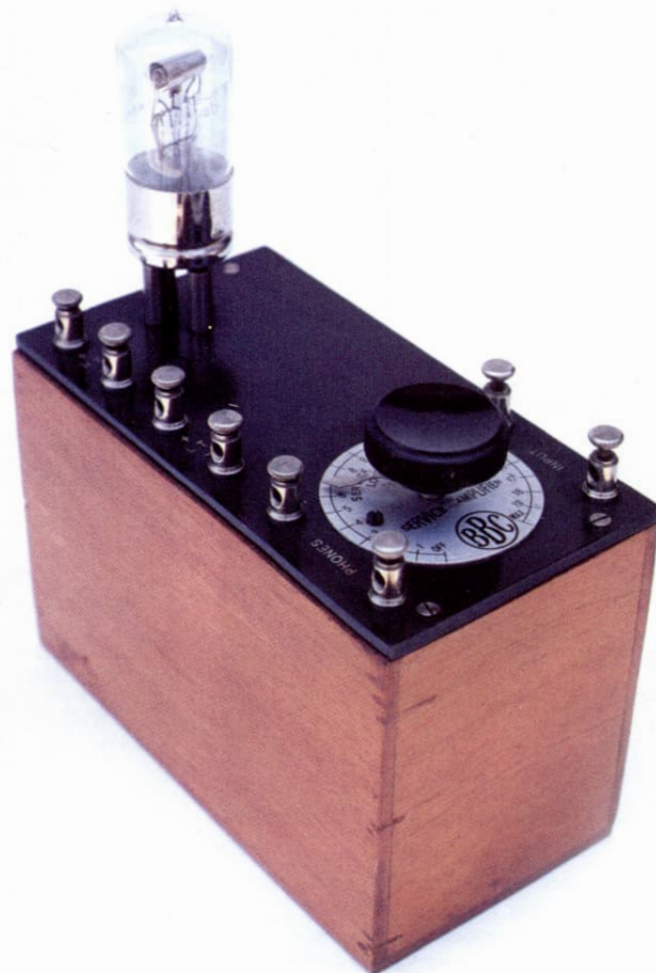
Left: Service Radio Company's Service Crystal model with one-valve amplifier fitted into the headphone compartment.
