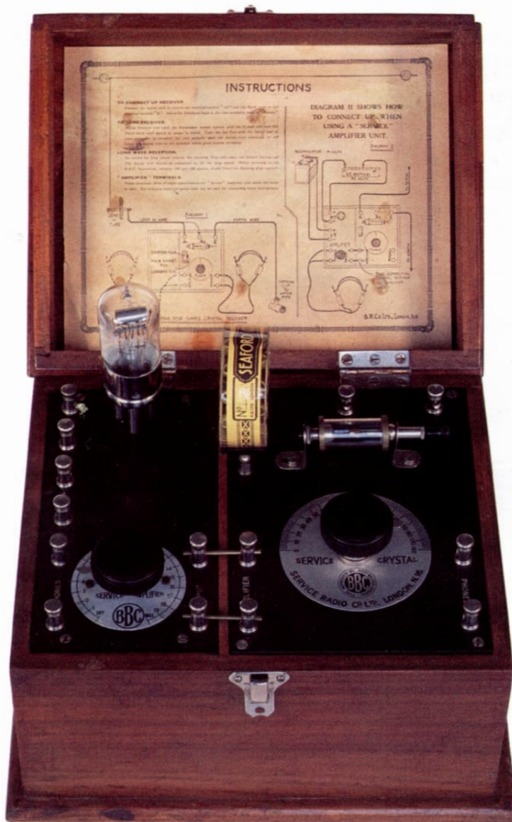
Left: Service Radio Company's Service Crystal model with one-valve amplifier fitted into the headphone compartment.
