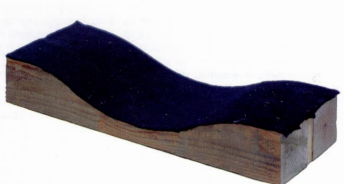
Below: Former to help veneer keep shape on curved top of Philips set
