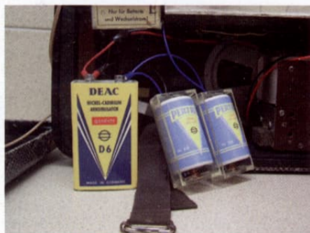
DEAC ni-cad and Pertrix No.231 cells
