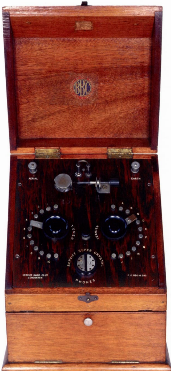
Above: 'SERVICE SUPER CRYSTAL' receiver by Service Radio Company Limited featuring the Service Multi-Crystal Detector and Multiphone headphone adaptor Above, Right: 'SERVICE SUPER CRYSTAL' receiver by Northern Radio Service Company Limited also featuring the Service Multi-Crystal Detector
