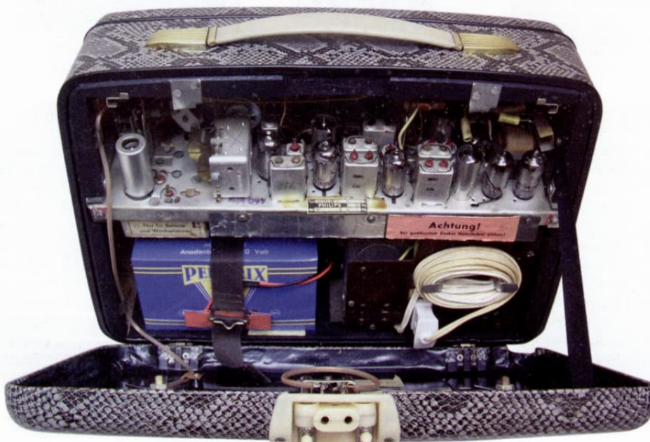
DEAC ni-cad and Pertrix No.231 cells
