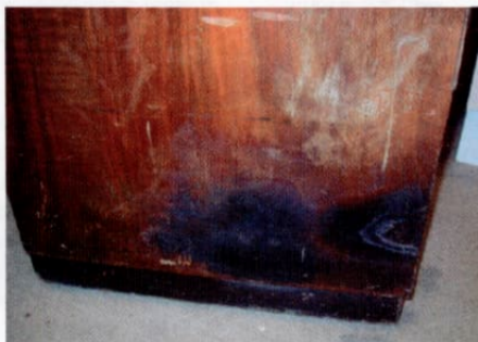
Burns on the cabinet
