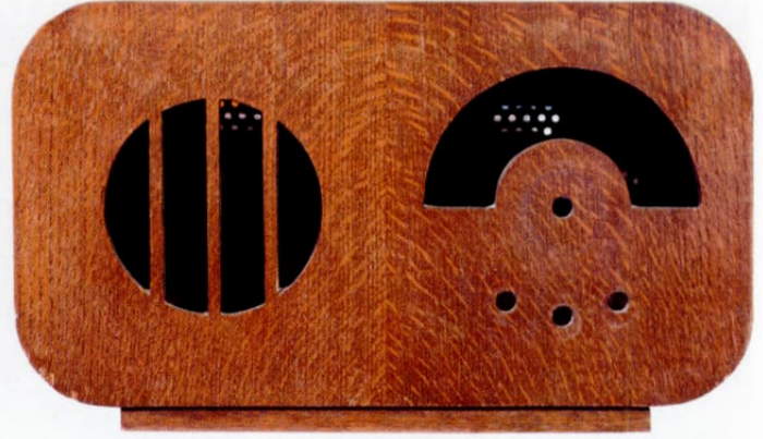
Prototype cabinet for testing fit of Ekco AC85 chassis.
