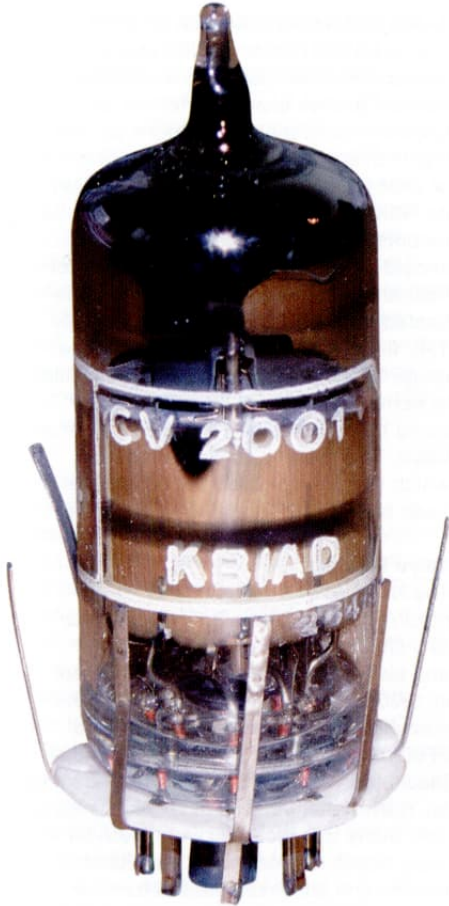
Figure 11: Photo of the CV2001 valve, or more accurately this seems to be the code for the valve-plus-socket assembly.
