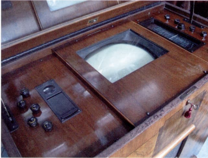
Viewers view - control panel. Note blanking plug over redundant system switch
