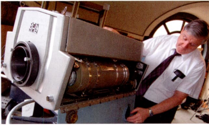
TK 42 colour camera. 3 Vidicon and 1 Image Orthicon tube combined. Not a happy mix.
