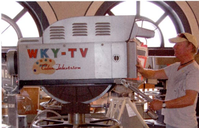
Dicky manhandles a TK41C. This camera type was capable of producing under the right conditions, very pleasant colour pictures.
