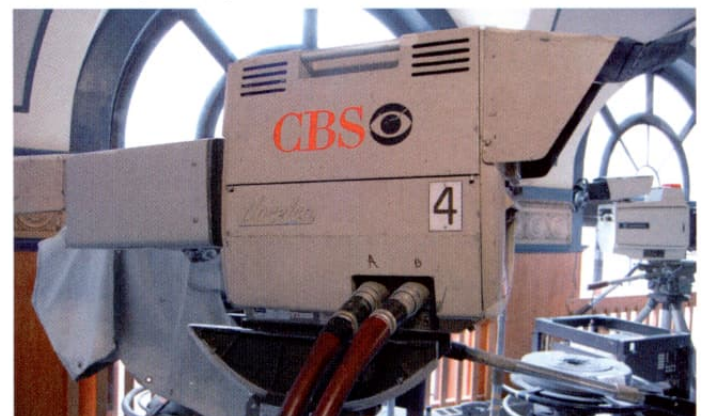
A PC 60 ex-CBS News. Note the camera's grab handle is tubular. Later models had one piece body panel oblongs. The things you learn.....
