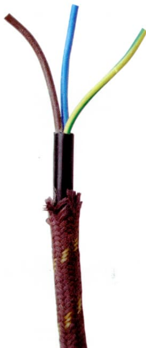
The new mains lead inside the original braid
