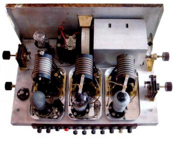
RF stages, and one at the detector. Care was taken not to let them escape! Each of the three coil assemblies was then dismantled. This gave access to the three sets of switch contact pairs for the wave-change mechanism. Crocus paper and a switch cleaner restored the contacts to reliable operation.
