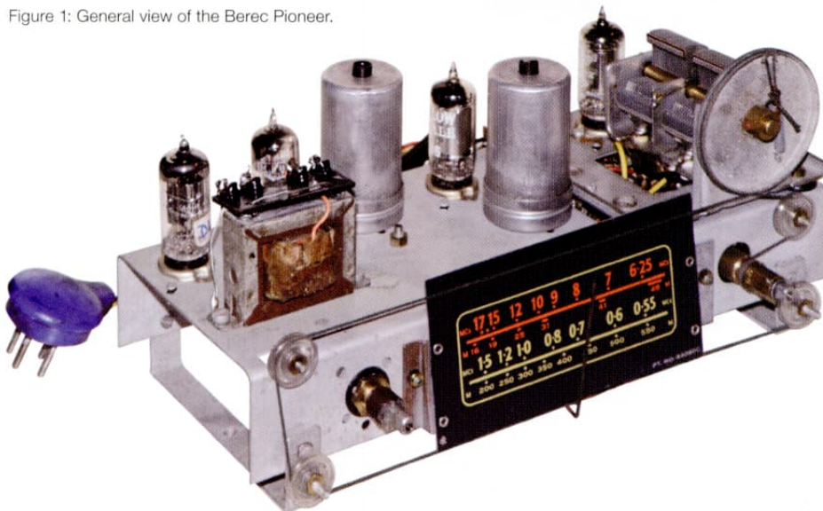
Figure 2: Front view of the Pioneer's chassis removed from the case. This is 'as removed', with no dusting, and its clean condition can be seen. The battery plug can be seen 'lurking' round the back.
