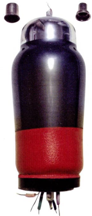
Fig 6: EBL1 large top cap removed, correct EBL31 cap ready
