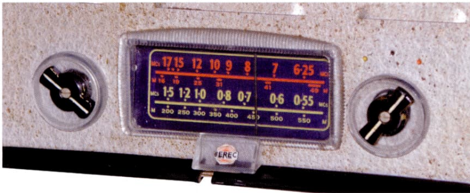
Figure 3: The controls and tuning dial of the Pioneer with a 'BEREC' sticker mounted under the dial. The combined wave change / on-off switch is on the right, inside the tuning knob, and the volume control is on the left. The background colour to the dial is the classic Ever Ready blue.
