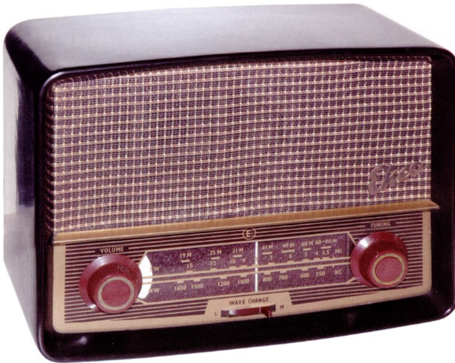
Figure 9: The Ekco U241 table radio, after the cabinet had been cleaned and polished. The white band by the volume control indicates that the set is switched on. There are no dial lights.
