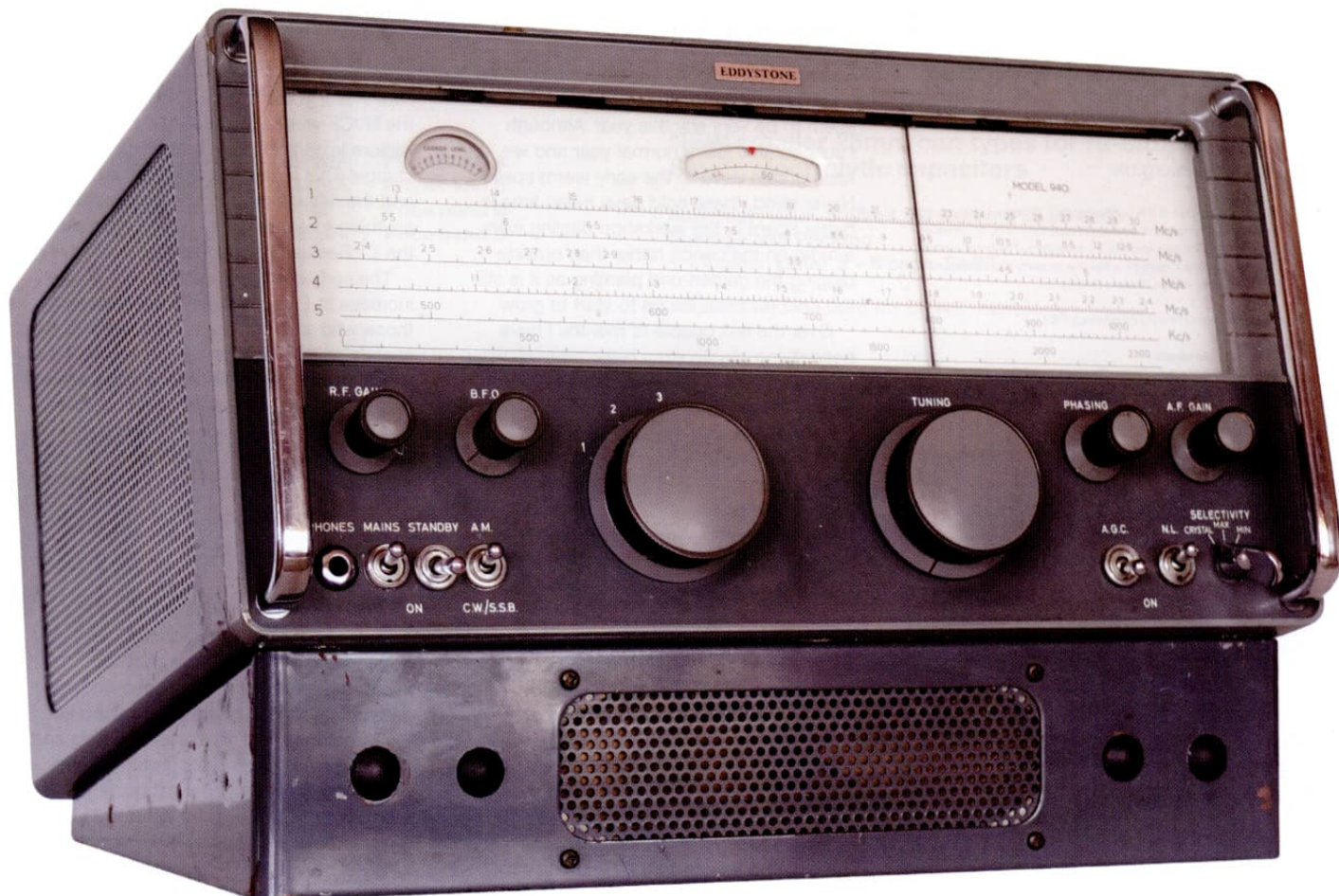
The Eddystone S940. The large knobs are for tuning and wave changing. At over 14 inches wide, the tuning dial provides plenty of room for well spaced and legible calibrations. At the centre top of the dial is a window showing the edge of the 6 inch diameter vernier disc. To the left is the meter indicating the strength of the received signals.
