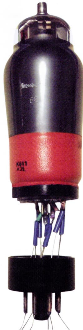
Fig 5: EBL1 conversion to EBL31 ready for base to be soldered
