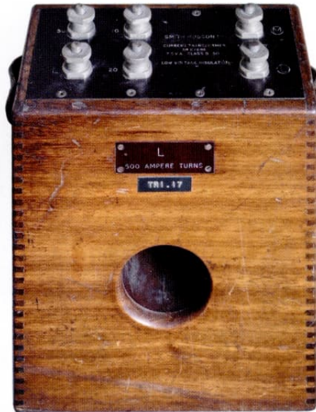
Fig 16: Current Transformers (a) Smith Hobson Ltd.
