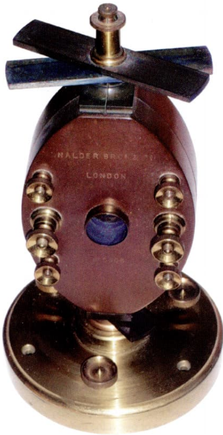
Fig 4a: Astatic Tangent Galvanometer (Nalder Bros)
