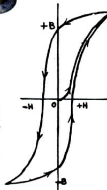
Fig 7 (above): Kelvin Current Balance (Glasgow University) Fig 8 (left): B-H magnetisation curve
