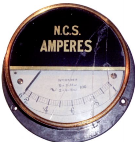
Fig 14a: NCS Gravity Ammeter (repulsion)
