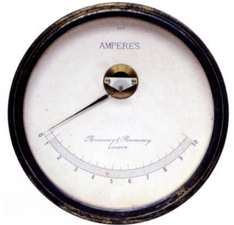
Fig 13a: Rumney & Rumney Ammeter (repulsion)
