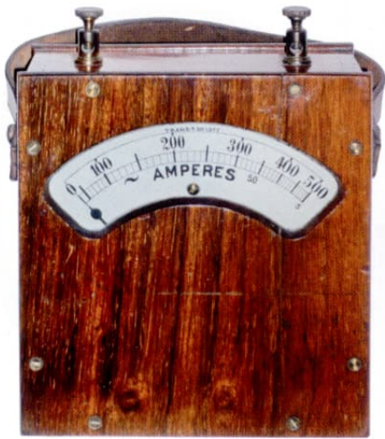
Fig 15: NCS Spring-controlled ammeter (repulsion)
