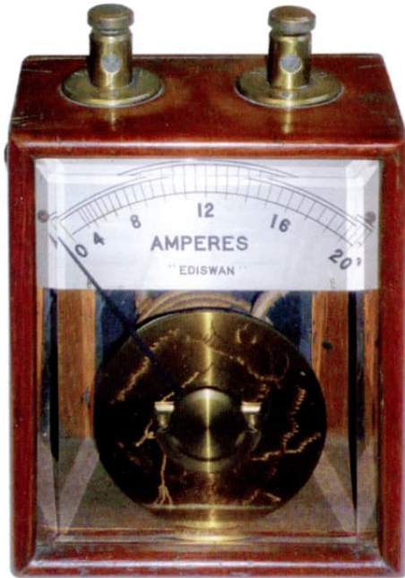
Fig 12a: Ediswan Gravity Ammeter (repulsion) ten-strand insulated wire (Fig. 9c) which could be connected in series or parallel by a commutator (Fig. 9d). This gives two ranges with sensitivities differing by a factor of ten, whose initial purpose was to allow calibration at a lower current than it was designed to measure. To do this a standard 1\Omega resistance was incorporated and from the readings with and without this, and the known battery voltage, it was possible to calculate the sensitivity constant in Webers per degree.
