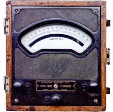
Figure 27. Sangamo Weston voltmeter
