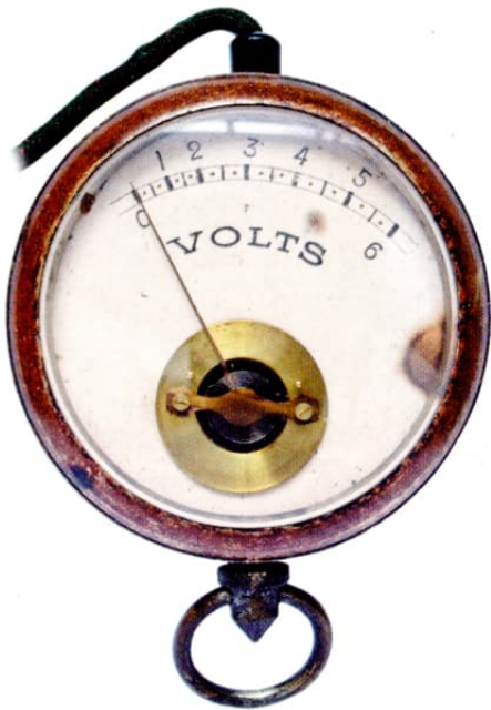
Figure 16. 'Watch case' repulsion type
