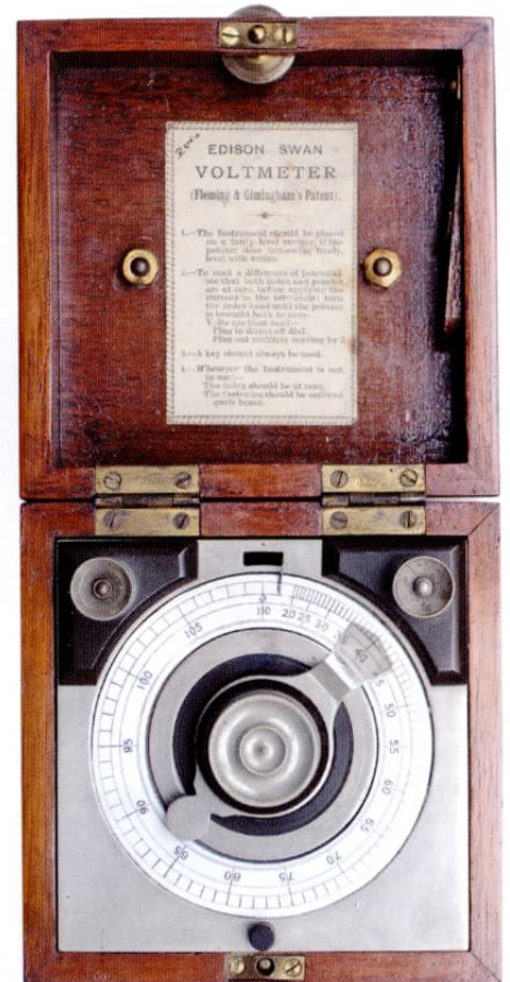
Figure 18. Fleming & Gimingham electrodynamic type
