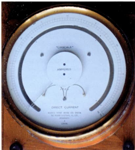
Fig. 2 A Cirscale sub standard ammeter. The overall diameter is 22 cm (8 1/2") and it weighs 6 kg (13.2 lb).
