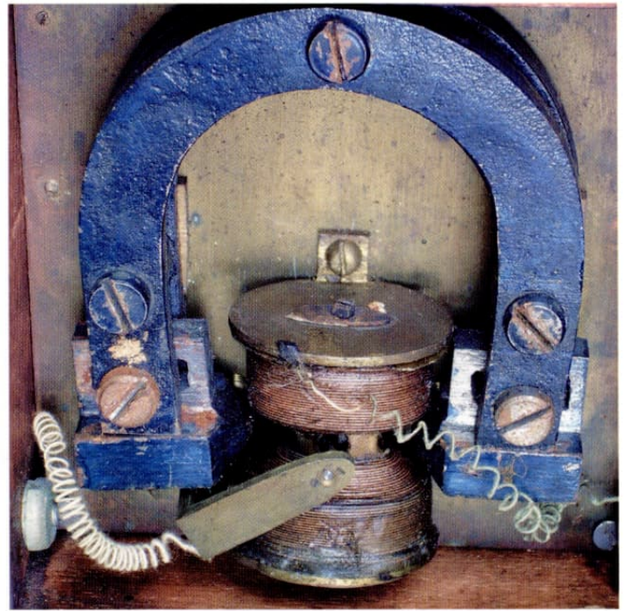
Figure 11B. ECC moving magnet voltmeter
