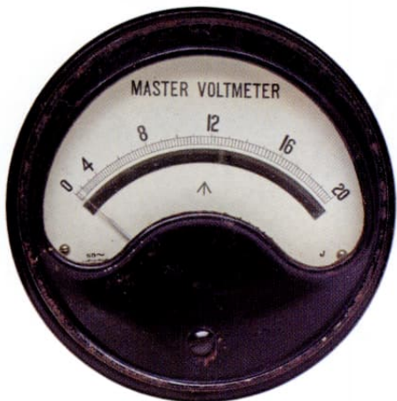
Figure 15. MV moving iron repulsion type
