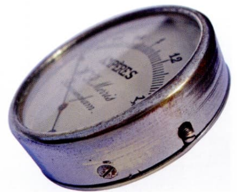
The Ammeter adjusting screw
