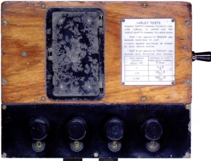
Fig. 16a: Record Bridge-ohmmeter
