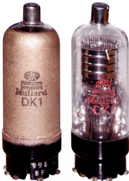
Figure 5: Two examples of the DK1 frequency changer valve. The one on the left has golden-coloured metallising and was the original valve from the 5214.
