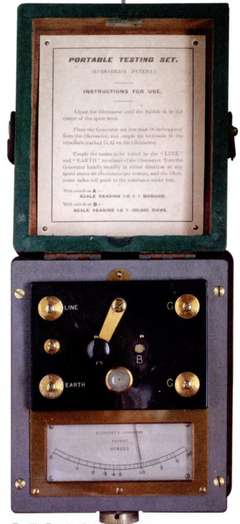
Fig. 7b: Evershed's 1895 ohmmeter
