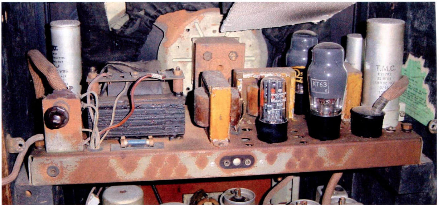
Rust as far as the eye can see
