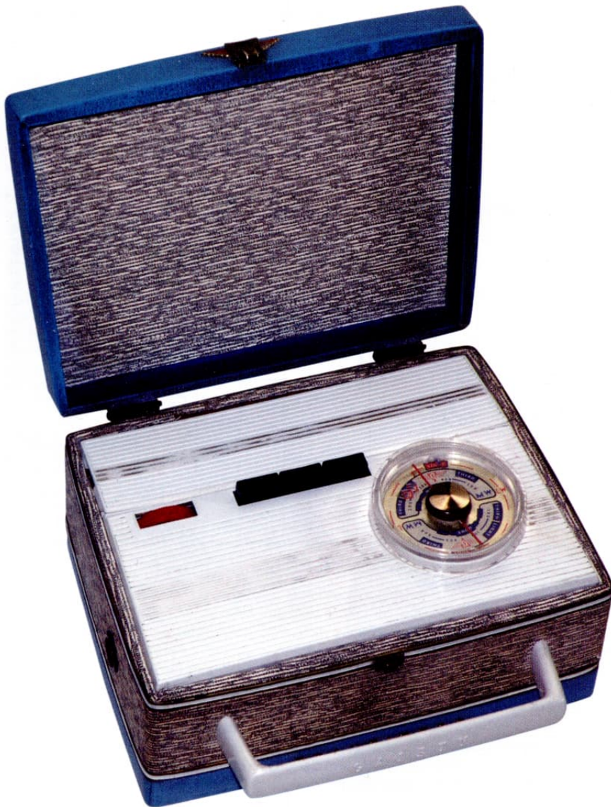
Figure 2: The Kolster-Brandes Gaiety QP21 radio, after a good cleaning. To the right of the volume control, left-to-right the push buttons are: On/off, MW and LW, though no markings can be seen on the case or on the buttons themselves. The grey-ish looking strips on the speaker aperture are partially worn-off gold paint. The handle has 'Gaiety' moulded into it, though this is hardly visible after cleaning
