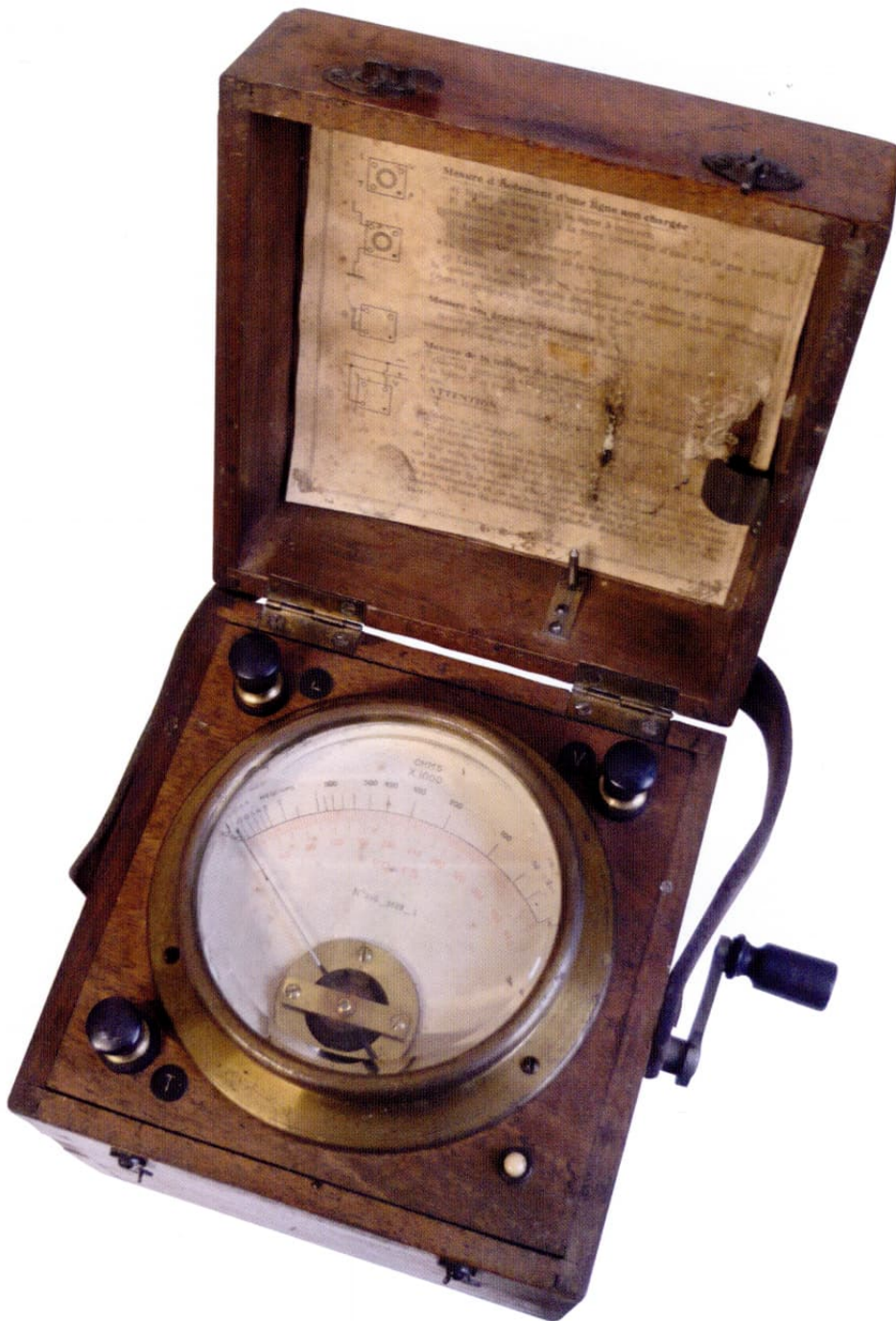
Fig. 8: French ohmmeter relying on correct voltage
