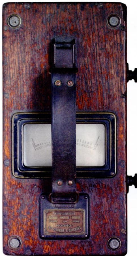
Fig. 11a: Evershed & Vignoles moving-coil Megger
