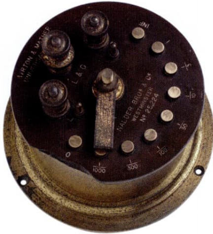
Fig.7 Ayrton & Mather universal shunt, Nalder Bros and blanking off the former 'mV' terminal holes. The 1930 re-calibration certificate shows that the Weston movement took 32.4mA fsd (31Ω/V) whereas No.1312 takes 24.7mA fsd (40.4Ω/V). The AC modification is labelled 'Dorking Century Test Set' on its separate calibration certificate and is presently accurate to within 2%.
