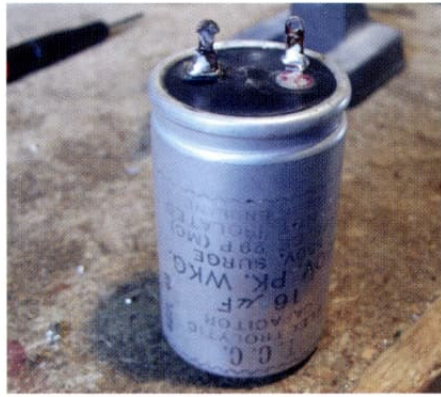
Fig. 9: New leads soldered to existing tags
