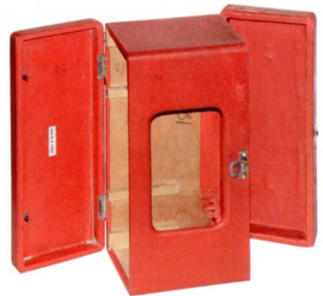
Figure 6: The restored cabinet before the chassis was re-fitted. The batteries are inserted through the case bottom and I think were originally held in place inside cardboard tubes. My radio has the serial number B5551, engraved on a small plastic plate, attached to the inside of the bottom cover.
