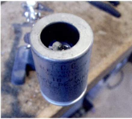
Fig. 8: Replacement capacitor installed
