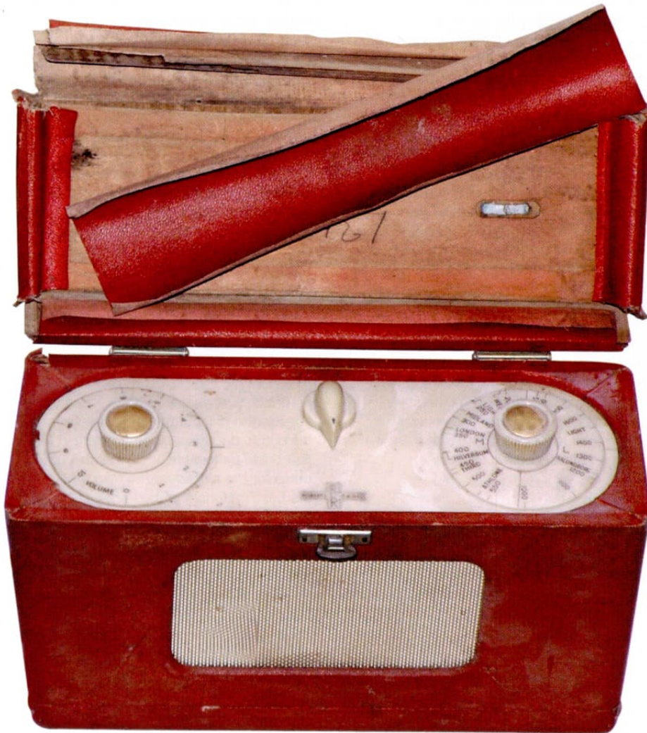
Figure 4: My R88, as donated for restoration by Mike Barker. The radio has a hinged lid over the controls and a hinged bottom cover, giving access to the batteries, and the chassis fixing screws and brackets. The lid looks as if it has been immersed in water for some time, and has also suffered considerable woodworm attack.
