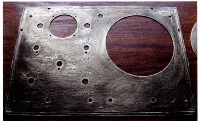
Fig. 6: Front panel cleaned & ready for spraying
