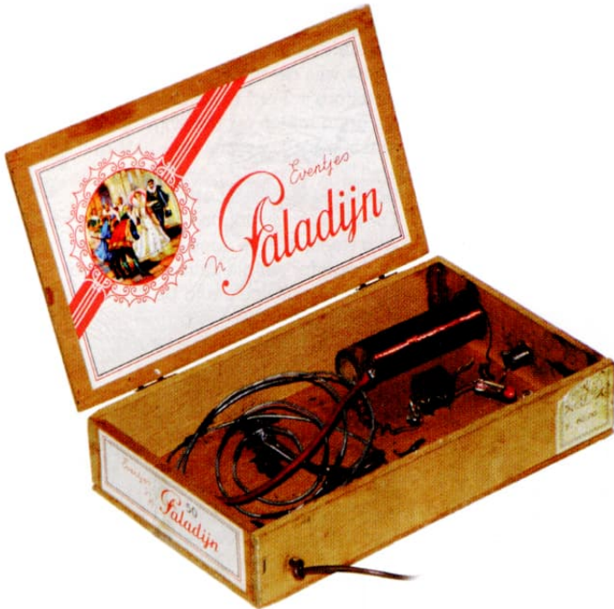
Figure 1: A crystal set built into a small cigar box, as purchased recently at Harpenden.
