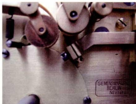
Photo 6b: Detail of reliefwriter from 1861
