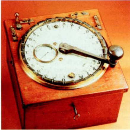
Photo 2: His second model of the dial telegraph
