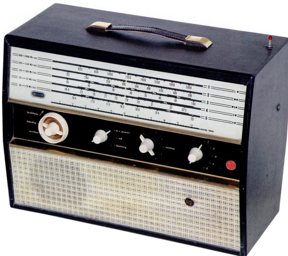
Figure 1: The Pye P94MBQ/LW portable/mains radio, fitted with its smart new carrying handle. The telescopic aerial can be seen extending slightly from the top of the radio, and an external aerial socket is mounted on the right hand side of the cabinet. My radio has a black cabinet: I have also seen an example with a brown finish.
