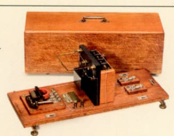
Early wireless telegraphy receiver after a design by Marconi, with coherers by Max Kohl, 1903 (Euro 2.500 – 4.000)
