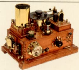
Giant rarity: Detector + Morse Receiver, c. 1910 Compact laboratory experimental unit for very early wireless data transfer! – (Euro 5.000 – 8.000)
