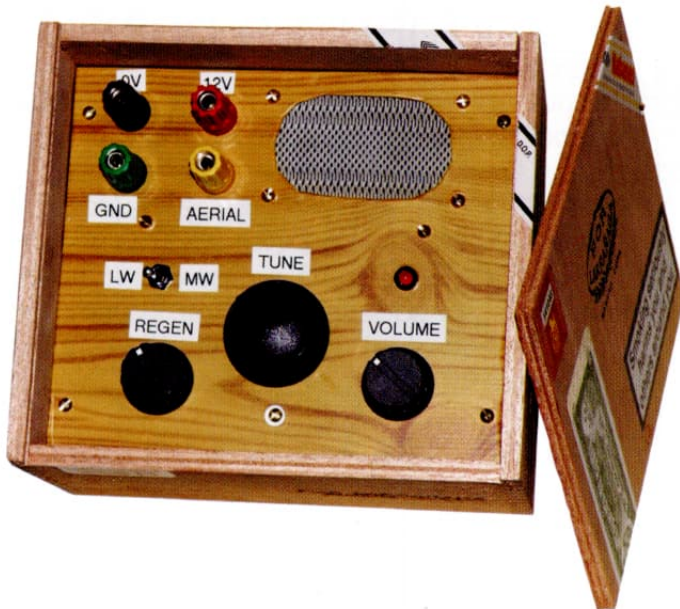
Figure 5: My cigar box radio showing the front panel controls, with the slide-on lid to the right. The aluminium front panel was covered with self-adhesive wood effect vinyl.
