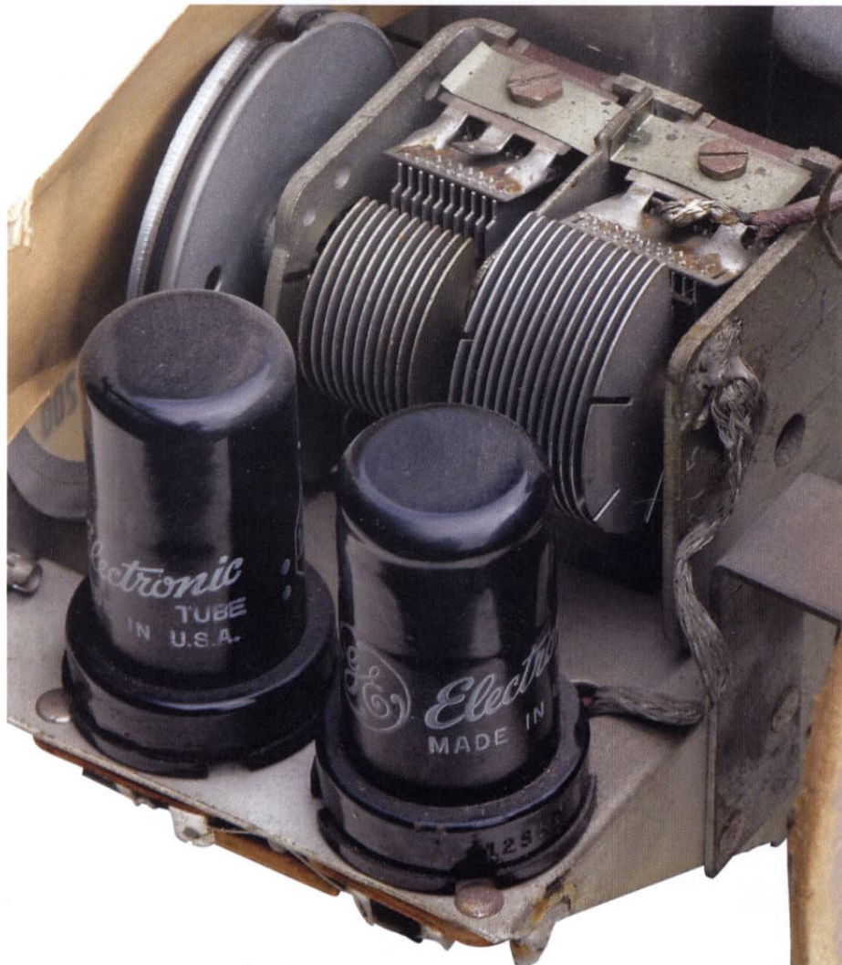
Figure 10: Close up of the RF amplifier and frequency changer stages of the 1000-series radio. You can see the different size plates (and hence the different capacitances) on the two gangs of the tuning capacitor, which make it easy to achieve good tracking across the single band covered.
