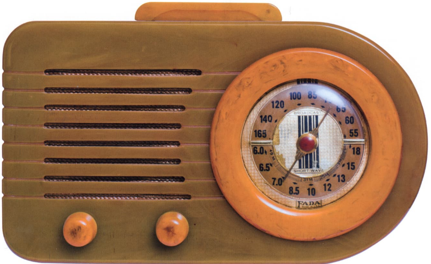
Figure 1: The classic pose of a Fada Bullet radio: a model 116 - short and medium wave, five-valve superhet. Photo courtesy of Carl Glover.
