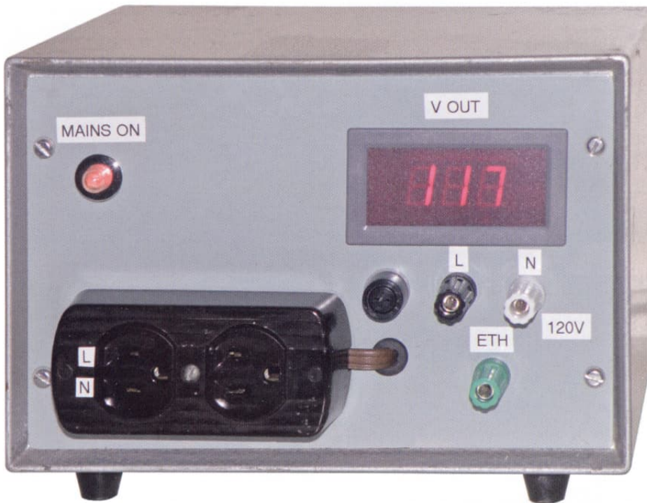
Figure 1: Front view of the completed power supply.
