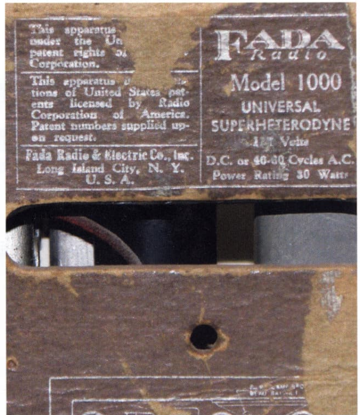
Figure 13: Detail from the back panel of the model 1000. The radio's model number and six valve line-up is printed on the panel. Previous models, and some examples of the 1000, had a label stuck onto the bottom of the cabinet containing this information.
