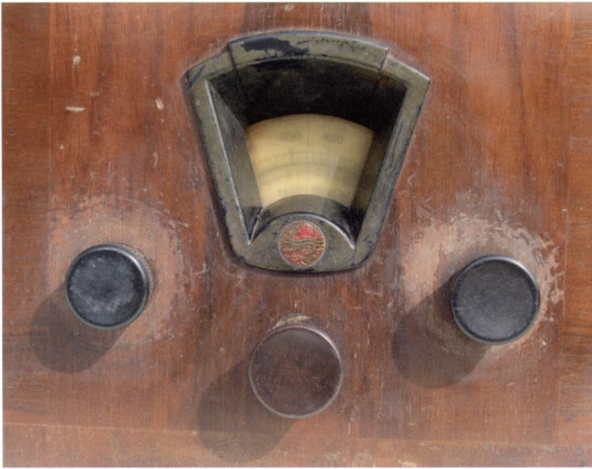
Front Panel wear around the controls
