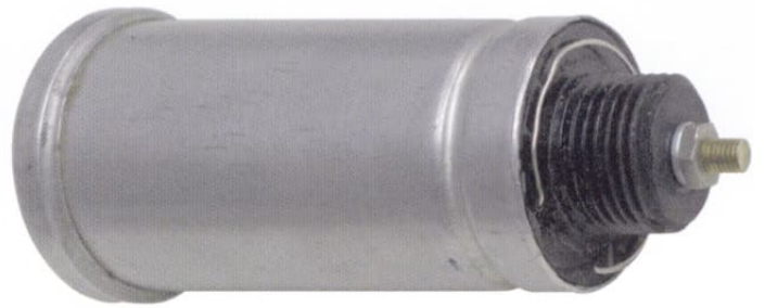
The Re-assembled Smoothing capacitor showing the negative wire
