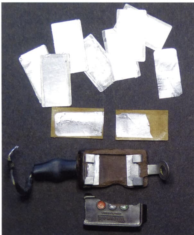
A leaky Micamould cap
