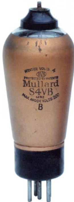
One of the re-sprayed Valves with a new water slide transfer
