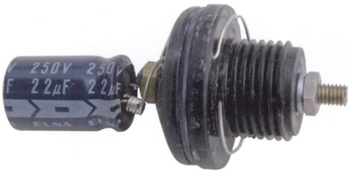
The Smoothing capacitor end plug with new capacitor
