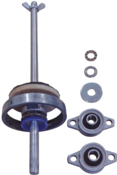
Fig 5. The supply reel - parts spindle and bearings two M5 nuts spaced about 25 mm apart which were soldered directly to the lower end of the brass carriage. A plastic slide connected to the upper end of the carriage slid along a brass tube. The stepper motor was out of a fax machine and had 20 steps per revolution. A 'Johnson Electric Unipolar Stepper Drive' that was purchased from RS (RS number 443-0102) was used to drive the Stepper Motor. The Stepper Drive has its own internal oscillator that could be varied by a Pot, which set the speed that the motor runs at, its frequency was set as high as possible without the Motor losing torque.
