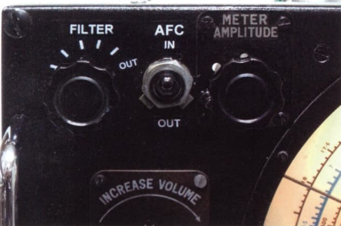
The AFC switch in place
