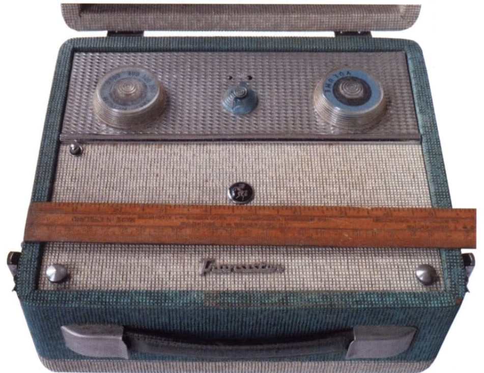
Fig 11. The Invicta model 30, early British 'all transistor' radio
