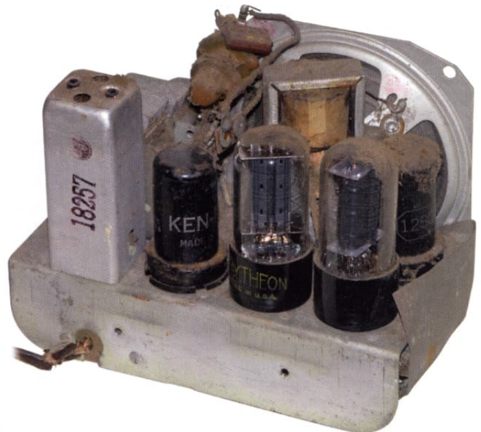
Figure 7: Rear top view of the chassis removed from the cabinet, with a deep covering of dust.
