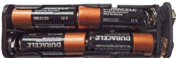
Fig 7. HT battery holder made from a cut-down AAA holder
