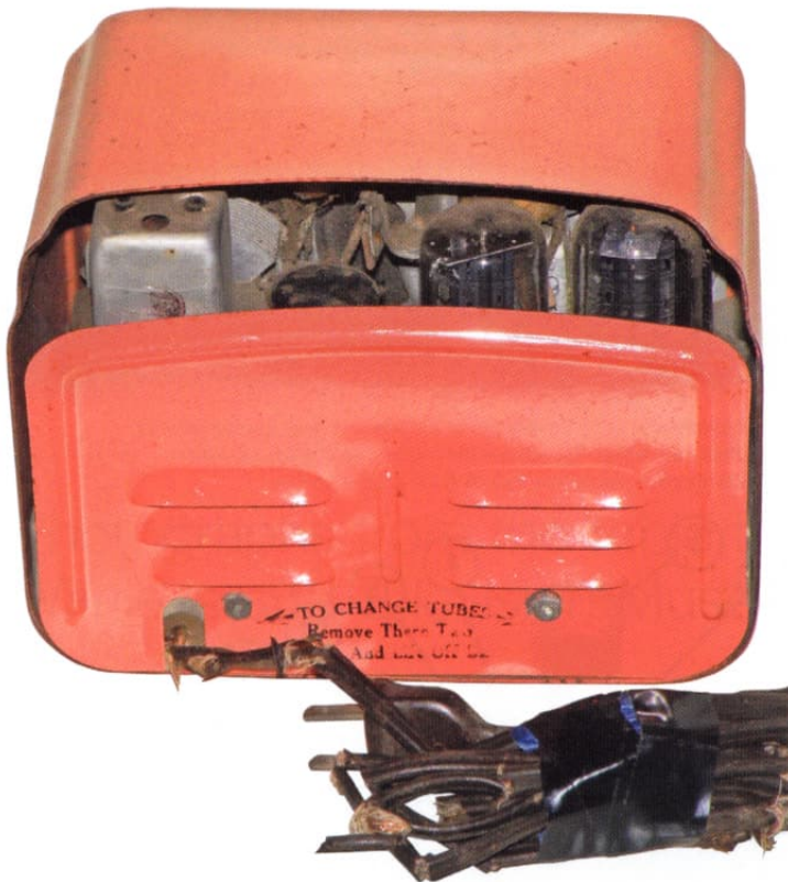
Figure 6: Rear view of the radio, showing the three-quarter height of the back panel, and the terminally perished mains lead that was swiftly removed.
