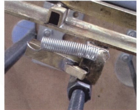
Fig 15. Transverse - carriage to lead screw coupling
