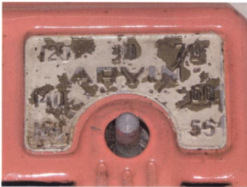
Figure 11: The radio's dial, as found. The thin white coat of paint was easy to remove, leaving the gold-coloured dial underneath.
