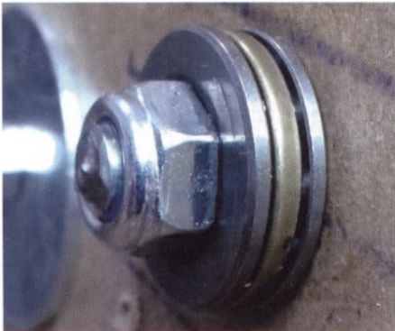
Fig 13. Transverse - lead screw thrust bearing
