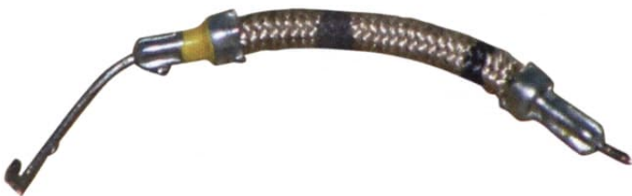
Figure 8: The strange, flexible 47Ω resistor, which measured open-circuit, and was replaced by a 'normal' resistor.
