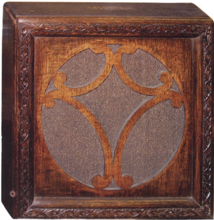
Figure 12: Celestion cone speaker of 1928 vintage. Seems ideal to match to the first generation pentode audio output valves.
