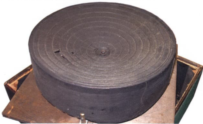
Figure 13: Parchment cone reinforced with a 10 turn spiral of 1mm square bamboo on front side. Glued to a paper cylinder at the cone edge
