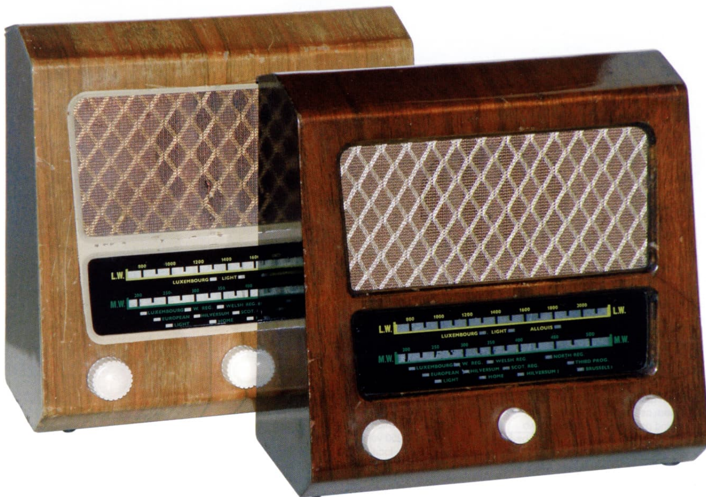
Figure 1: The two radios posed together. As you can see, from the front there's no way of telling which one is which, the dials and control layouts being identical. In fact the superhet is at the front, with the darker cabinet, and the TRF is at the back. The TRF's cabinet's sides are painted, rather than veneered as the superhet's sides are.
