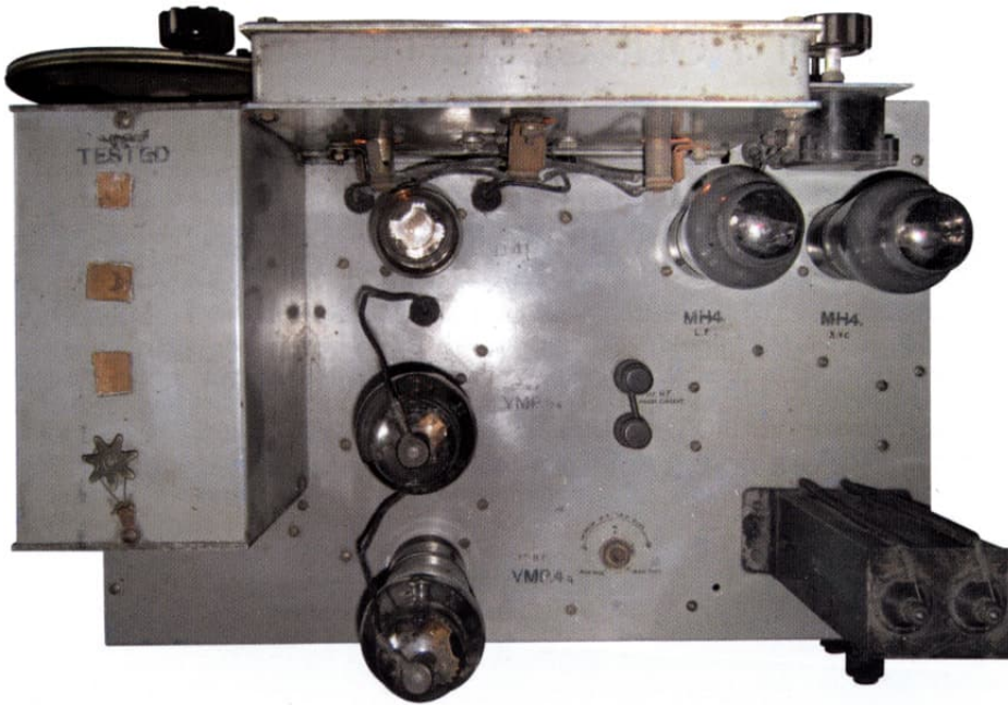
Damp damage to second Colvern coil set
