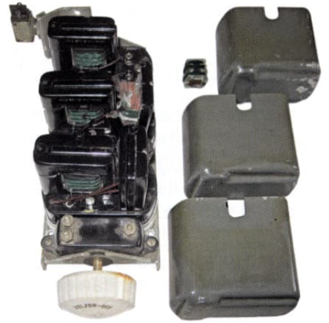
Damp damage to second Colvern coil set
