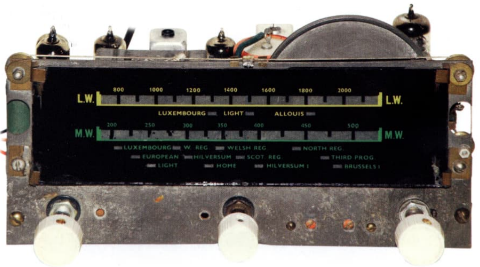
Figure 7: Front view of the superhet chassis. At this stage I hadn't replaced the dial lamp, which fits into the hole to the right of the dial. Left to right, the controls are: volume and on/off (using a double pole on/off switch on the 500k volume control); tuning; and the medium / long wave bandswitch. An identical dial was used for the TRF version of the radio.
