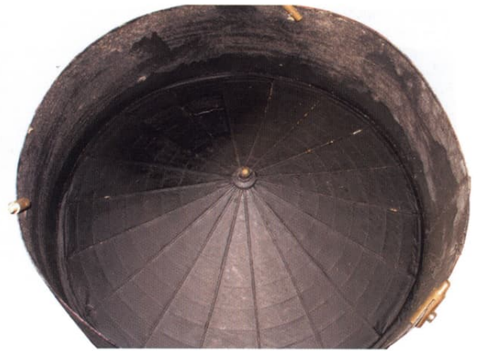
Figure 14: Eighteen bamboo radials support the back side. I wonder how much labor was required to fabricate these in volume production?
