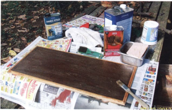
Figure 6: Removing the polyurethane varnish on the salvaged board and staining to match the original cabinet was no small task.
