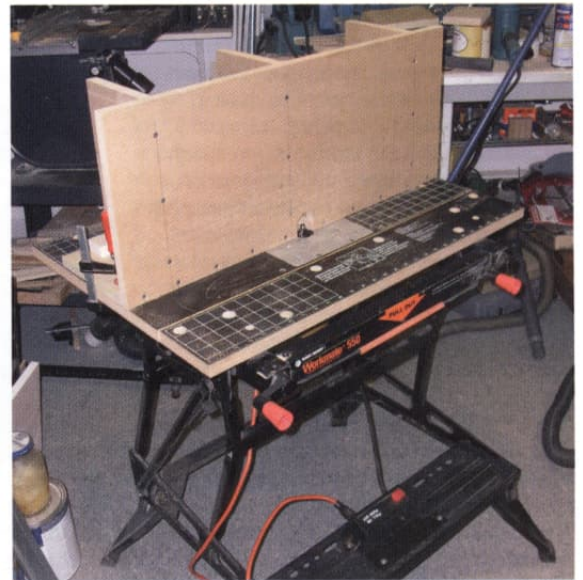
Figure 5: My modifications of a folding work bench to make a high fence router table.
