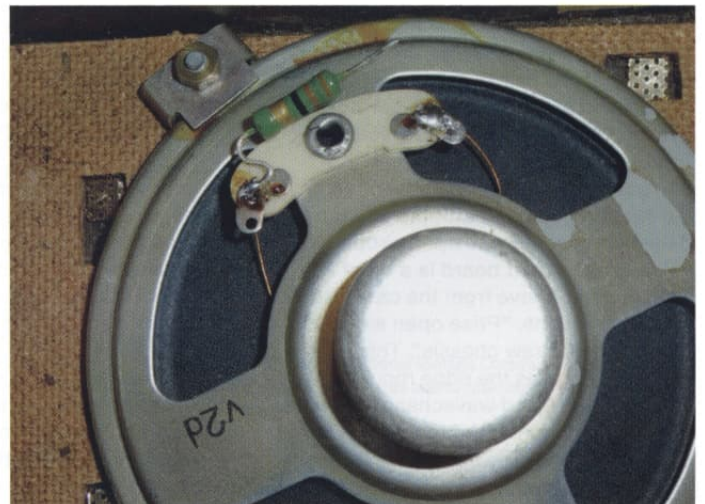
Replacement speaker with series resistor wired direct
