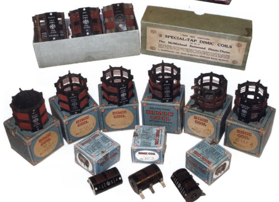
Figure 2: The three coils in one box were standard issue for MW and Daventry. The other 9 coils were optional.
