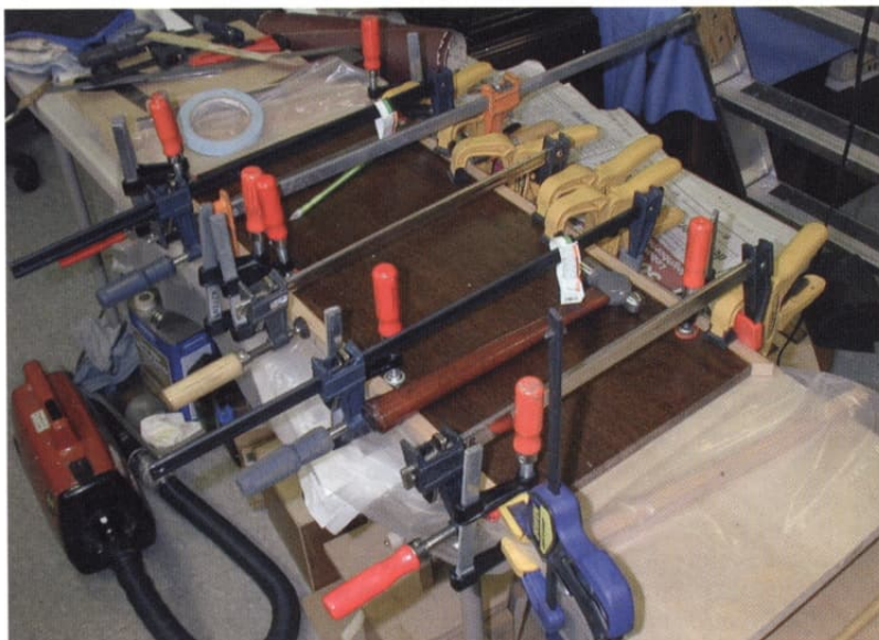
Figure 4: 'Stretching' my available board by gluing-on oak strips to the edges. Proving you can never have too many clamps in the shop.
