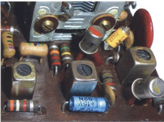
Close-up of tiny IF transformers and Texas transistors
