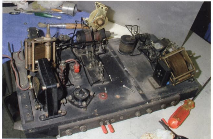
Figure 9: Heavy soil and corrosion on the top side of the chassis demanded all parts be removed for proper cleaning.
