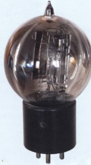
Figure 2A WE Type 205D valve. Revealing their pioneering ancestry, dating from 1917, the early members of the 205 family had globular envelopes. Later valves had conventional stepped envelopes. The 205F, which eventually replaced the 205D was made until 1979!
