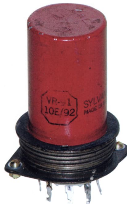
Figure 3 (below): A robust ceramic EF50 socket, with a locking ring which holds the valve in the socket even under high vibration and shock conditions, typical of what could be encountered in military and airborne applications.
