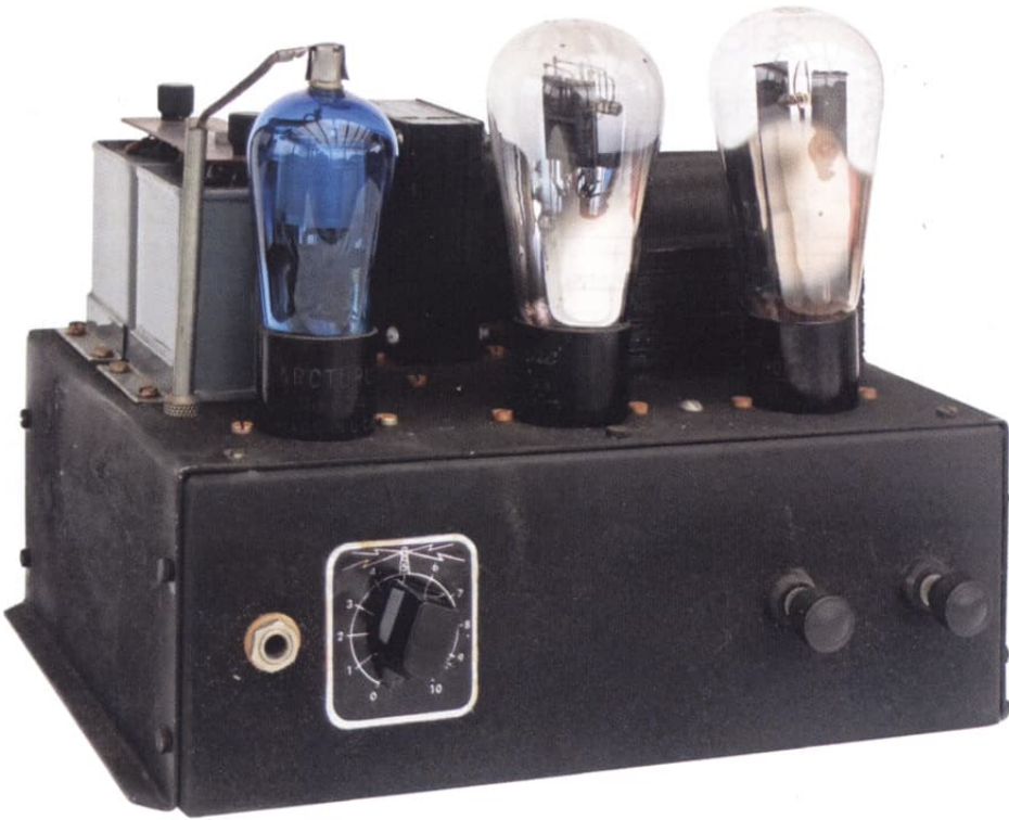
Figure 6: The Loftin-White amplifier shown in Figure 3 as built by the writer. It is very compact when compared with its contemporaries. This example is in frequent use as his workshop amplifier.
