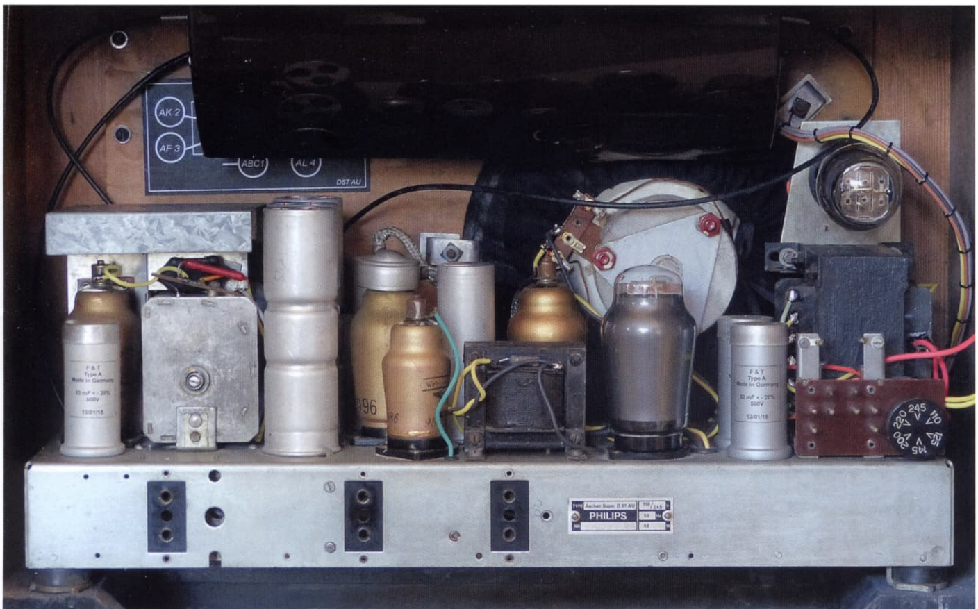
That cableform needs re-routing
