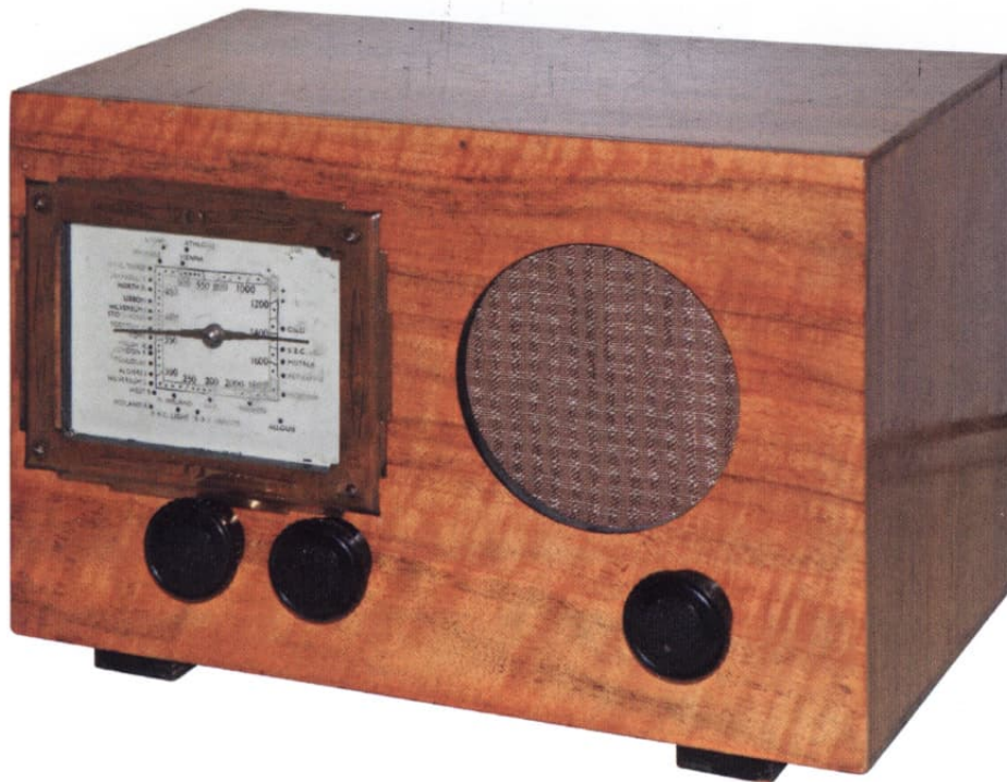
Figure 1 (left): Front view of the restored radio. Hopefully the attractive vintage bronzed edging to the dial can be seen. Left to right the controls are: Tuning, Volume and Wavechange.
