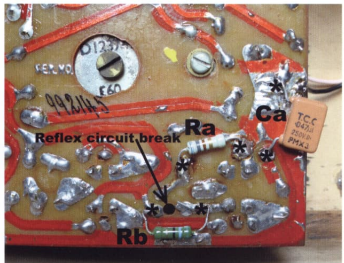
Reflexed board showing break in strip and modification components
