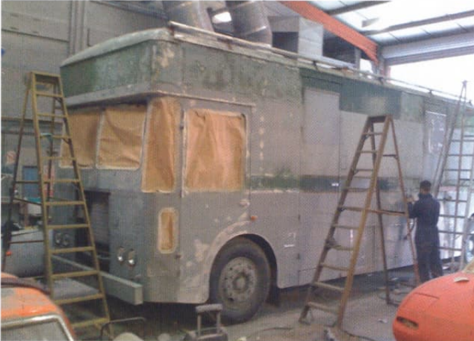
In the spray shop, with all the glass and trims removed
