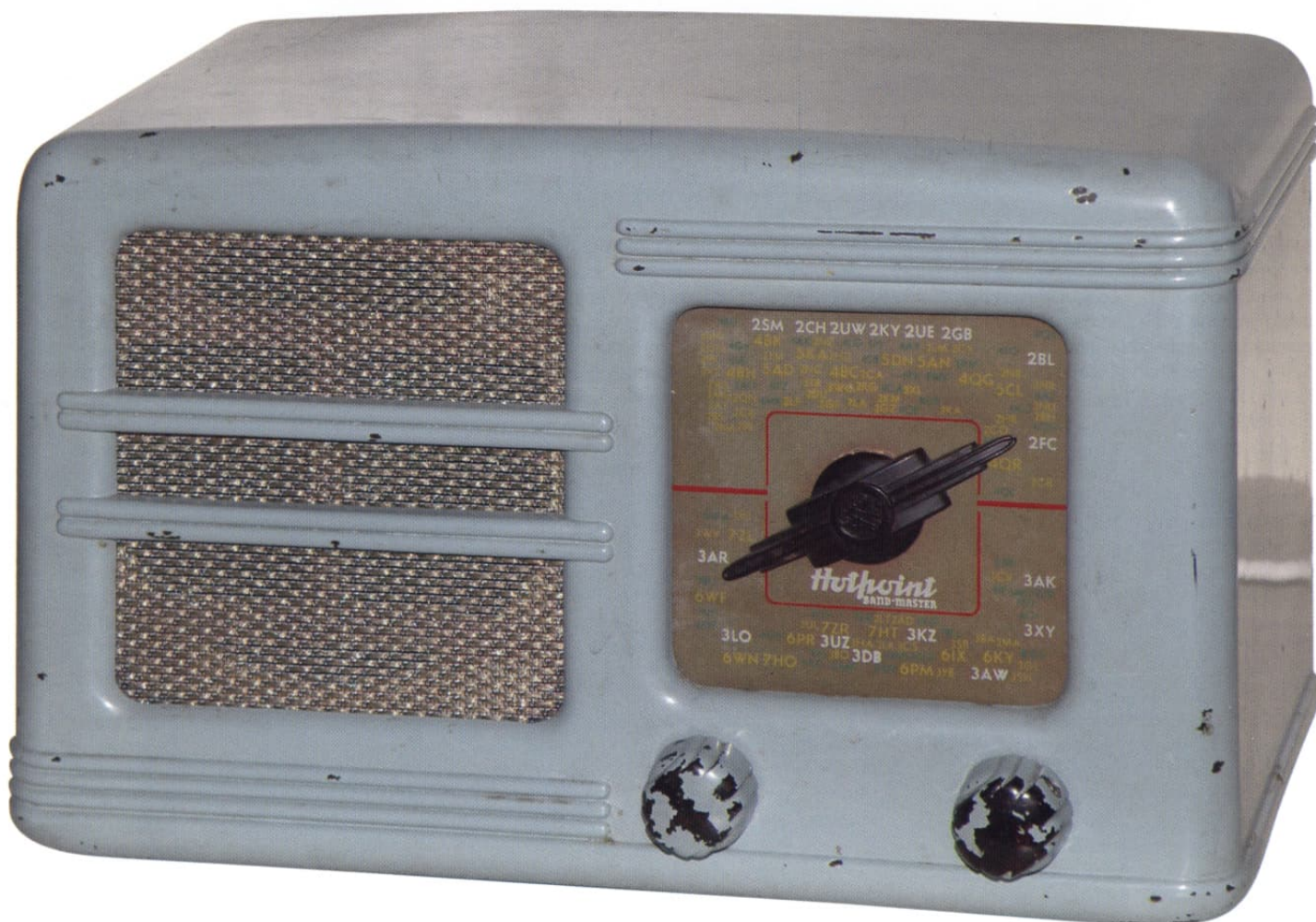
Figure 1: The Hotpoint radio fitted with a new speaker cloth, and with its painted Bakelite cabinet cleaned up.
