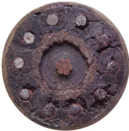
Fig. 13b: 1865 transatlantic cable. 29mm diameter
