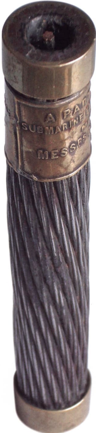
Fig. 8a: 1857/8 transatlantic cable by Glass Elliot & Co. (left hand lay, western half)
