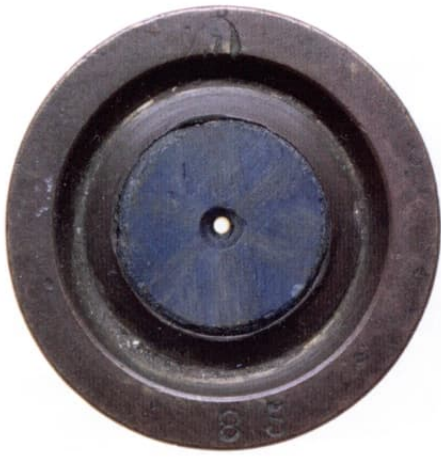
Fig. 6: Feldspar wire drawing die, 30mm diameter
