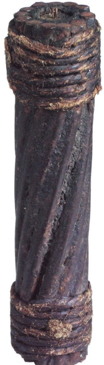
Fig. 9a: 1857/8 shore end cable by RS Newell & Co (right hand lay, Irish end)
