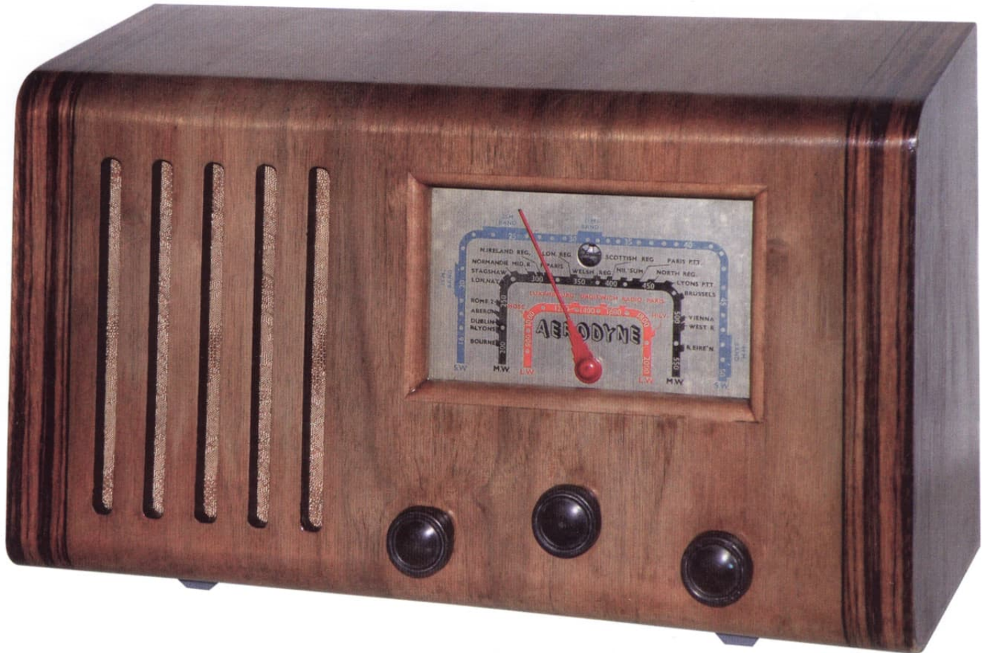
Figure 10: Restored condition of my Alba 472 with an Aerodyne dial. The knobs are original, though I think they let the side down slightly now that the cabinet colour has been lightened.
