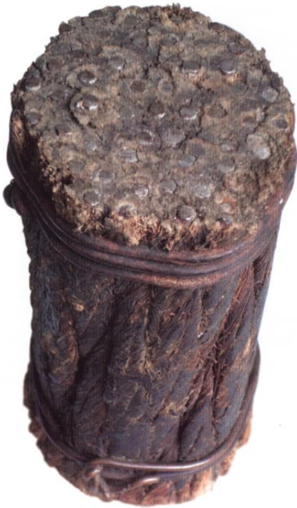
Fig. 16: 49 strand grappling cable for 1866 recovery of 1865 cable. 48mm diameter
