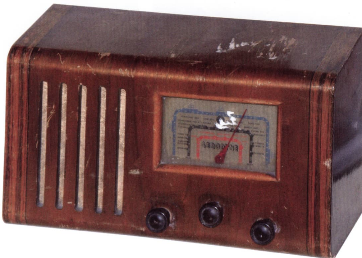
Figure 1: Pre-restoration view of my tired looking Aerodyne-branded (at least from the front) radio. The dial markings look out of focus, but this is because of the thick layer of dust on the inside of the dial glass.
