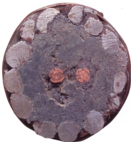
Fig. 27: Reconstructed cable section from Knightstown harbour with five sector conductors. 37mm dia.
