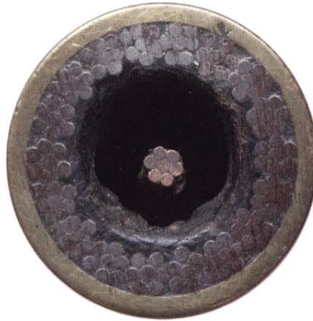
Fig. 8b: 1857/8 transatlantic cable by Glass Elliot & Co. (left hand lay, western half) 17mm diameter
