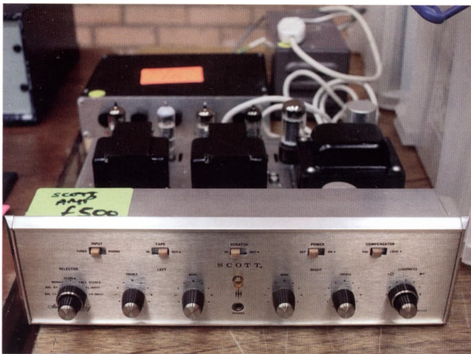
1960's Scott 4 x ECL86 stereo amplifier (note the dud valve)
