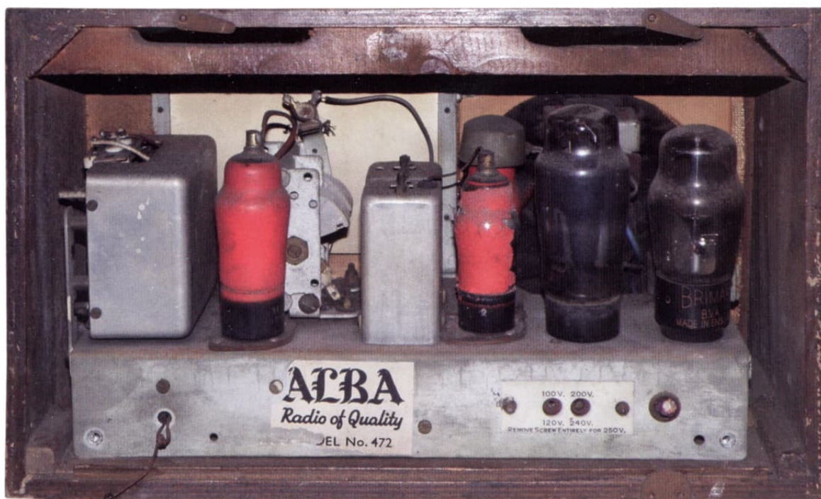
Figure 2: Rear chassis view before restoration, clearly showing the Alba model 472 identity of the radio. The rolled-up throw-out aerial can be seen emanating from the left side of the chassis.
