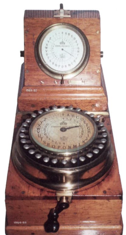
Fig. 5: General Post Office ABC telegraph sender & receiver (Science Museum London)
