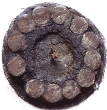
Fig. 9b: 1857/8 shore end cable by RS Newell & Co (right hand lay, Irish end) 41mm diameter
