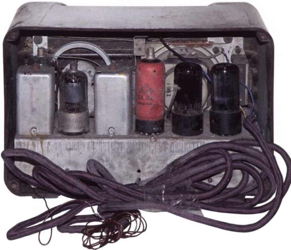
Figure 1: Rear view of the Masteradio radio, with its original mains line cord. The red DK32 in the centre of the view is a cuckoo in the nest.
