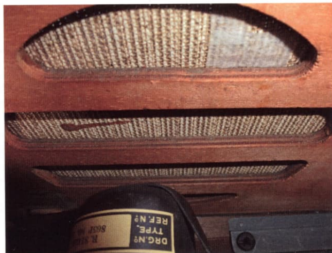
Internal fabric repair to rear cabinet vent (top, right of picture)
