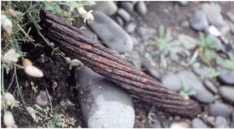
Fig. 20a: Portpatrick four channel cable emerging from beach (presumably same cable as Fig. 19)
