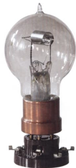
The BTH tape A was a hard valve modelled on the original French TM hard triode of 1915. It was mass produced for the war effort in France and from 1916 in Great Britain. The design formed the basis of all bright emitter triodes and valves such as the Ediswan and MOV V24 in the early days of broadcasting.
