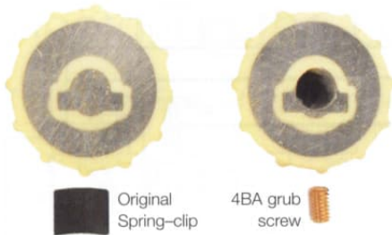
Fig 4: Spring-clip removed, knob filled, drilled out to 6mm, and a 4BA grub screw fitted in the side.
