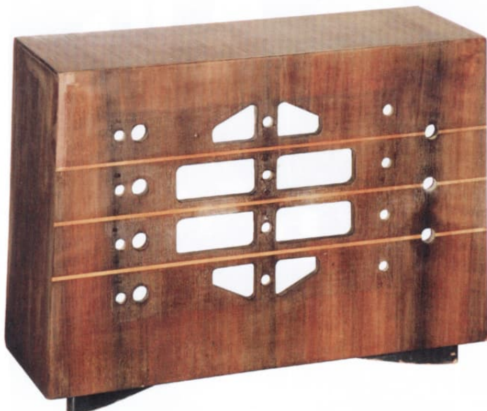
Figure 6: The stripped down cabinet, with the repair to the veneer in the top left hand corner, awaiting varnishing. I've been careful not to rub down the surface too much, to retain the 65 years old patina. The central openings allow the sound from the 8-inch Goodmans speaker to escape.
