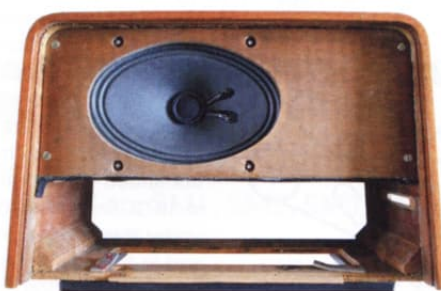
Fig 14: The new speaker installed
