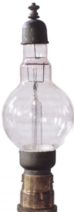
GW White developed a soft triode at the Cavendish Laboratory in 1917. It was used as an RF amplifier in the Mk III tuner.
