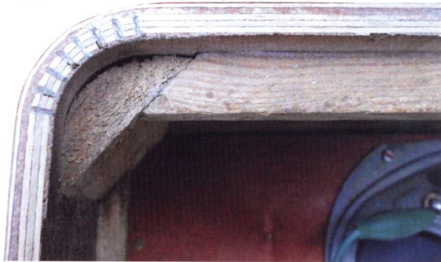
Fig 3: 'Kerfed' bends on cabinet corners
