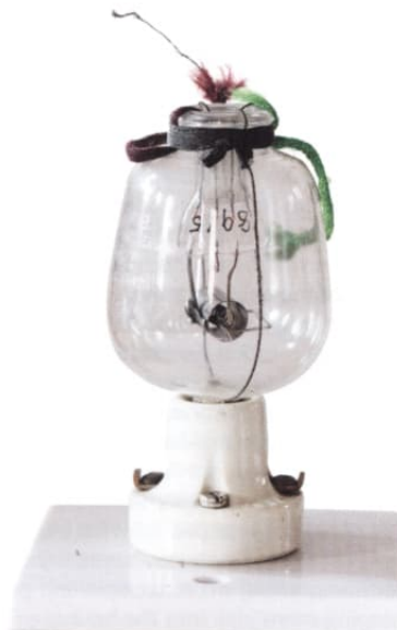
The GEC R2 was made to replace the BTH Audion, at first with a nitrogen fill and later helium. It was the last soft triode to be developed in WWI.
