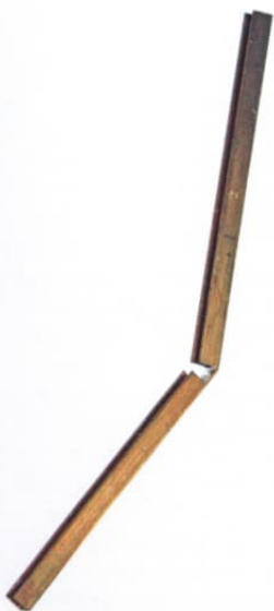
Fig 5: Cutout made and bend commenced
