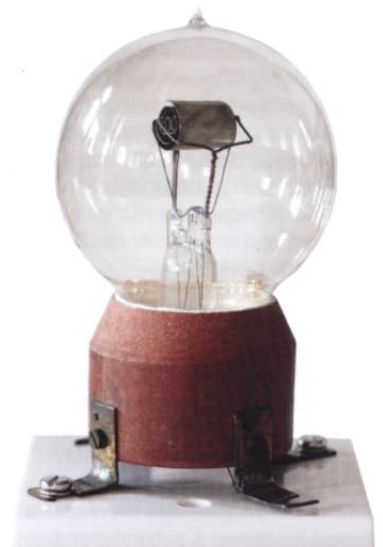
The Post Office Valve, Amplifying No.2 was made c.1919. This example has a sheet nickel anode. Some samples have been seen with a wire spiral anode. It was manufactured by BTH.
