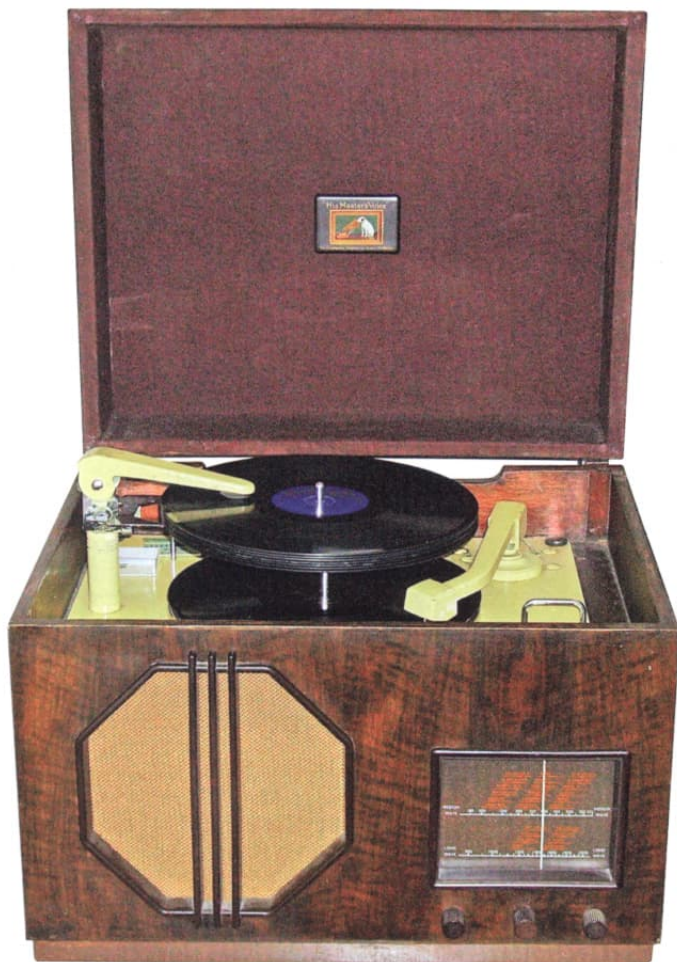
Figure 1 (below, left): The ten inch diameter record stacking ledge in position. No provision is made for manual operation as pressing the autobutton is so simple. To stop the mechanism before all records have been played press down fully OFF. The arm will return to its rest as the mechanism disengages and the motor switches off without dropping the next disc. To resume playing press down fully AUTO and the next record drops. Also AUTO can be used to reject onto the next record
