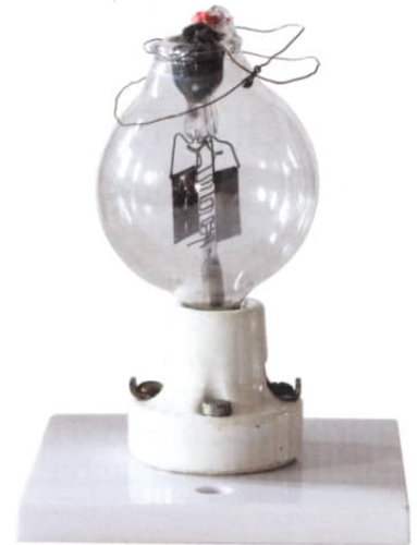
BTH made a replica of De Forest's Audion soft triode around 1917. It was used by the Royal Navy but was discontinued due to reported manufacturing problems.
