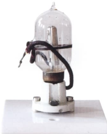
JA Fleming developed Edison's diode-effect lamp, patented in 1884, as a demodulator or detector for a Marconi-Fleming receiver in use around 1905-1906.
