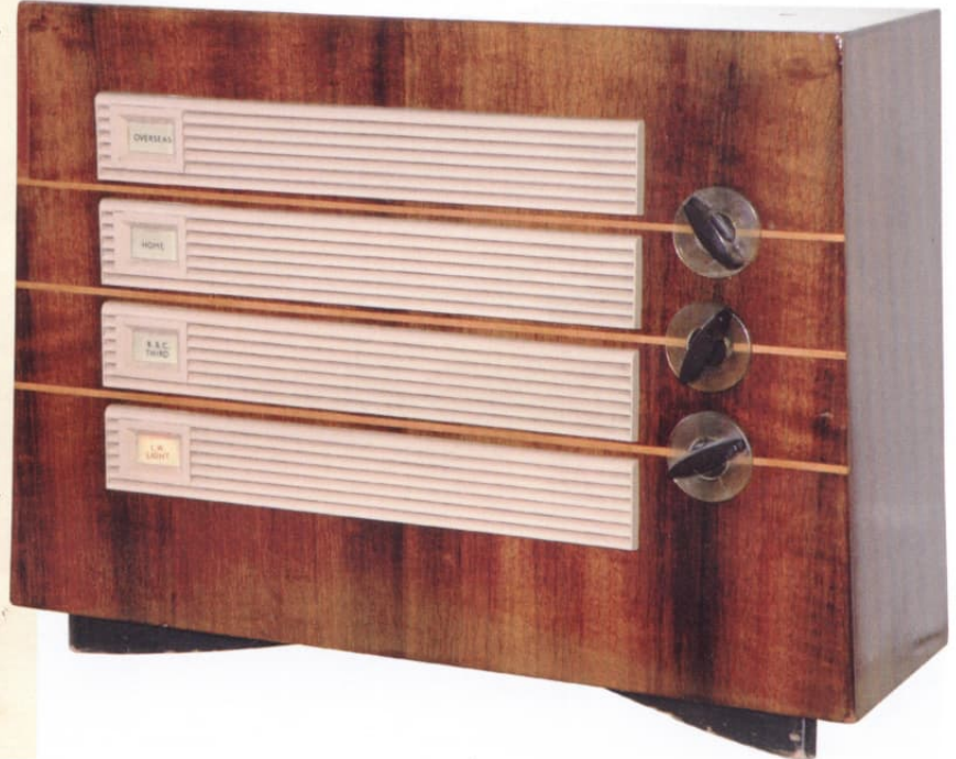
Figure 14: The A147 in restored condition, showing the distinct obelisk shape of the cabinet. The four plastic strips are attached separately and effectively form the grille over the 8-inch speaker. The radio is tuned to what is now BBC Radio 4 on 198kHz, as indicated by the 'LW Light' lamp being lit. Additional labels, other than those shown, were provided with the radio, but not surprisingly these have been lost over the years. When the station selector switch is set to the 'gram' position, the top and bottom lamps are both lit.
