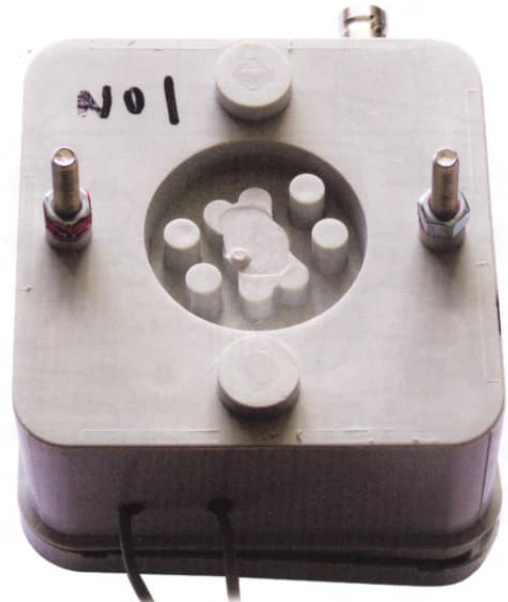
Captive 2BA fixing bolts through the box
