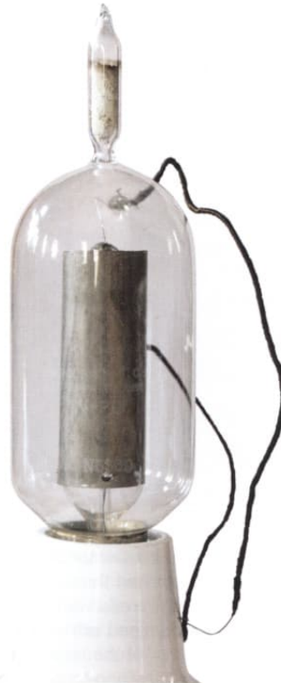
HJ Round of the Marconi Wireless Telegraph company developed a soft triode around 1913. It was used throughout much of WWI and manufactured by Edison Swan.
