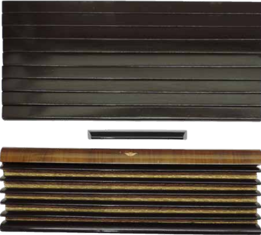
The roll top and louvered grill ready for re-fitting into the cabinet after refurbishment and spray painting in the final colour matched cellulose paint.
