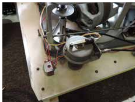
Close up of the lock solenoid assembly and the motor supply contact.
