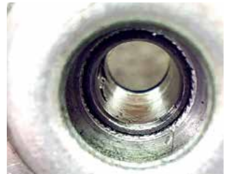
Although difficult to spot at first, the image captured here via an endoscope camera shows sections of wear seen inside the motor bearing housing, and was part of the cause of the stiffness found with-in the motor in general.
