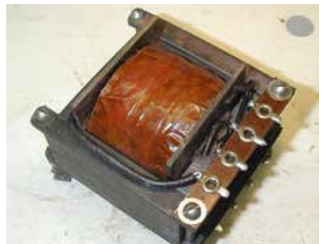
Fig. 17 – Transformer after cleaning and rebuild. It looks like NOS (New Old Stock).
