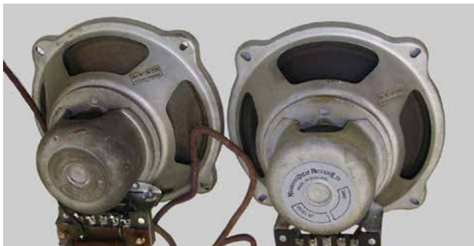
Fig. 26 – Note how well one of the speakers cleaned up after an application of phosphoric acid "rust converter".
