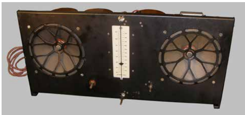
Fig. 24 – Front of chassis showing robust Magnavox brand loudspeakers.
