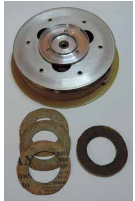
The underside of the turntable showing what was found including the paper spacers cut out from a newspaper. It's anyone's guess as to how it ended up like this in the first place.
