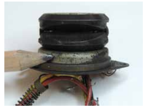
The recording head completely dismantled. The general dirt and dust that was found can be seen prior to cleaning. The slot can be seen where the wire travels across the head which is a combined type and incorporates the bias, erase and record/replay windings.
