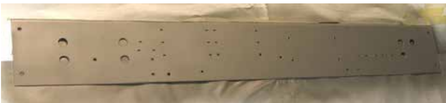
Fig. 14 – Rear panel of chassis stripped of hardware, masked and painted.
