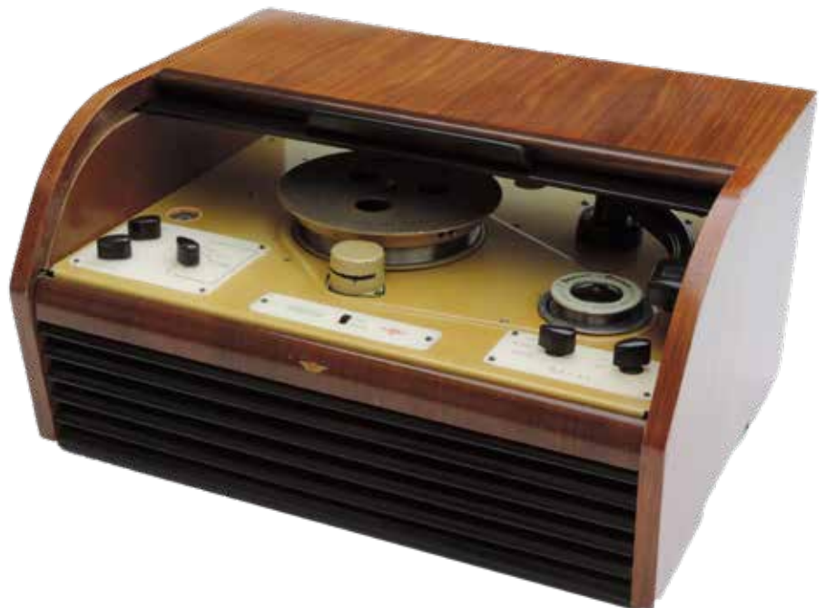
Fully restored: The KB wire recorder in all its splendour, reassembled into the cabinet.
