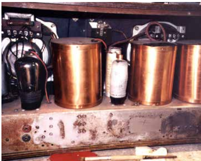
Fig. 3 – 1996 photo of rust on chassis.
