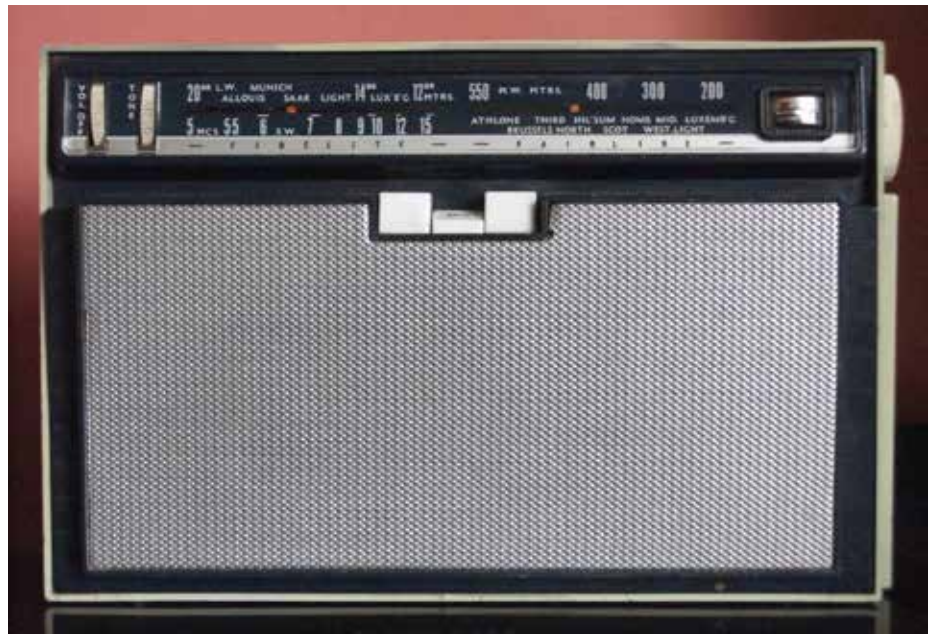
Figure 2: The Fidelity Fairline radio, predecessor of my radio, and with a cabinet looking very similar to the 208, with the three 'piano' keys selecting the band. Note the short wave band, covering 5MHz to 15MHz.
