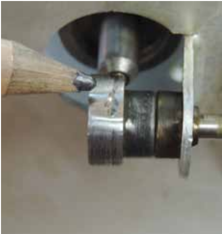
The extensive damage on the play cam can be seen in this picture.
