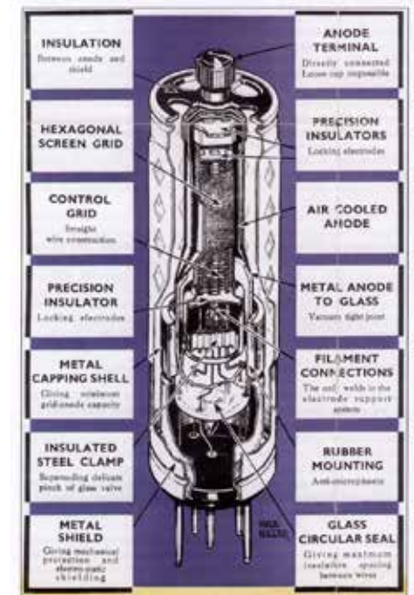
Fig. 38 – Catkin cut away shown in The Saga of Marconi Osram Valves
