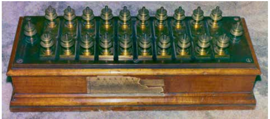
Fig. 5a O & FH Varley's 10-stage artificial cable model
