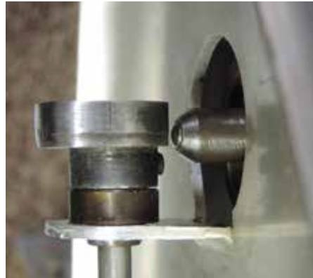
With the turntable drum dropped into the play position the general mis-alignment with the top of the cam can be seen. The bearing should be resting on top of the cam so that turntable drum is lifted clear of the deck plate in play or rewind mode.
