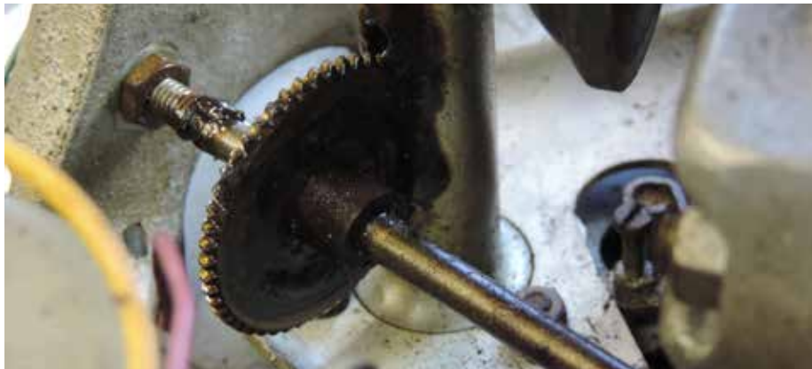
The underside of the worm drive assembly that couples the spool carrier hub to the drive. The muck seen here was almost solid.
