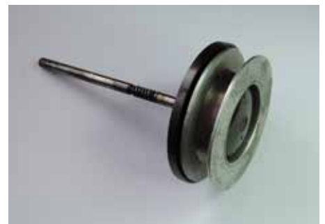
The careful removal of the reel carrier necessitated its complete disassembly from the rest of the deck in order that the wire reel could be freed off, without causing any further damage.
