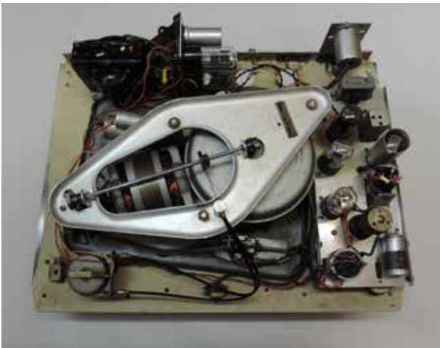
With the turntable drum dropped into the play position the general mis-alignment with the top of the cam can be seen. The bearing should be resting on top of the cam so that turntable drum is lifted clear of the deck plate in play or rewind mode.
