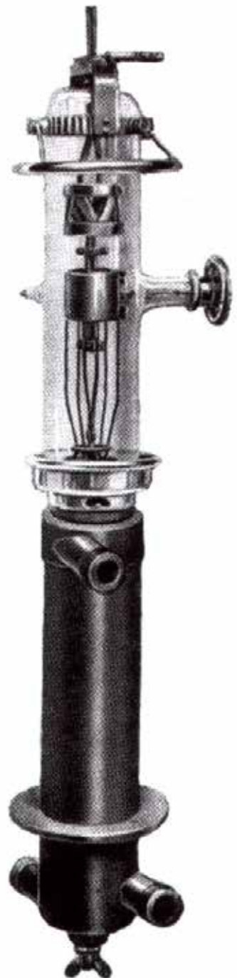
Fig. 36 – CAT water cooled high power transmitting valve.
