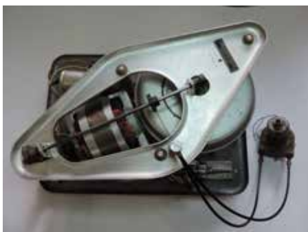
The underside of the deck showing the general transport arrangements, with the Bowden cable controlling the rotation of the cams that are positioned at either side of the deck depending on the positioning of the deck control. The main control mechanism can be seen on the far right which also houses the lock solenoid.
