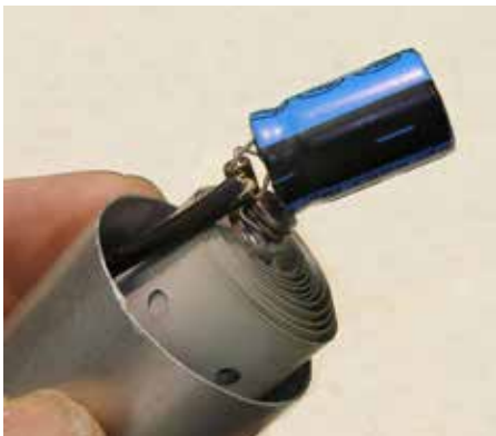
Fig. 20 – Mounting replacement electrolytic to the top of the central aluminum post.
