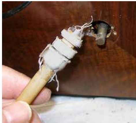
Fig. 10 - Making the cloth bushings and gluing in place.
