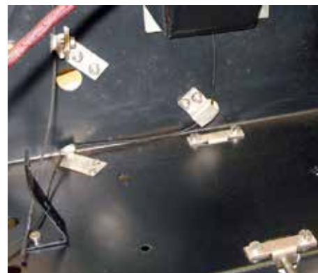
Fig. 32 – Unusual dial string channel brackets
