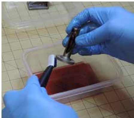
A thorough cleaning of all the major drive assembly parts was the only option. Parts degreaser was used along with various small brushes and pipe cleaners.
