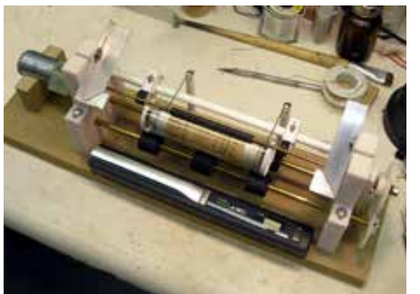
Fig. 18 – My home built Torch Battery scanner to capture the electrolytic condenser graphic.
