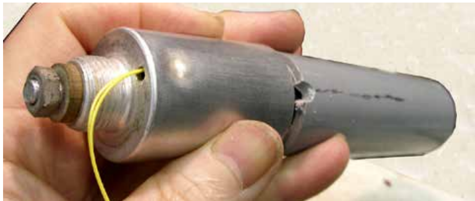
Fig. 21 – Condenser – Wire brought out of base and PVC pipe used to insulate old positive spiral plate.
