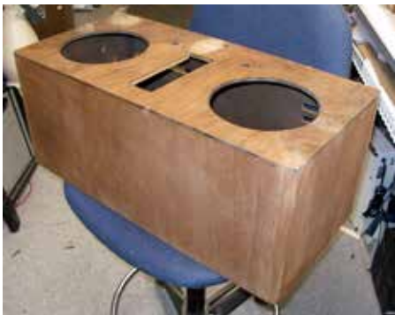
Fig. 7 – Stripped cabinet with patched holes.
