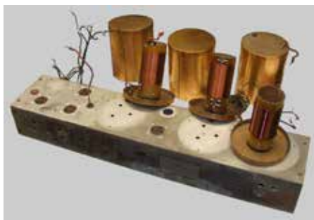
Fig. 33 – To properly clean the top of the chassis I had to get the RF coils and mounts out of the way.
