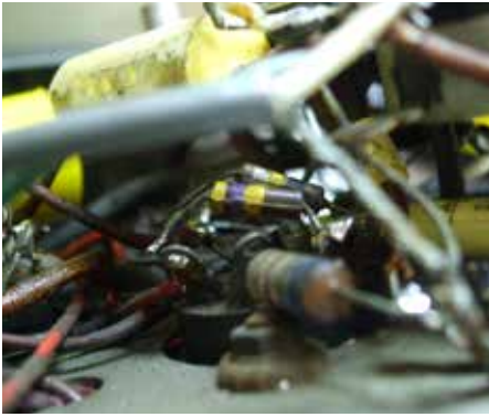
A gut feeling about these two resistors found on V1, proved to be right. Both had nearly doubled in value.
