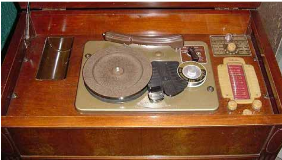
The US produced Silvertone radiogram and wire recorder shows a similar idea for playing 78 only records. Note the level of sophistication in the actual deck compared to the more basic features found on the KB unit.
