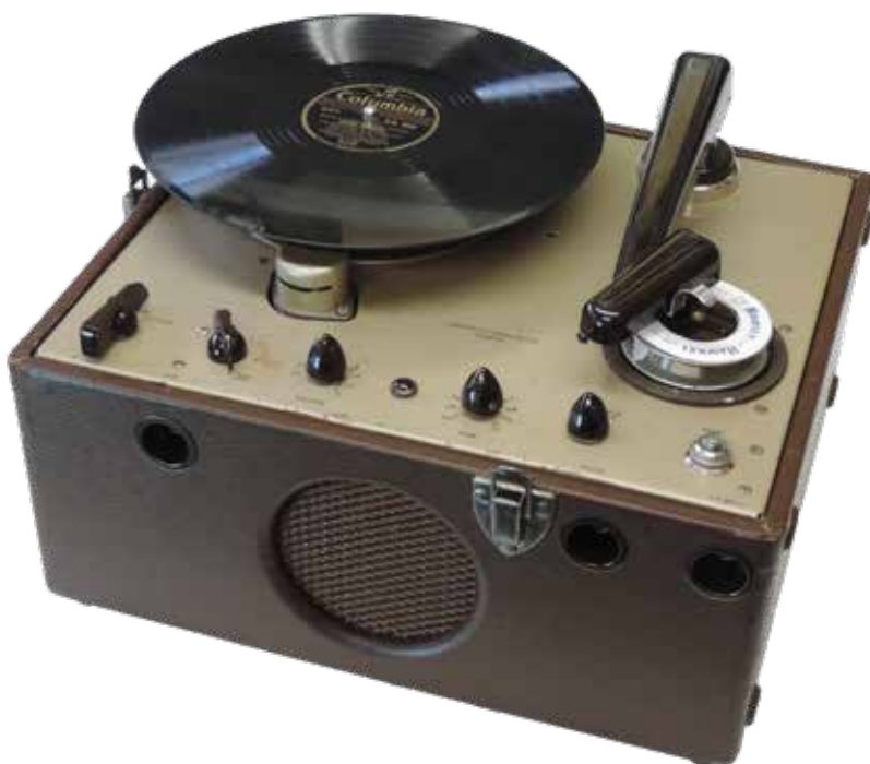
The KB EWR60 shares the same type of deck as the Boosey and Hawkes (Wirek Electronics) Model B1 wire recorder as featured in this picture.
