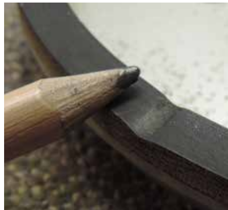
The damage caused to the flywheel rubber rim can be seen here and just goes to show how much damage can be caused by carelessly leaving the deck in the play position for a period of time.
