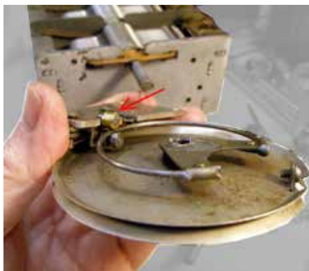
Fig. 30 – The Slo-motion drive for the beautiful Polar brand tuning condenser.
