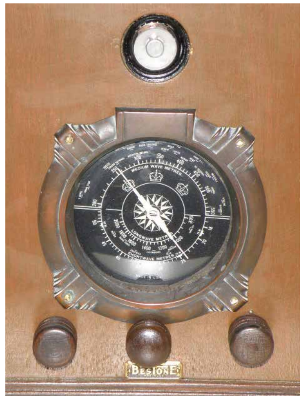
Figure 15: Close-up of the front panel, clearly showing the Bestone branding and the 6E5GT magic eye. The bright colours on the dial do not show up in this view, but have a very attractive effect when the radio is switched on.
