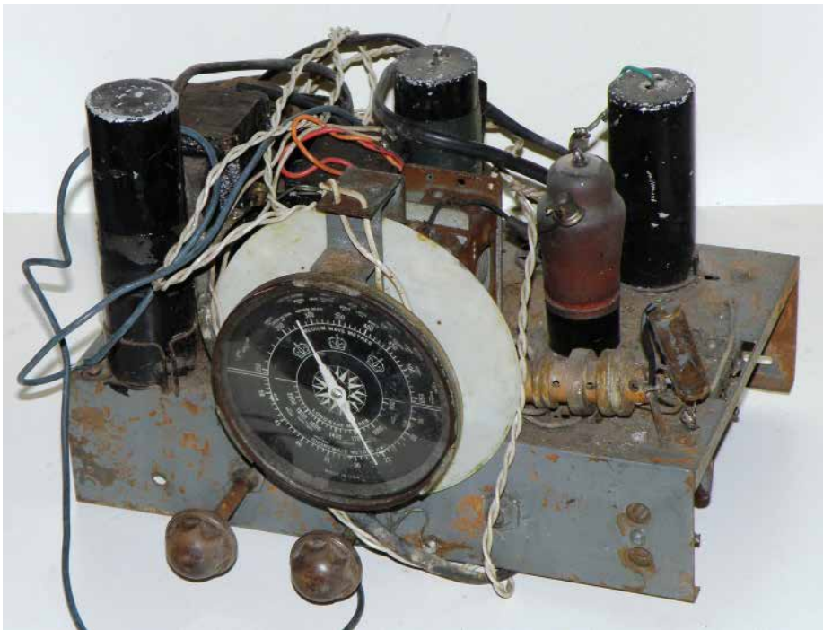
Figure 5: The state of the chassis as it reached me, fitted with its two remaining original wooden knobs.
