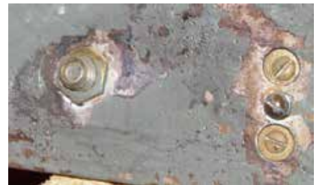
Figure 6: The sheared-off shaft of the wavechange switch.
