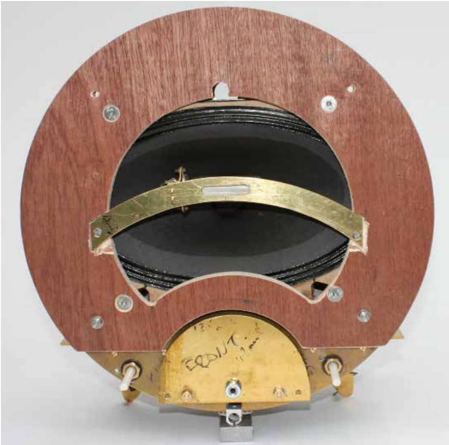
Photo 10 - Magic eye and dial & control mountings
