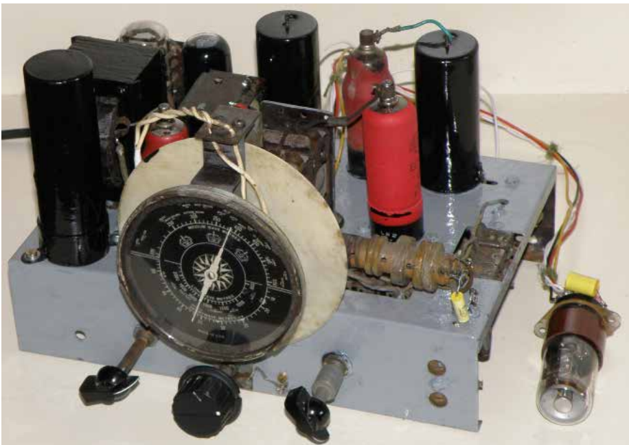
Figure 12: The restored state of the chassis, with the 6E5GT magic eye alongside, supplied by flying leads, before it was mounted onto its fixing bracket.
