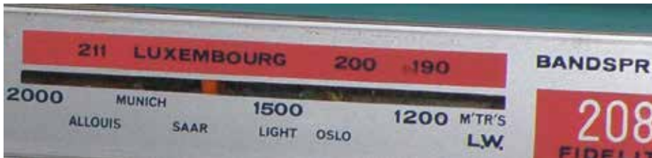
Figure 5: My Fidelity 208 Bandspread transistor radio's long wave dial, from 1965. I believe that the station marked Saar is the same as Deutch Sender marked on the Emerson CULW274's dial. The prominent Luxembourg marking is indicating the position on the bandspread dial of the station's medium wave 208m transmitter.
