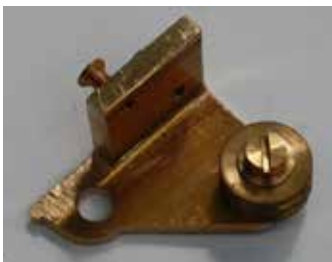
Photo 14 - RH dial string pulley
