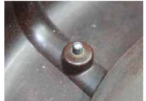
Photo 4 - Grub screw in-situ
