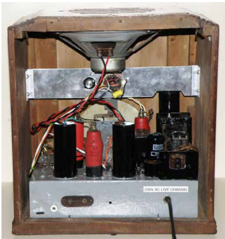
Figure 13: Rear view of the radio with the chassis back in the cabinet. The upward facing speaker and the magic eye mounting bracket can be seen.
