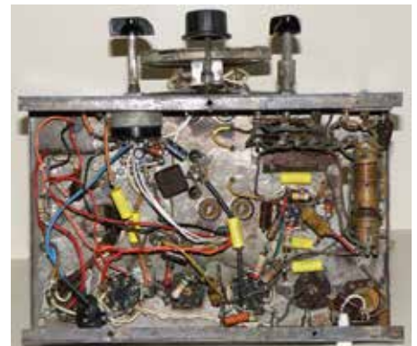
Figure 9: Bottom view of the chassis after restoration. You can see the new shaft on the wavechange switch, fitted with an extension to restore it back to its original length, and the power supply choke has been removed.
