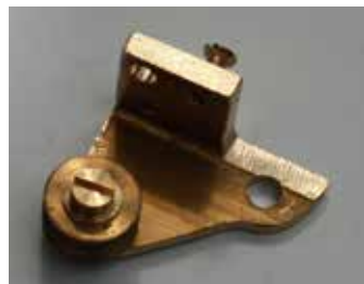
Photo 15 - LH dial string pulley
