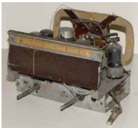
Figure 5: Front view of the chassis. The horizontal ruler scale - calibrated in inches - is used to indicate useful wavelength points when aligning the radio.
