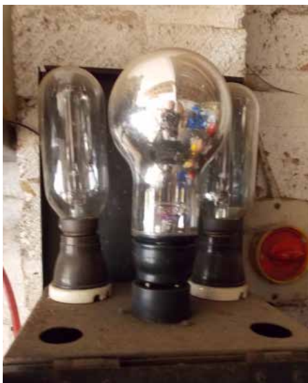
Fig 1 Interior of charger showing low voltage "Tungar" rectifier valve.
