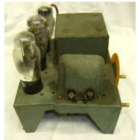
Figure 2 Unrestored chassis showing bent chassis.
