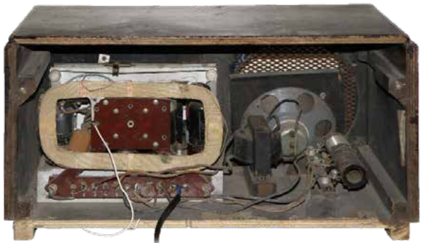
Figure 2: Rear view of the radio, again in 'as received' condition. The 11-way tag strip is stepped away from the chassis by a couple of 1-inch long spacers. The white wire dangling out of the back seems to have been an external aerial connection, but the 'official' connection is to the socket in the middle of the paxolin panel in the frame aerial.
