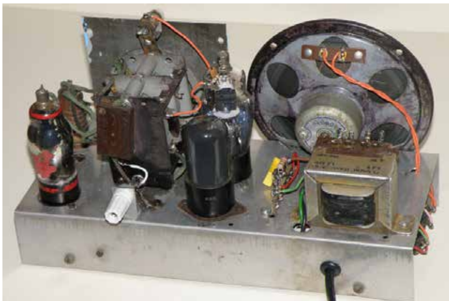
Figure 8: Rear view of the chassis after restoration. I hadn't replaced the screening can around the detector valve at this stage, and it didn't seem to suffer any instability. The new tag strip accommodating the new diode and series resistor, and the class X2 capacitor can be seen next to the new heater transformer. The original EF39, still without most of its red coating, works well enough to be left in the radio.
