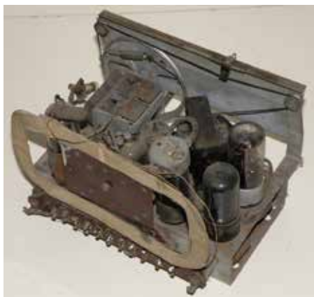
Figure 4: Top rear view of the chassis, showing the large choke at the centre. You should be able to see the small size of the tubular-canned IFTs when compared to the valves, as shown by the one next to the tuning capacitor.
