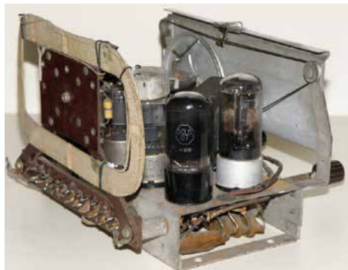
Figure 10: Left hand side of the chassis, showing the frame aerial, and the audio output valve (with a 50L6GT fitted instead of the original 35L6GT) and the original U76 rectifier.
