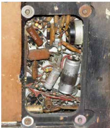
Figure 3: Through the keyhole - bottom view of the radio, with the inspection panel removed, showing the exposed bottom of the chassis in original condition. All the components seem to be original ex-factory. The cut-out also seems to be original, being much neater than I would expect from an amateur. The exposed, and potentially dangerous, chassis fixing screws can also be seen.
