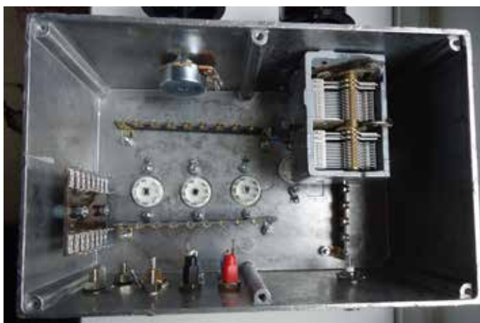
Figure 7: The various controls, sockets and tag strips loosely mounted
