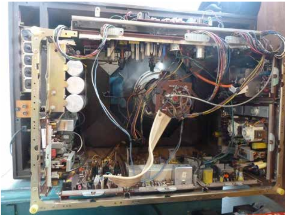
Fig 4: The 2000 showing chassis pulled back for service. The two line output transformers and the EHT transformer are visible on the right. The large mains transformer is concealed in the front of the cabinet on the other side. The largish grey block bottom centre is the PAL delay line. The convergence adjustment panel, inverted at the top, slides out and can be mounted on the top of the cabinet for adjustment from the front.
