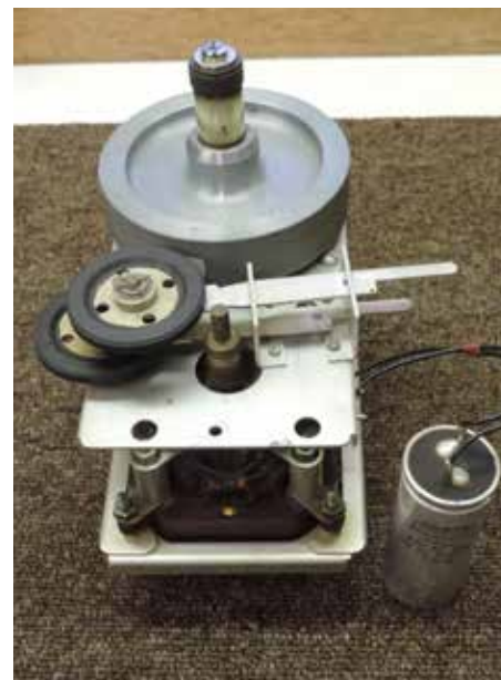
Fig 15 The restored capstan drive sub unit prior to re-assembly onto the main deck showing the relative positions of the idlers, capstan and motor.
