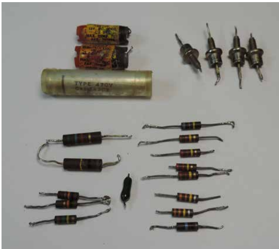
Fig 21 A small number of components were renewed in the Ferrograph mostly resistors associated with the amplifiers. The scorched capacitor (C48) can be seen at the back of the picture.
