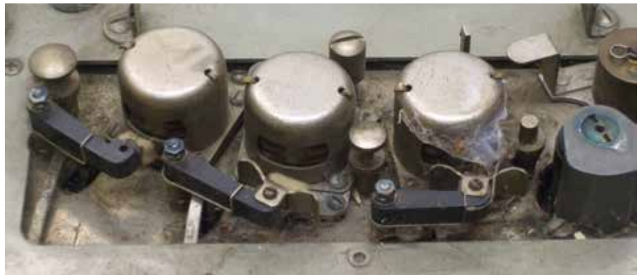
4 A wider view of the general state of the tape path area of the deck and the recently deceased livestock whose home had occupied most of the replay head.
