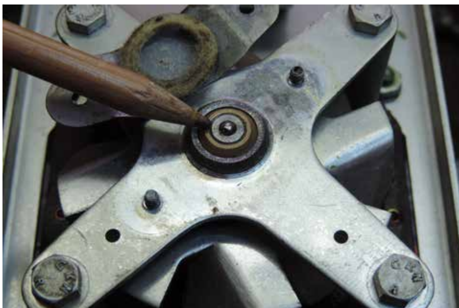
Fig 14 The bottom bearing of the capstan drive motor, this along with the take-up and rewind motors were disassembled, cleaned and re-lubricated
