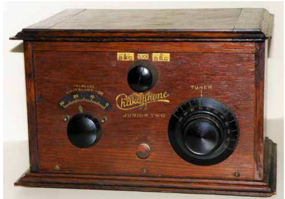
Figure 1: Front view of the radio, showing the excellent condition of the front panel. The lettering is pretty much complete, apart from the worn Pull On and Push Off decals above and below the on-off switch.
