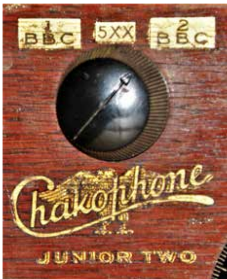
Figure 2: Close-up of the waveband switch and the 'Chakophone' branding on the front panel. Note the eagle behind the Chakophone lettering, presumably referencing the Eagle Engineering Company.
