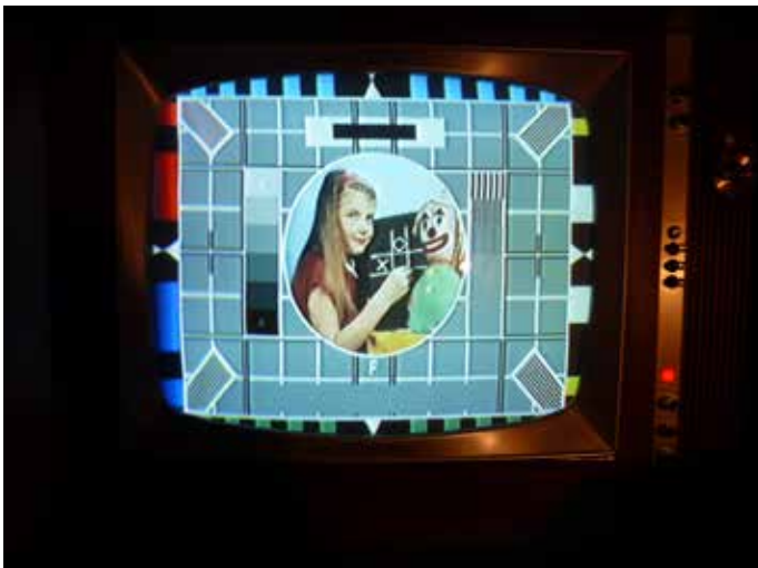
Fig 1: A colour Test Card on a 1967 GEC hybrid . Note the colour patterning in the middle of the frequency bars on the right. This is due to the 4.43 colour sub-carrier falling within the luminance pass-band and is a limitation of the PAL and NTSC systems. The red light on the right comes on to indicate you are receiving a colour picture!
