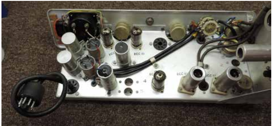
Fig 5 The general view of the front amplifier chassis showing the layout of the valves associated with the recording amplifiers and meter circuit. Note the sticky pool of electrolyte on top of the capacitor towards the lower left of the picture.
