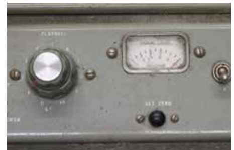
Fig 7 Yuk! What a mess. The screen printing will have to be cleaned very carefully to avoid removing what remains of it.
