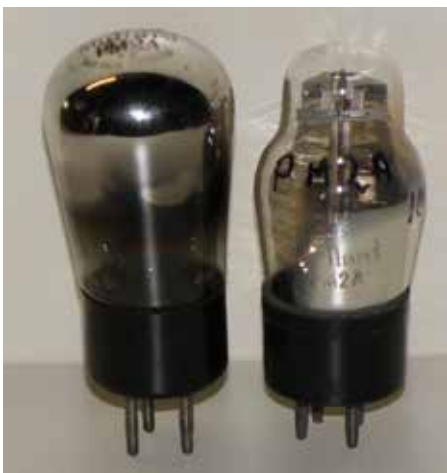
Figure 5: The two shapes of the PM2A as manufactured by Mullard. The left hand valve is the original balloon shape and on the right is the later, 1930s envelope style.
