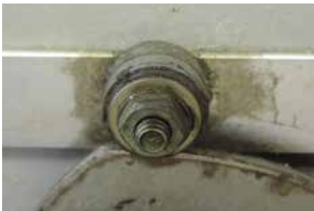
Fig 10 This shows one part of the assembly that needs to be cleaned and re-greased. Wear on this roller guide and the deck function cam can impede smooth operation of the deck
