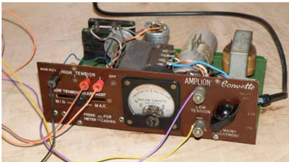
Figure 10: The front panel of the Amplion Convette model M2V mains power supply connected to my radio. The Low Tension Adjustment control adjusts the position of the slider on a 16Ω potentiometer.
