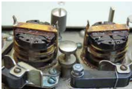
Fig 6 This view of the magnetic heads with their mu-metal shields removed shows just how much further tape oxide and general dirt was found.
