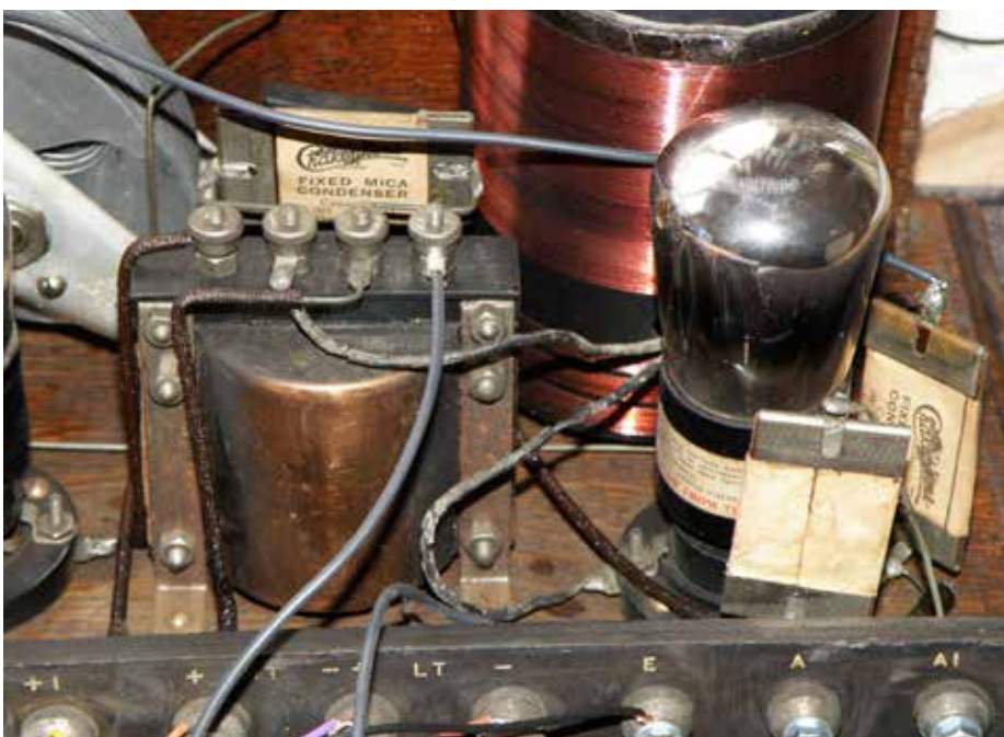
Figure 7: The audio coupling transformer, and the three mica capacitors - all with Chakophone branding and presumably produced locally at the Warwick location – and the PM1HF detector valve.
