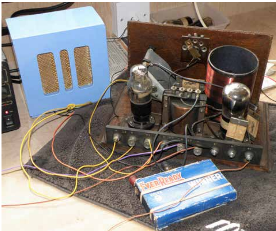
Figure 8: Rear view of the chassis, alongside my distinctly non-period loudspeaker. The connections to the Ever Ready Winner grid bias battery and the other power wiring can be seen.
