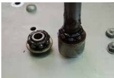
Fig 8 Treacle anyone? This is how the bearing races were found once the capstan had been completely disassembled.
