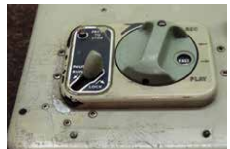
Fig 9 This view of the control knob area fitted on a later series of deck shows quite clearly the wear and tear generally inflicted upon it and the things to look for.
