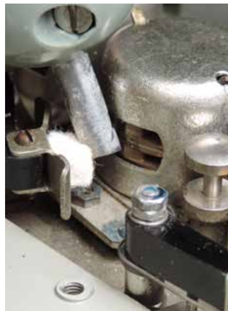
Fig 19 Demagnetising the record and replay heads along with the tape guides is an essential part of the maintenance regime.
