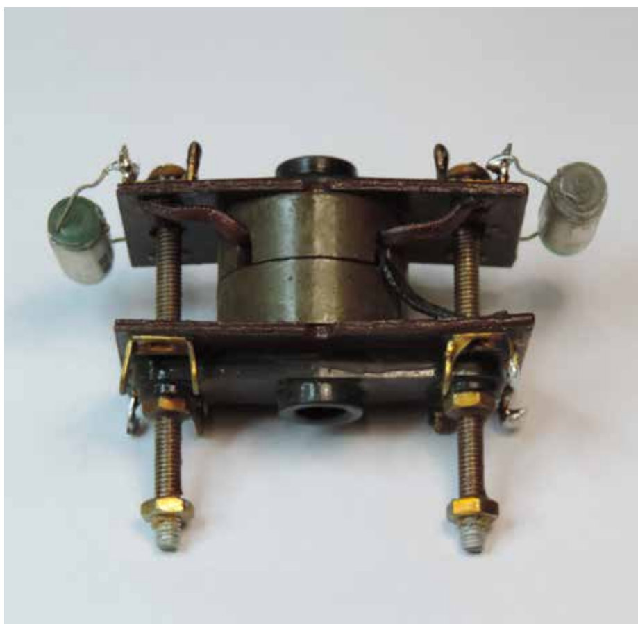
Fig 17 The defective bias/erase oscillator coil referred to in the text. It is very unusual for this component to fail in these machines; in fact almost unheard of.
