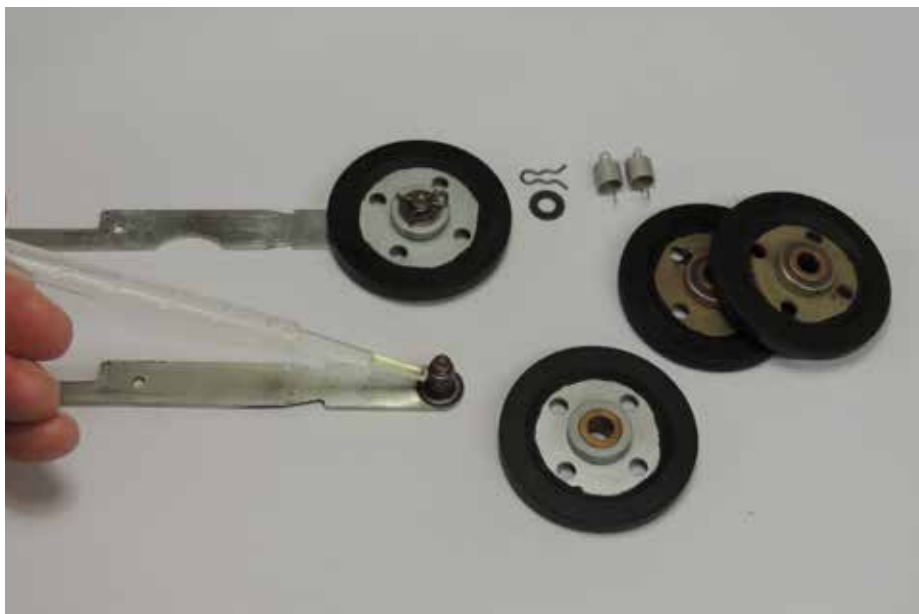
Fig 13 The two idler carriers ready for reassembly with new idler wheels also receiving a single drop of oil prior to reassembly.
