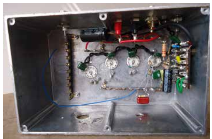
Figure 8: Discriminator tag strip in place and valve heaters wired up
