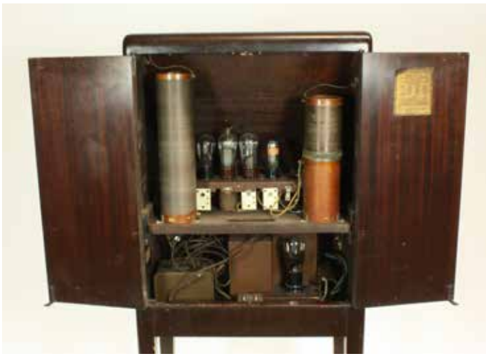
RF chassis (above) and power chassis (below) with 240 to 110V transformer on left.
