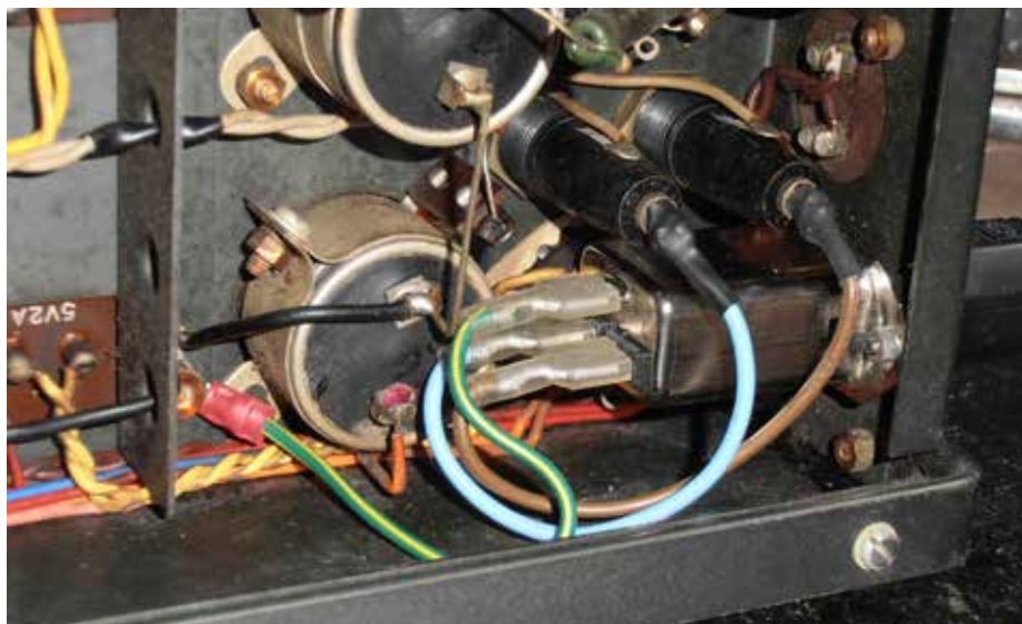
Figure 13: New mains connector / filter. A bit of a squeeze but it's in!
