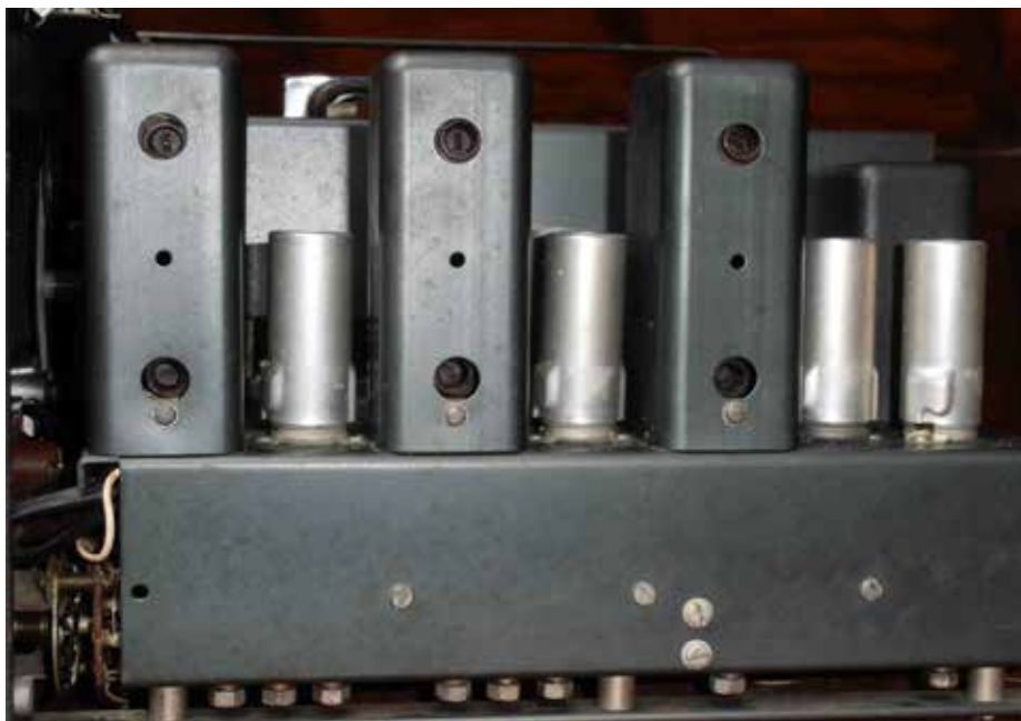
Figure 14: IF adjustment cores. Lower cores only accessible at 'Narrow' selectivity setting.
