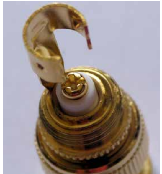
Pic.9. Inner wire screw fixing
