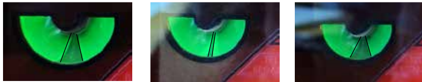
No 1t feedback wdgs. Pantry Xmitter MW With 1t feedback wdgs. Pantry Xmitter MW 2m of coax from Amp With 1t feedback wdgs. Pantry Xmitter MW 30m of coax from Amp
