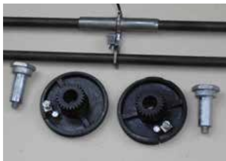
Figure 10: Pulleys and cursor fitted with soldered in terminal block inserts.
