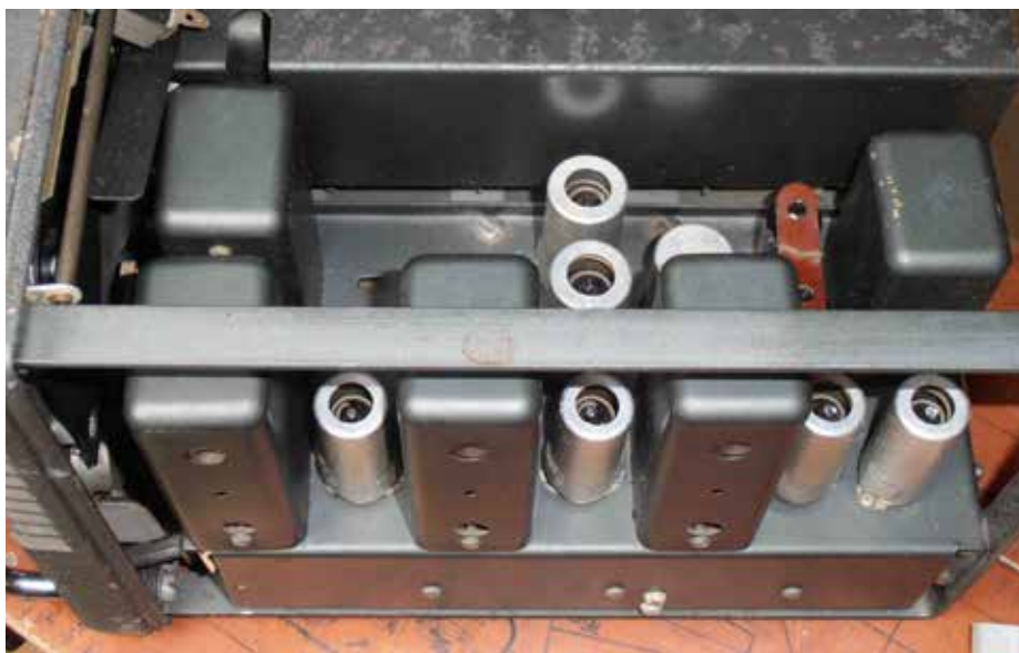
Figure 6: Right hand IF / output stage chassis.
