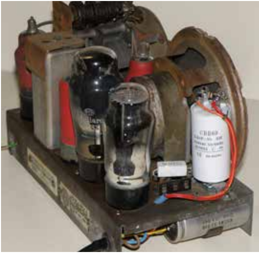
Figure 8: Top view of the chassis after restoration. The white cylindrical object is the 2.5µF motor capacitor, now acting as the heater voltage dropper.
