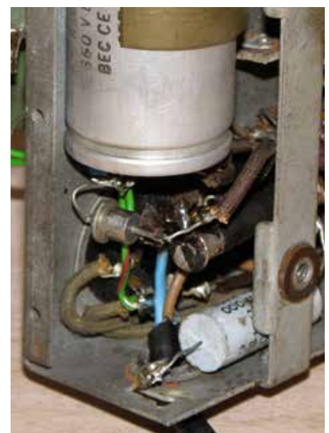
Figure 5: Close up of the power supply area of the chassis, showing the silicon power diode.
