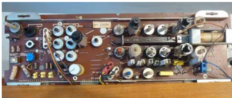
Fig. 3, The convergence board in the service position. The system switch can be seen on the right.
