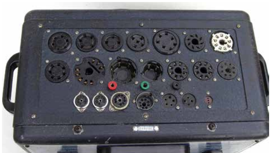
Valve socket deck
