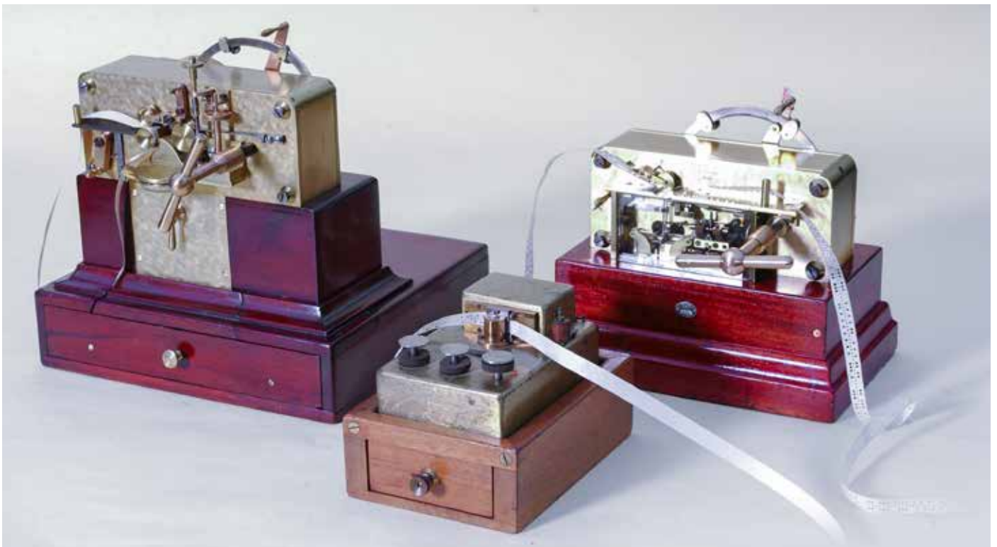
Fig 7 High speed telegraph ensemble, from right to left Tx, Rx and Puncher - photo coll. of the author
