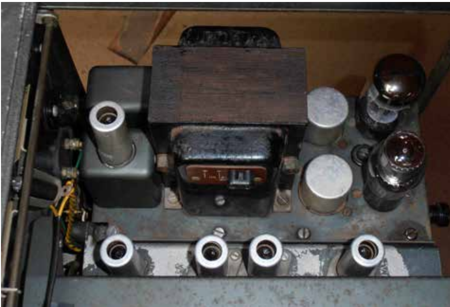
Figure 4: Left hand PSU and BFO chassis.
