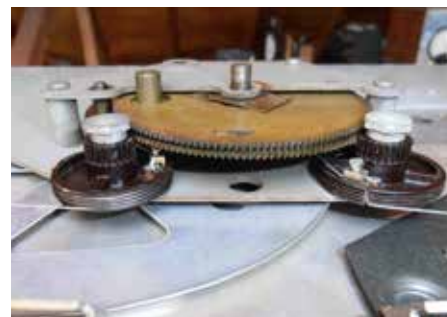
Figure 11: New wire on the two pulleys, left hand full, right hand almost empty apart from about 1/4".
