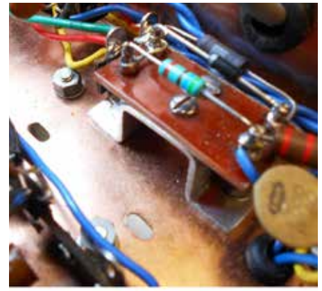
Pic 9 Tag-board & bracket with new silicon rectifier
