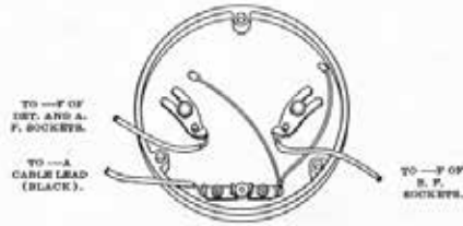
FIG. 54. REAR VIEW OF DOUBLE RHEOSTAT AND FILAMENT SWITCH ASSEMBLY USED IN MODEL 20 (No. 4619-7570), 19 AND 21.
