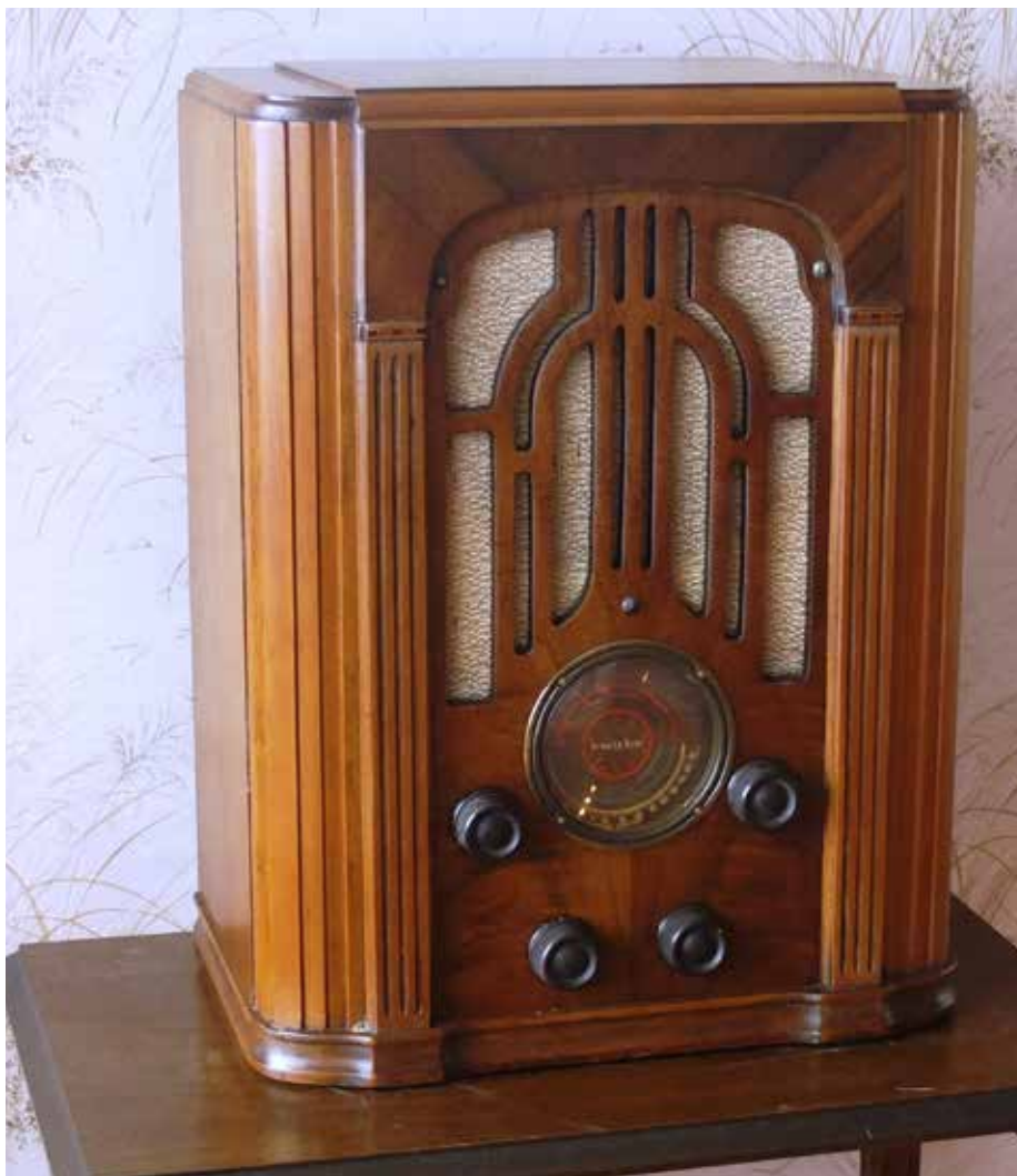
Figure 10 Model 637 type 2 1935-36 - This receiver was one of the current production models at the time of the factory's closing. The cabinet was available in a variety of shadings and used on several related models. A very popular and effective superhet configuration as used by many manufacturers, they had an R.F. and a single I.F. stages covering a couple of shortwave bands as well as the standard broadcast band. Atwater Kent's model 216 now used the increasingly popular 6.3volt series of valves of 6D6, 6A7, 6D6, 75 and 42 with an 80 rectifier. Featured was the new circular style buff coloured Airplane dial, still with the two speed drive. Mid Year, the valves were changed to the new all metal series, with little modification necessary to become the 317/337/617 and 637 type 1 models. For 1936, the 637 type 2 was essentially the 1935 model with a new screen printed black dial, and with illuminated arrows replacing the metal pointer. Zenith had set the fashion for black dials. There is a fuller description of the chassis in the accompanying article.
