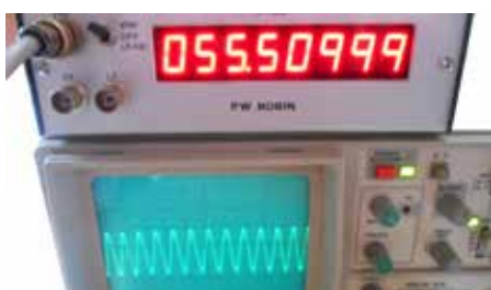
Pic 14 55.5 MHz displayed on 20 MHz Hameg 2037 scope
