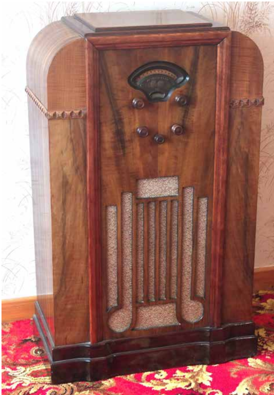
Figure 9 Model 447 1934 - The next season's development of the 1933 model 708, with a new pentagrid converter valve type 2A7 replacing two of the 5B's was the model 447. The tuning capacitor had split stators to spread the upper frequency band. The elaborate dual speed dial drive, reported to be Kent's favourite, changed the scales with band switching. This console cabinet was made in New Zealand, a common practice at the time, to economise on freight charges. Much of the chassis, the dial and the handsome mantel cabinet was the same as that used for the companion model 308 described by Gary Tempest in the Spring 2015 Bulletin.
