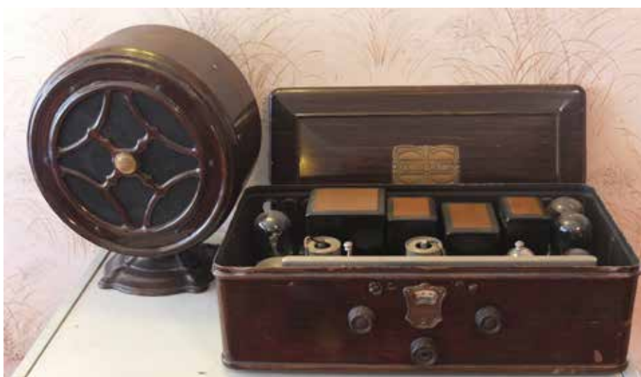
Figure 4 Model 55 1929 - The year 1929 saw the introduction of the new '24 screen grid tetrodes. The 55 has two 224's as R.F. amplifiers, two type '27' as detector and audio stage, a pair of push pull 245 triodes output stage and a type '80 rectifier. The loudspeaker is a 10 inch moving coil unit. By 1930 the 55 had grown to become the 60 and 70 series with massive chassis and three R.F. stages.
