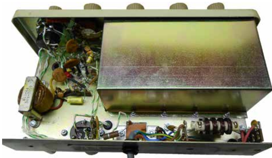
Pic 3 Under chassis screening box
