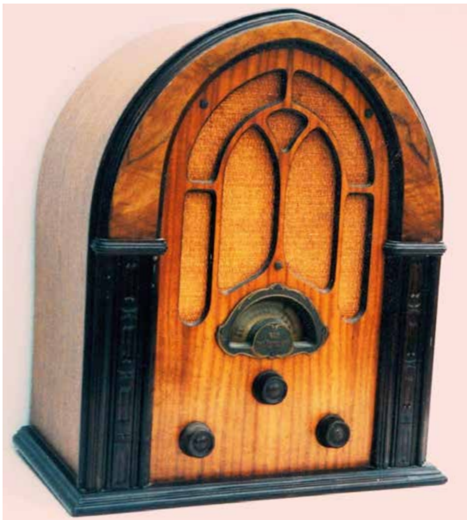
Figure 7 Model 627 Late 1932 - A classic 7 valve "cathedral" using the latest "50" series of valves, with RF stage preceding the mixer. New was the type 55 valve a combined diode detector / AGC/first audio stage. The cabinet is reproduced in the membership badge of the New Zealand Vintage Radio Society.
