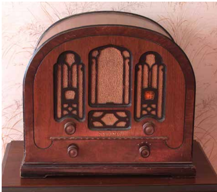
Figure 8 Model 708 1933 - A very compact squat cabinet with 8 valves and covering from 550khz to 20 mHz in 4 switched bands, a fully calibrated dial scale and planetary geared dial drive to a 4 ganged tuning capacitor. This was a very advanced and high performance receiver for the time, with two I.F. Stages tuned to 472.5 kHz to minimise images. It uses five type 58 pentodes, a 2A6 diode/triode and a 2A5 output pentode, all powered by the inevitable 80 rectifier.
