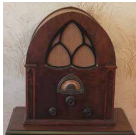
Figure 5 Model 84 type 1 1930/31 - Kent's first "midget" receiver and a first generation superhet. Three '24 valves as mixer, IF amplifier and detector. There was a '27 oscillator, '47 output valve and type '80 rectifier. The second type soon followed, using variable mu '35 valves as mixer and IF amplifier, solving the problem of effective gain control and difficulties coping with strong signals.
