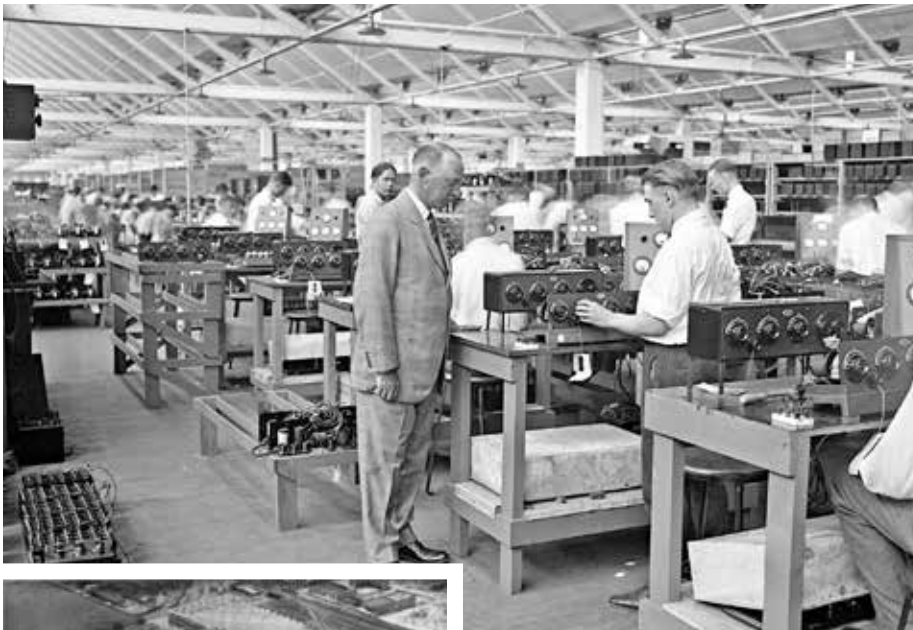
Figure 2 Arthur Atwater Kent observing the testing of a model 20C receiver
