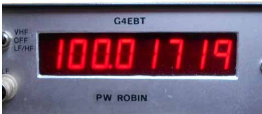
Pic 16 Dial accuracy at 100 MHz
