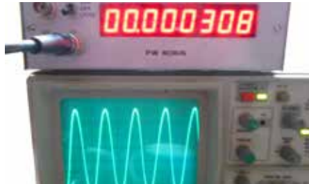
Pic 14 55.5 MHz displayed on 20 MHz Hameg 2037 scope
