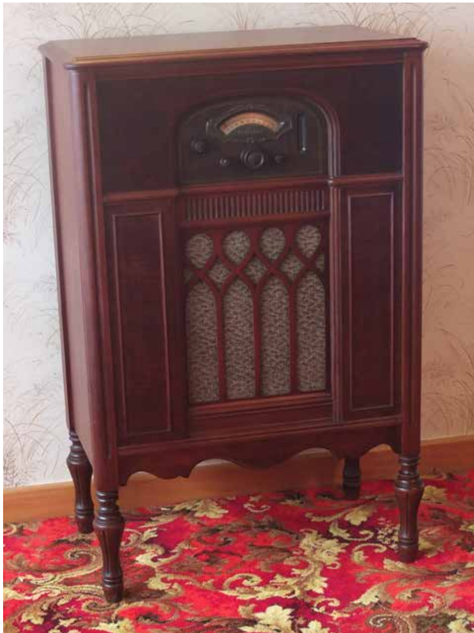
Figure 6 Model 96 Early 1932 - A delux superhet with large (14" wide) chassis, R.F. stage and automatic gain control with pentode output stage. Like many of the larger Atwater Kent sets at this time the dial and controls were mounted on a wood grained painted metal panel so that the chassis could be slid into a variety of cabinets. The cabinet, minus the decorative grill, was first used for the big 1930 model 70 TRF.
