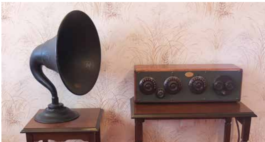
Figure 3 Model 20C 1925/26 - The model 20 was the repackaged popular 5 valve Model 10 Breadboard, dating from about 1923. In 1925 Kent reduced the size of the type 20 cabinet without compromising performance to create the best selling 20C. Over 250,000 were made. There were two separately tuned R.F. amplifiers, a tuned grid leak detector and two audio stages. With it in the photo is an AK type L horn speaker. There is a fuller description in the accompanying article.
