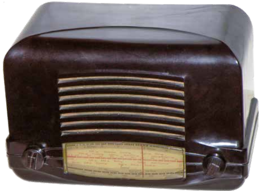
Figure 10: The radio in its restored state, back in its cabinet. You may be able to see that the clear, and yellowed, clear plastic dial barely covers the opening in the cabinet.
