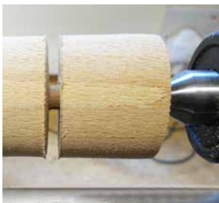
Pic 18: A blank for a small A22 knob being parted on the lathe from a beech spindle.
