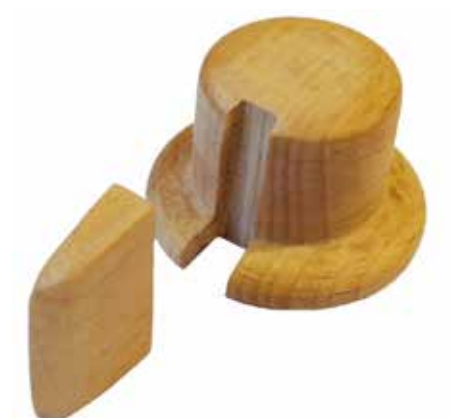
Pic 20 Small A22 knob notched ready for tab to be glued into place
