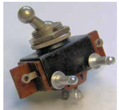
Picture 3. The switch held together with rivets
