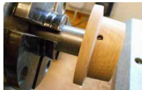
Pic 15: The large A22 knob blank mounted on a mandrel in the chuck, taking shape.
