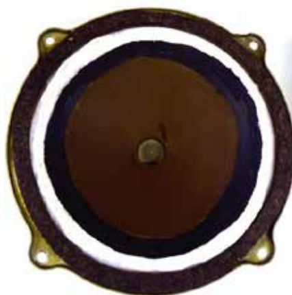
New support for loudspeaker cone
