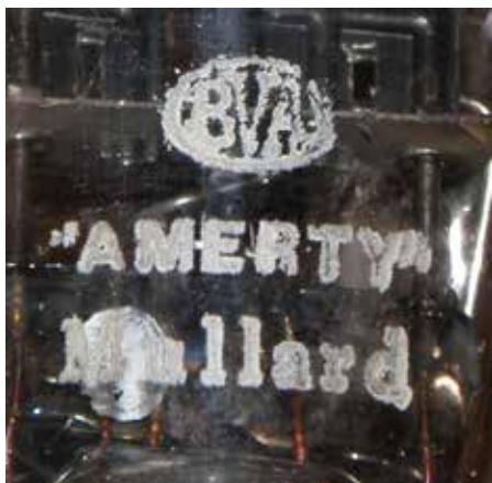
Figure 4: The Mullard 6X5G marked 'AMERTY', indicating that it had been made in the US and shipped to the UK to be sold by Mullard.
