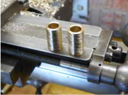
Pic 3: Two brass inserts turned and roughened up.
