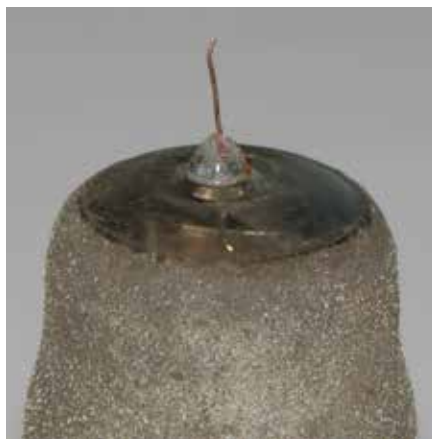
Figure 5: Top of the OM10's envelope showing the broken grid connection wire. Happily the wire was long enough to allow an extension wire to be attached, and the top cap to be re-attached, and the vacuum was still intact as indicated by a working valve when the radio was switched on.
