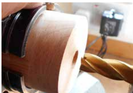
Pic 13: The chuck being rotated by hand, with a 12mm end mill in the tailstock to mill the blank to the correct depth for the brass insert.
