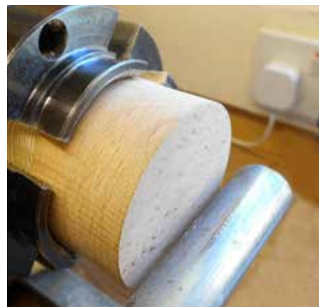
Pic 12: The beech blank in the chuck with a packing piece behind, trued up ready for drilling for the brass insert.
