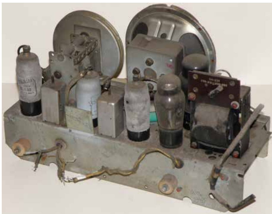
Figure 6: Rear view of the 464AC's chassis, after the frame aerial has been removed. A small screen, mounted between the two IF transformers, can be seen shielding the OM6 IF amplifier valve from the frame aerial. The two 'G' octal valves can be seen adjacent to the mains transformer.
