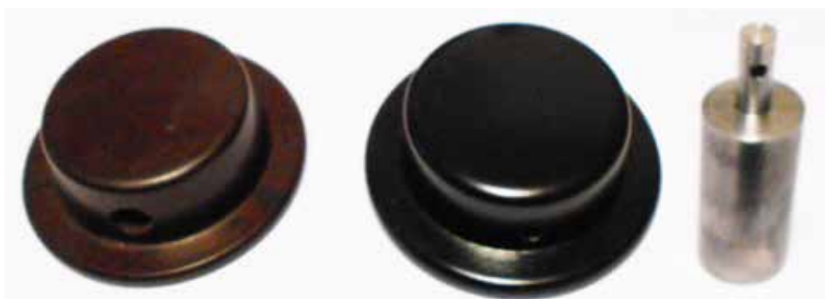
Pic 17: Finished large knob alongside my original brown A22 Bakelite knob, and the mandrel on which the replica knob was turned.
