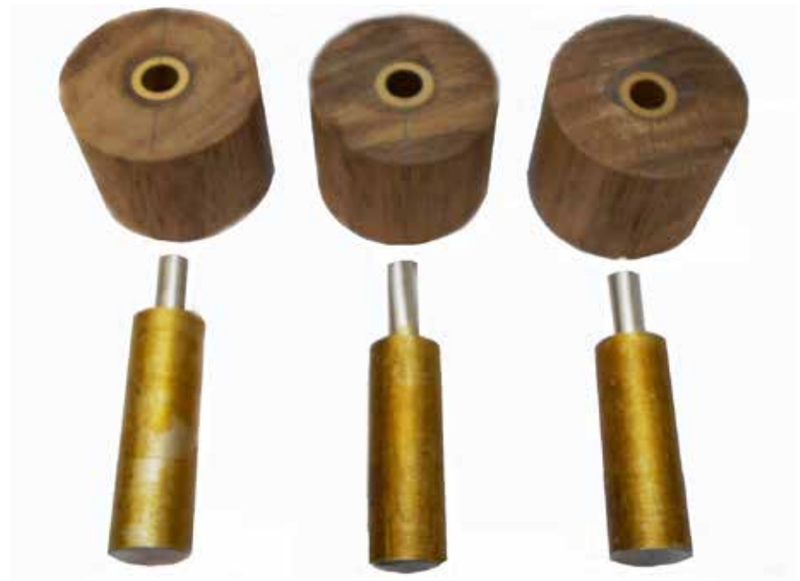
Pic 4: Three walnut blanks with inserts fitted, and three mandrels turned from scrap alloy bar on which to mount the blanks for turning.
