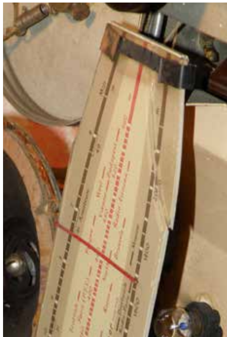
Figure 2: The broken piece of dial glass - sadly the fate of many 464AC dials - is held in place at an angle by the fixing bracket. A portion of the top layer of glass has been lost.
