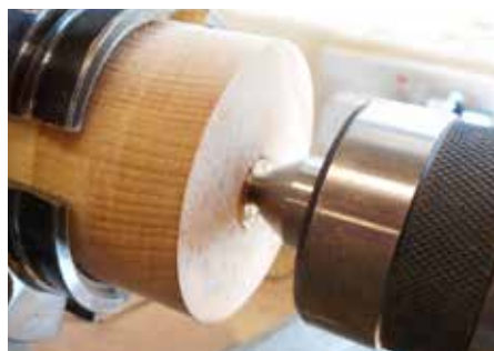
Pic 14: Gluing in the brass insert.
