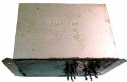
Dubilier Capacitor block
