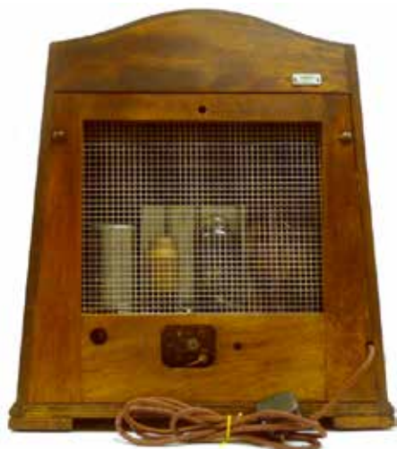
Wire mesh replacement for perished cloth
