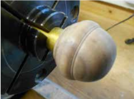
Pic 5: One knob turned and sanded, ready for the perimeter finger grooves to be milled.
