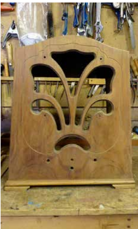
Stripped ready for staining and finishing
